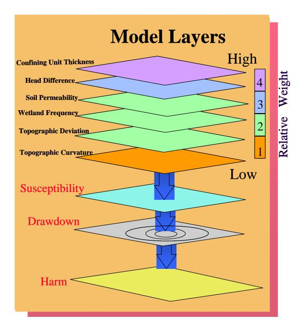
Figure 1. Graphical representation of the GIS model used to estimate the likelihood of harm to lakes from groundwater withdrawal in the St. Johns River Water Management District by the year 2025
