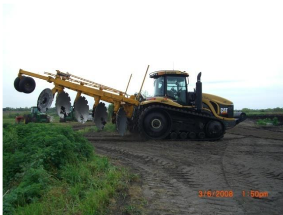
Figure 8. Four-bottom bi-direction plow with 52-inch disks
