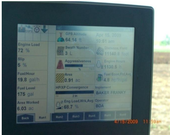
Figure 26. Screen for onboard computer system
