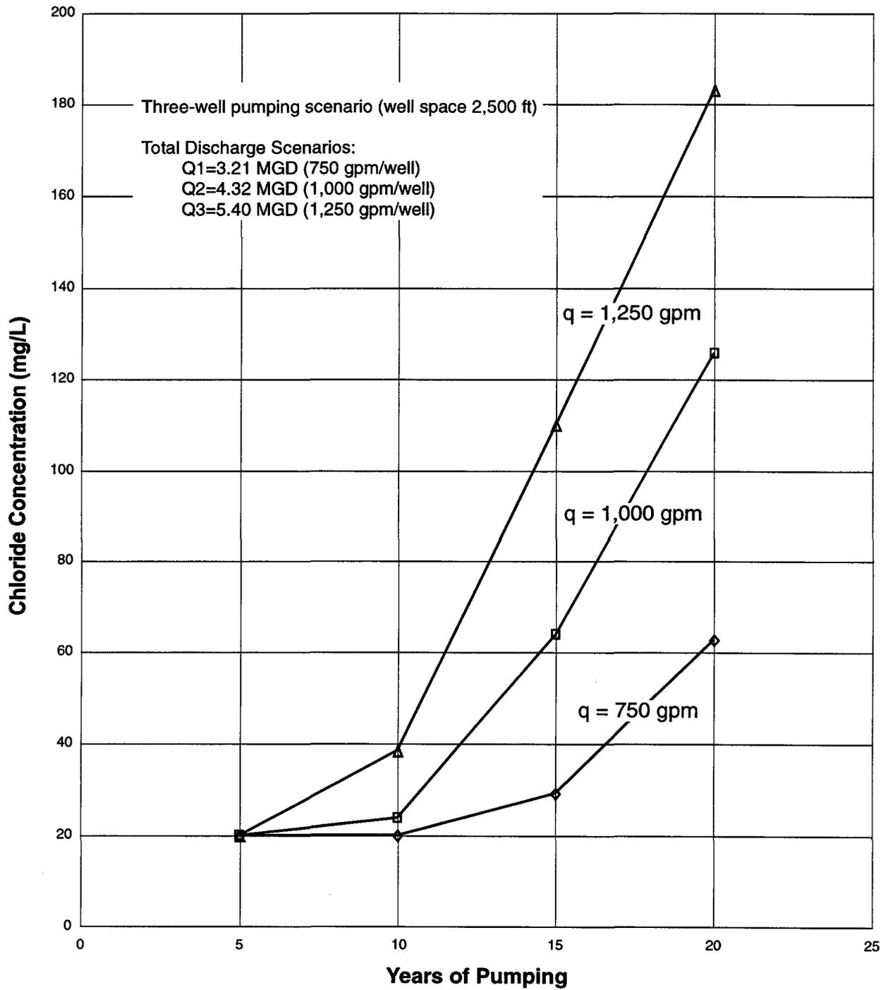
**Figure 34.** Chloride Concentration as a Function of Pumping Duration for the Volusia Site—Three-Well Configuration
