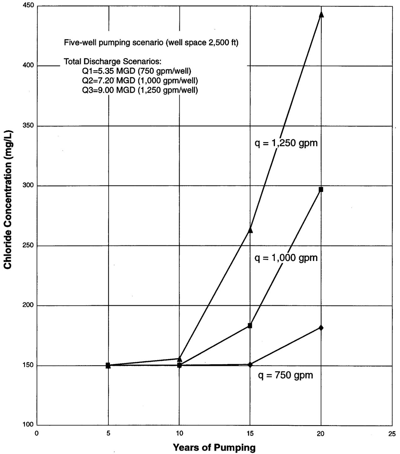
**Figure 30.** Chloride Concentration as a Function of Pumping Duration for the East Orange County Site—Five-Well Configuration
