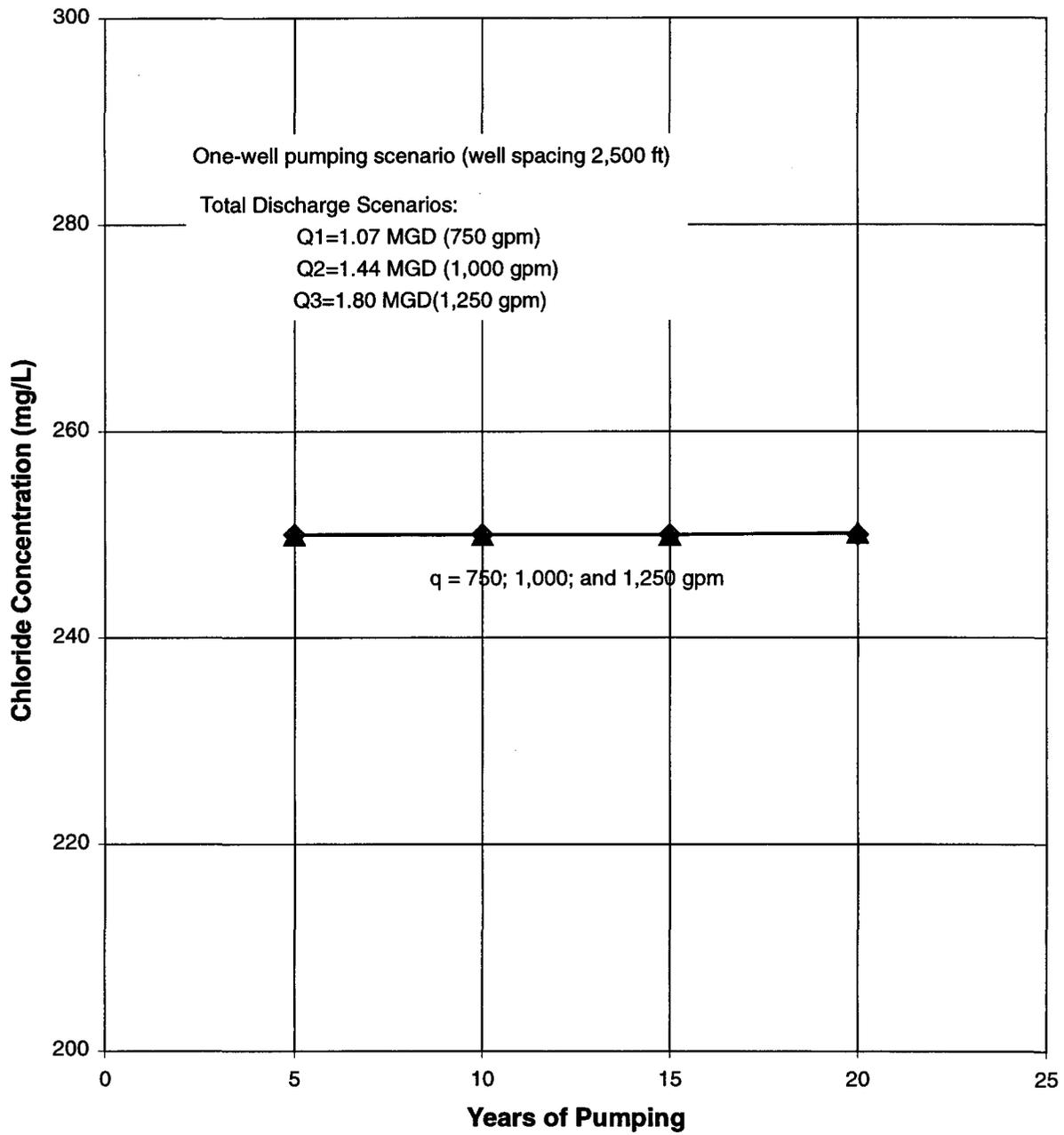
**Figure 23.** Chloride Concentration as a Function of Pumping Duration for the Titusville Site—One-Well Configuration
