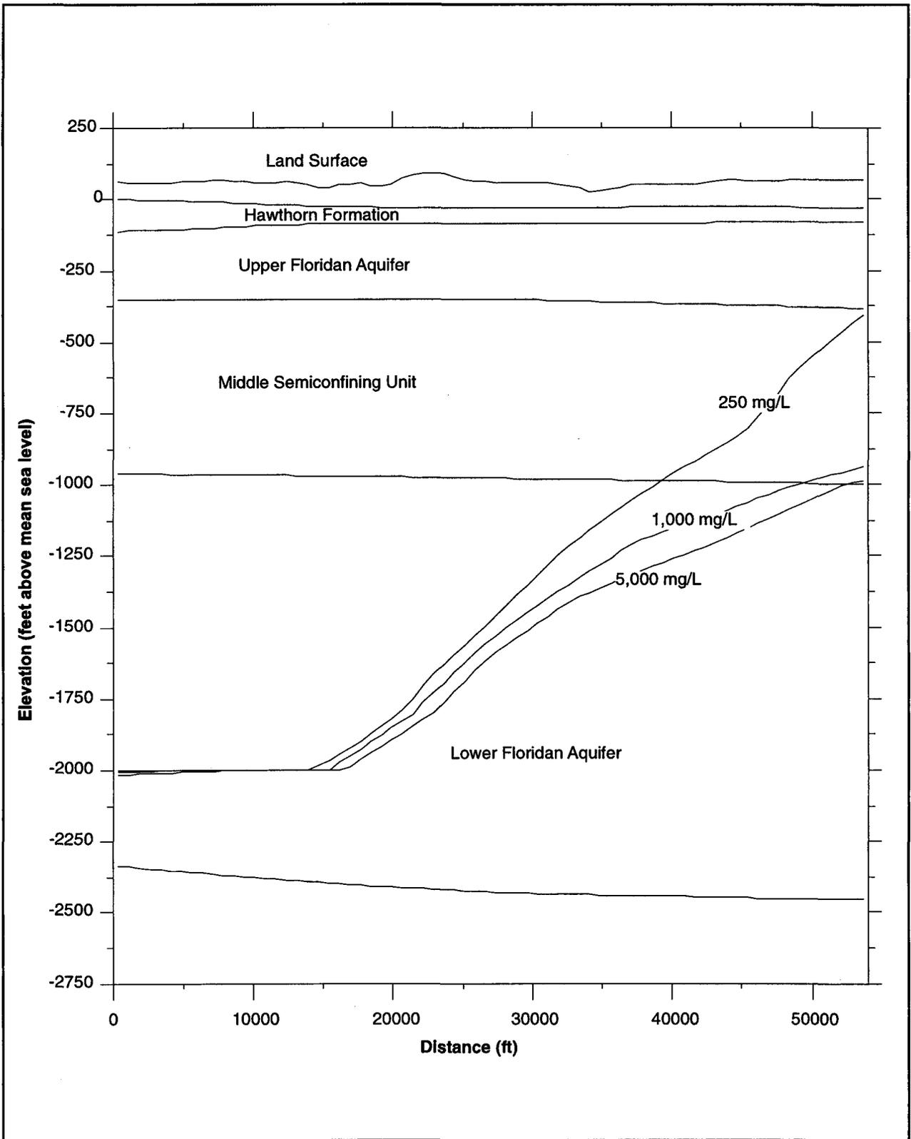
Figure 42. Typical Cross Section at the Lake Jessup Site
