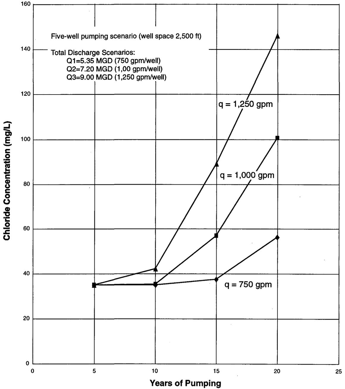
**Figure 48.** Chloride Concentration as a Function of Pumping Duration for the Cocoa Wellfield–Five-Well Configuration
