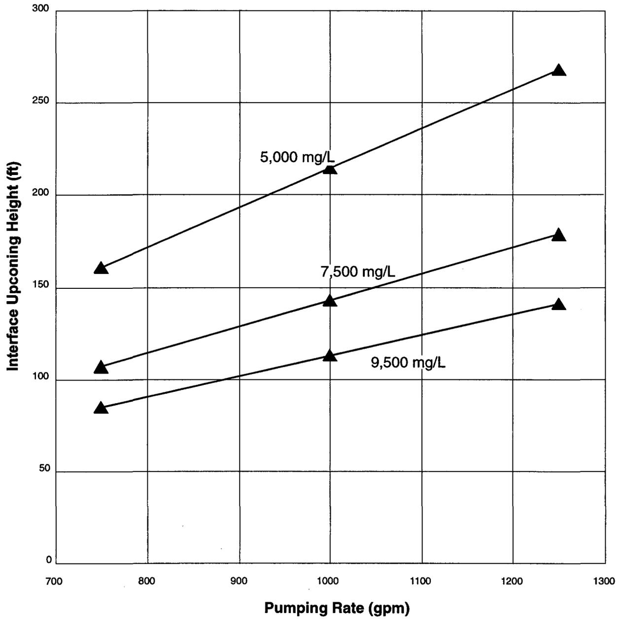
Figure 26. Interface Upconing Height vs. Pumping Rate for the East Orange County Site
