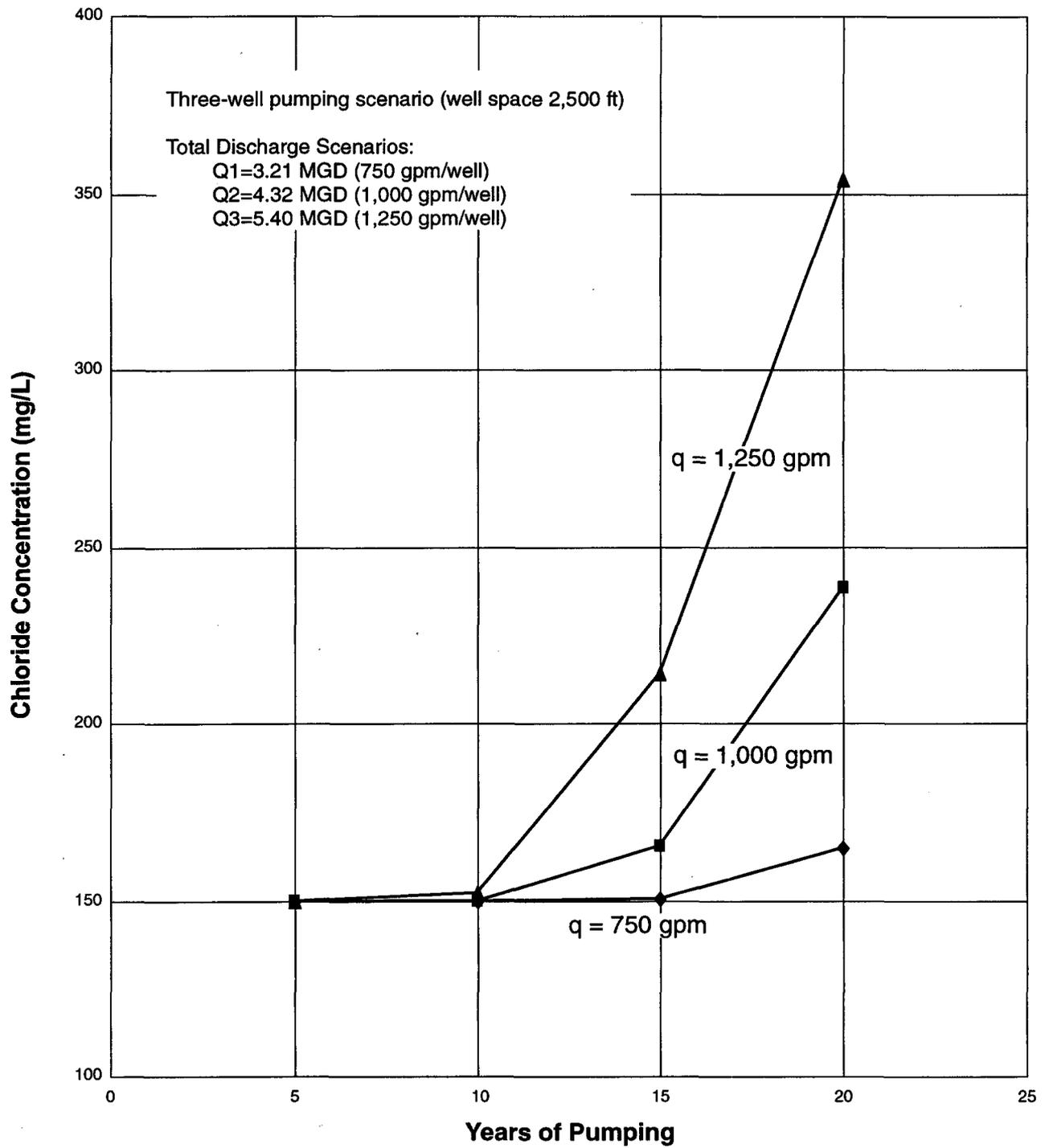
Figure 29. Chloride Concentration as a Function of Pumping Duration for the East Orange County Site—Three-Well Configuration
