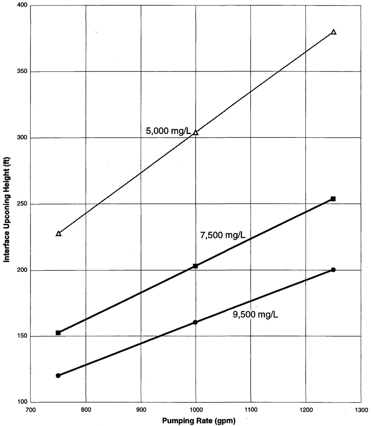
Figure 31. Interface Upconing Height vs. Pumping Rate for the Volusia Site
