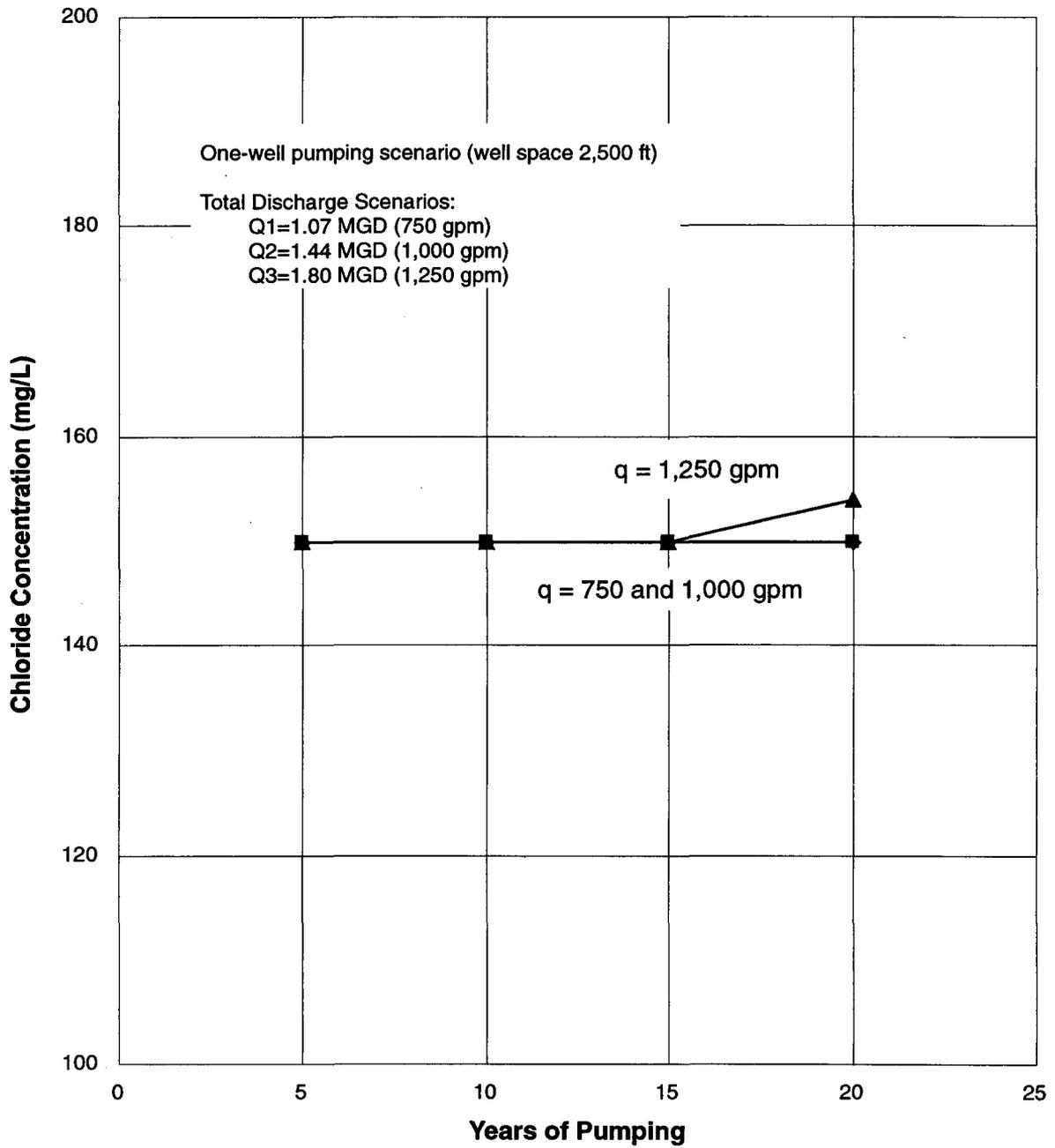
**Figure 38.** Chloride Concentration as a Function of Pumping Duration for the St. Johns County Site—One-Well Configuration
