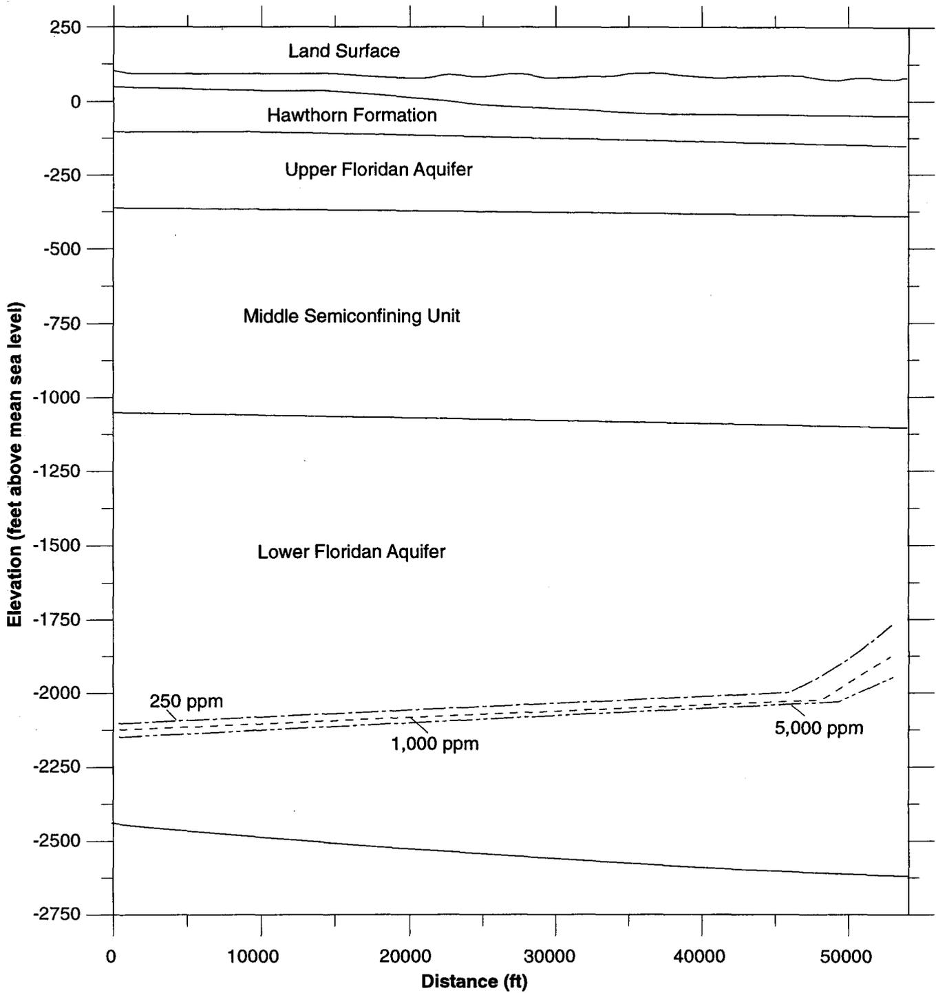
Figure 27. Typical Cross Section for the East Orange County Site
