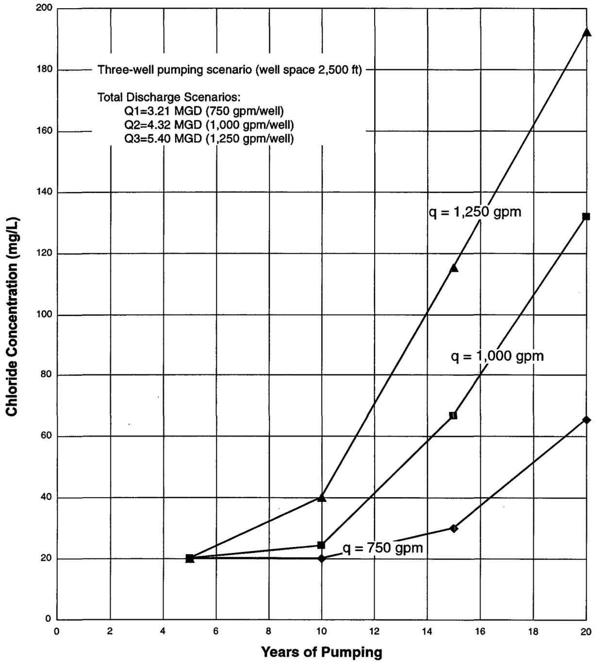
**Figure 44.** Chloride Concentration as a Function of Pumping Duration for the Lake Jessup Site—Three-Well Configuration
