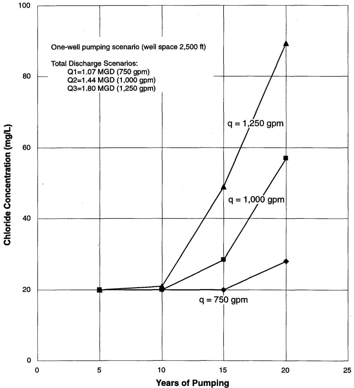
**Figure 43.** Chloride Concentration as a Function of Pumping Duration for the Lake Jessup Site—One-Well Configuration
