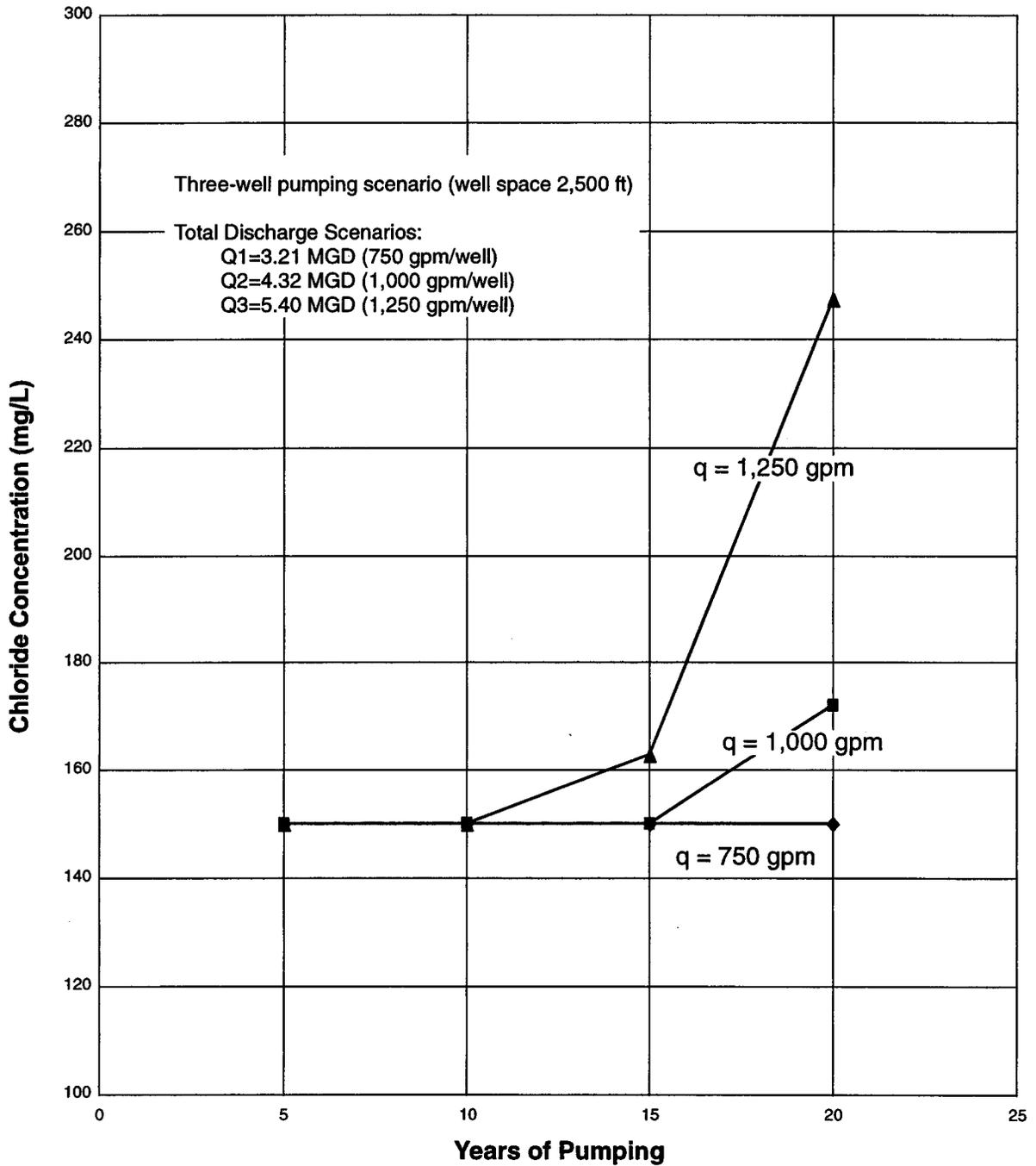
**Figure 39.** Chloride Concentration as a Function of Pumping Duration for the St. Johns County Site—Three-Well Configuration
