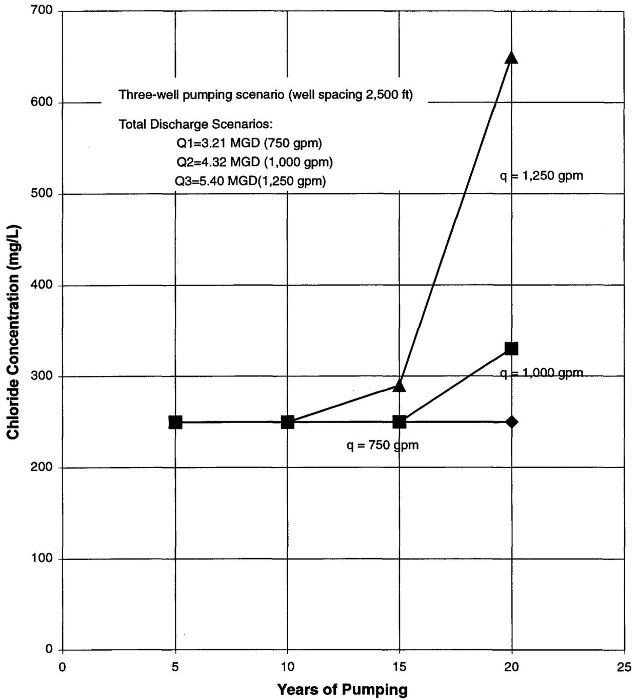
**Figure 24.** Chloride Concentration as a Function of Pumping Duration for the Titusville Site—Three-Well Configuration
