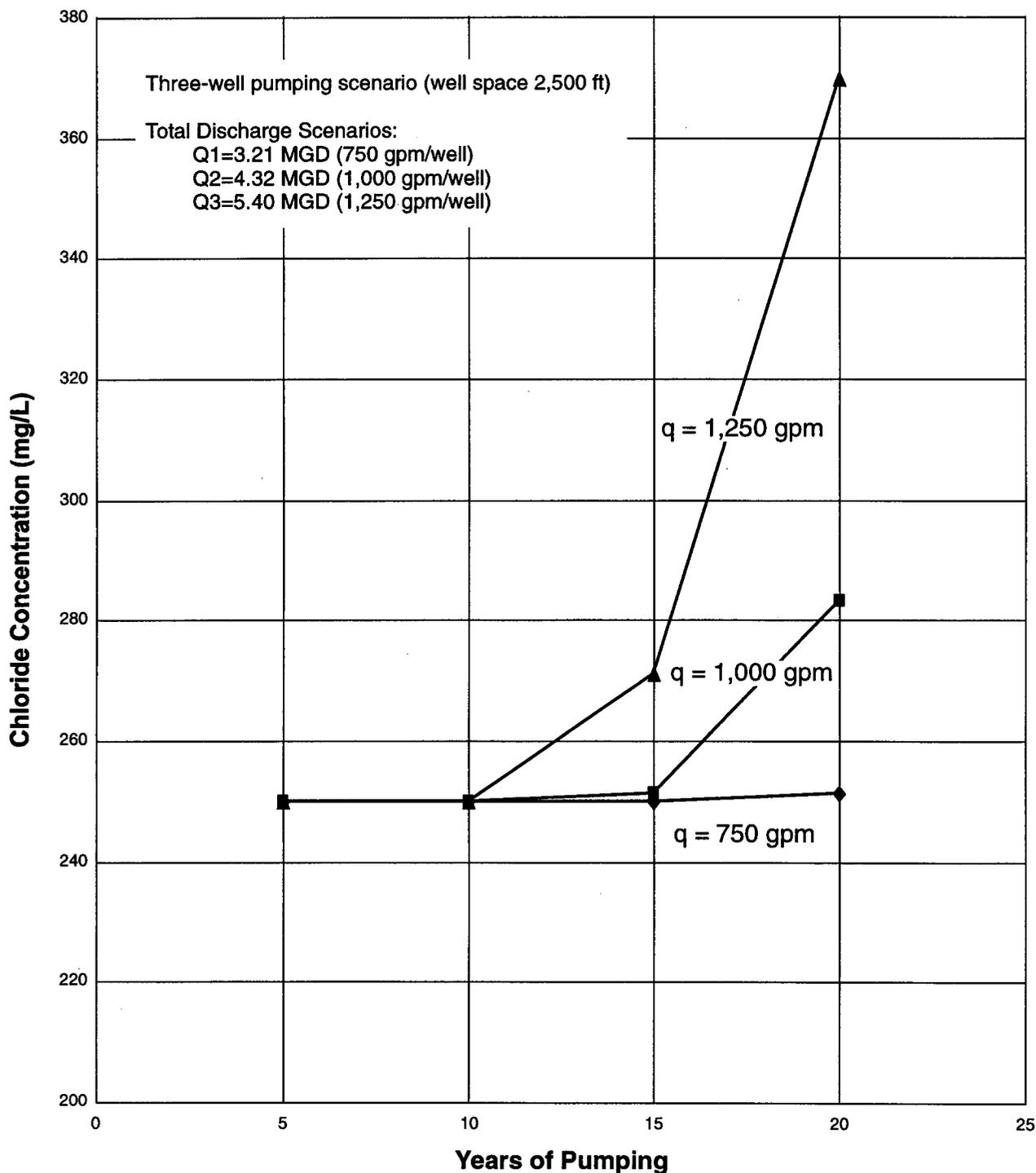
**Figure 19.** Chloride Concentration as a Function of Pumping Duration for the Lake Washington Site—Three-Well Configuration
