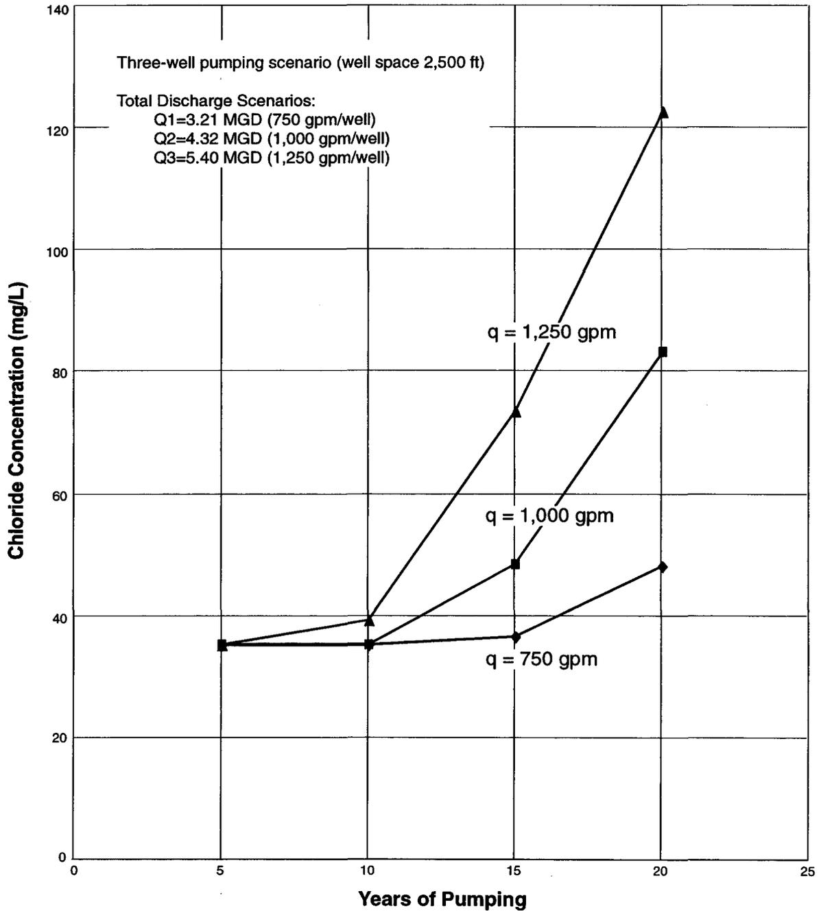
**Figure 47.** Chloride Concentration as a Function of Pumping Duration for the Cocoa Wellfield—Three-Well Configuration
