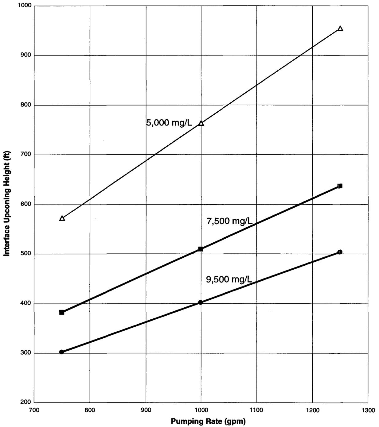
**Figure 41.** Interface Upconing Height vs. Pumping Rate for the Lake Jessup Site
