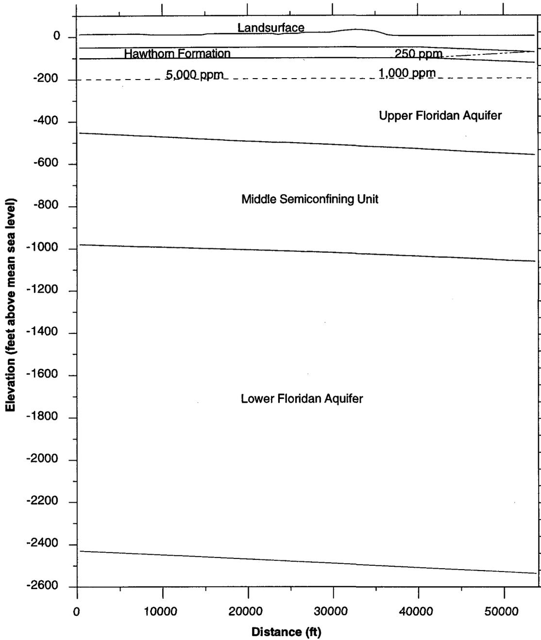
Figure 21. Typical Cross Section at the Titusville Site
