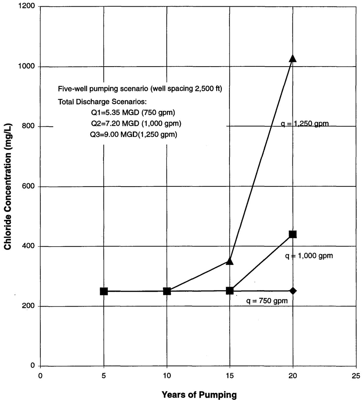
**Figure 25.** Chloride Concentration as a Function of Pumping Duration for the Titusville Site—Five-Well Configuration
