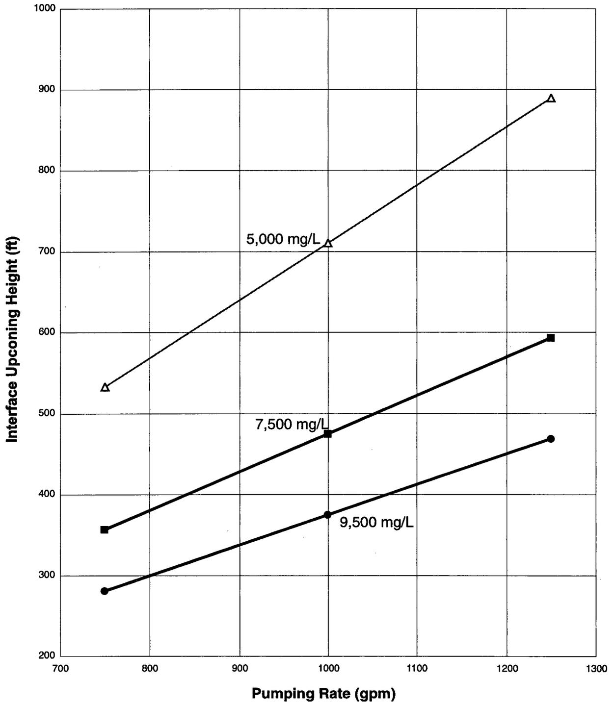
Figure 36. Interface Upconing Height vs. Pumping Rate for the St. Johns County Site
