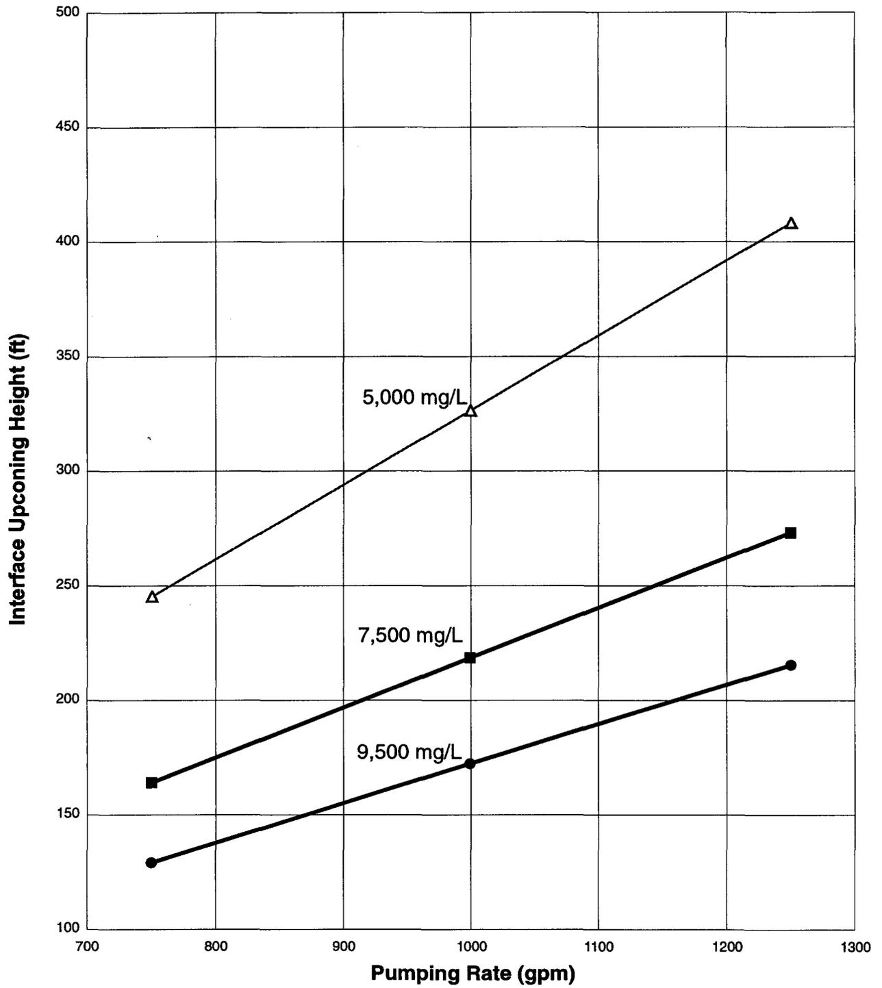
Figure 22. Interface Upconing Height vs. Pumping Rate for the Titusville Site
