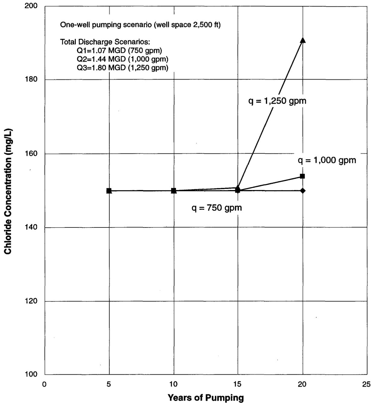
**Figure 28.** Chloride Concentration as a Function of Pumping Duration for the East Orange County Site—One-Well Configuration
