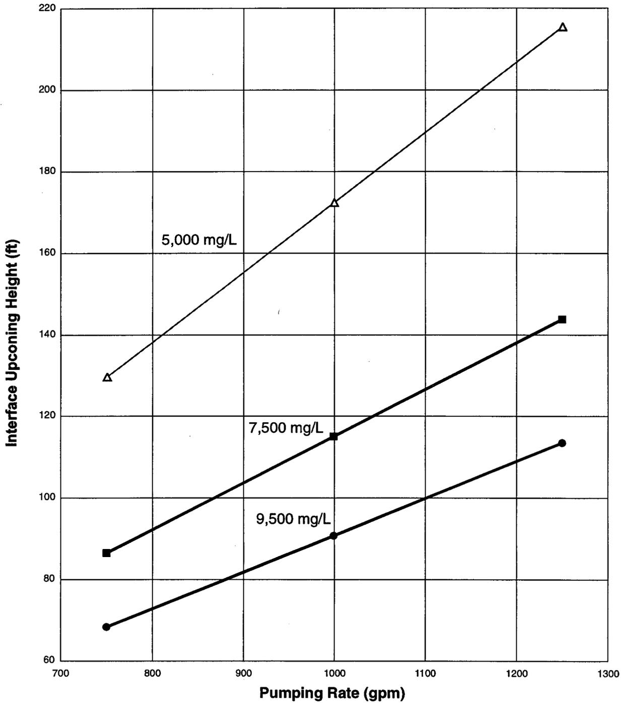
**Figure 17.** Interface Upconing Height vs. Pumping Rate for the Lake Washington Site
