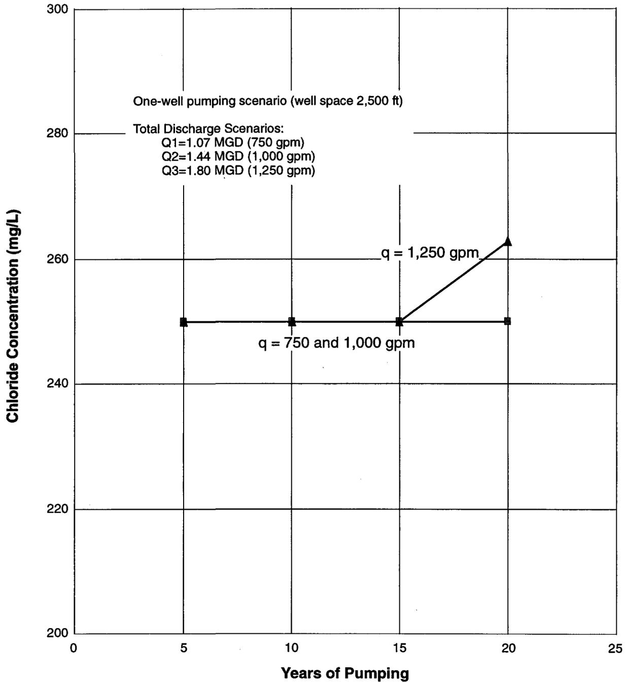
**Figure 18.** Chloride Concentration as a Function of Pumping Duration for the Lake Washington Site—One-Well Configuration
