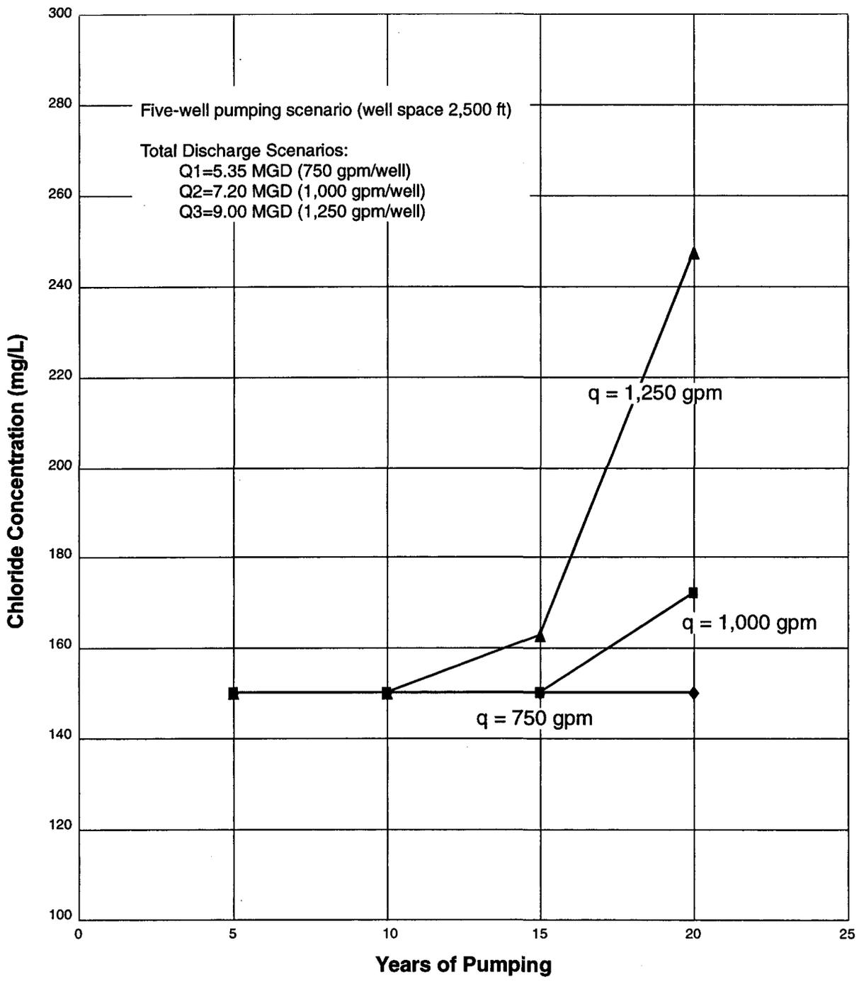
**Figure 40.** Chloride Concentration as a Function of Pumping Duration for the St. Johns County Site—Five-Well Configuration
