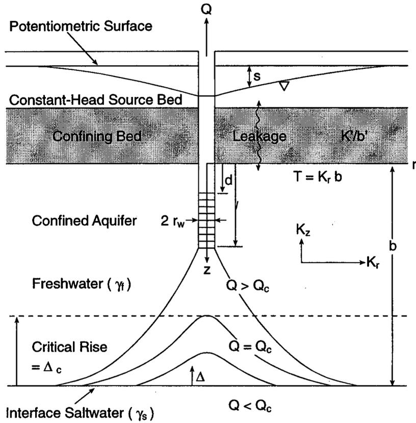
Figure 13. Saltwater Upconing Due to Pumping from a Well in a Leaky Confined Aquifer
