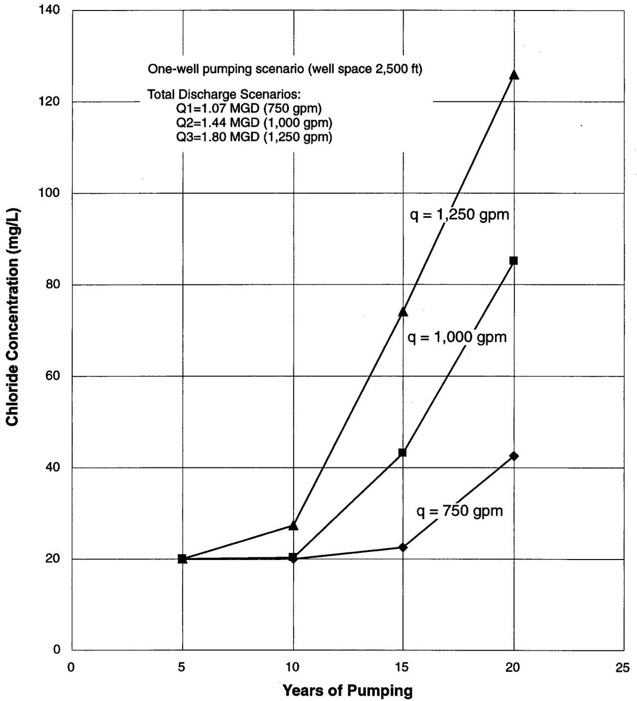
**Figure 33.** Chloride Concentration as a Function of Pumping Duration for the Volusia Site—One-Well Configuration
