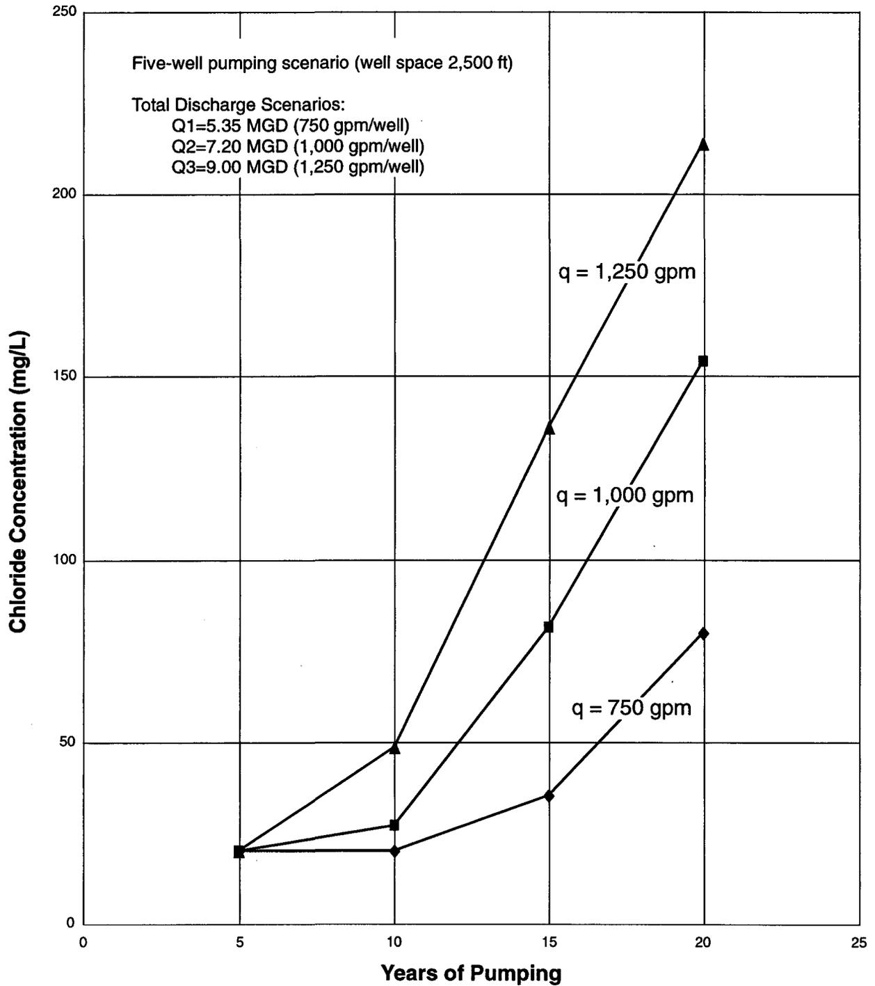
**Figure 35.** Chloride Concentration as a Function of Pumping Duration for the Volusia Site—Five-Well Configuration
