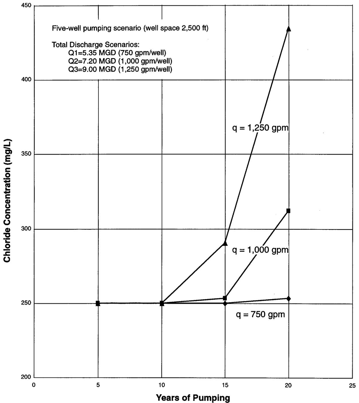
**Figure 20.** Chloride Concentration as a Function of Pumping Duration for the Lake Washington Site—Five-Well Configuration
