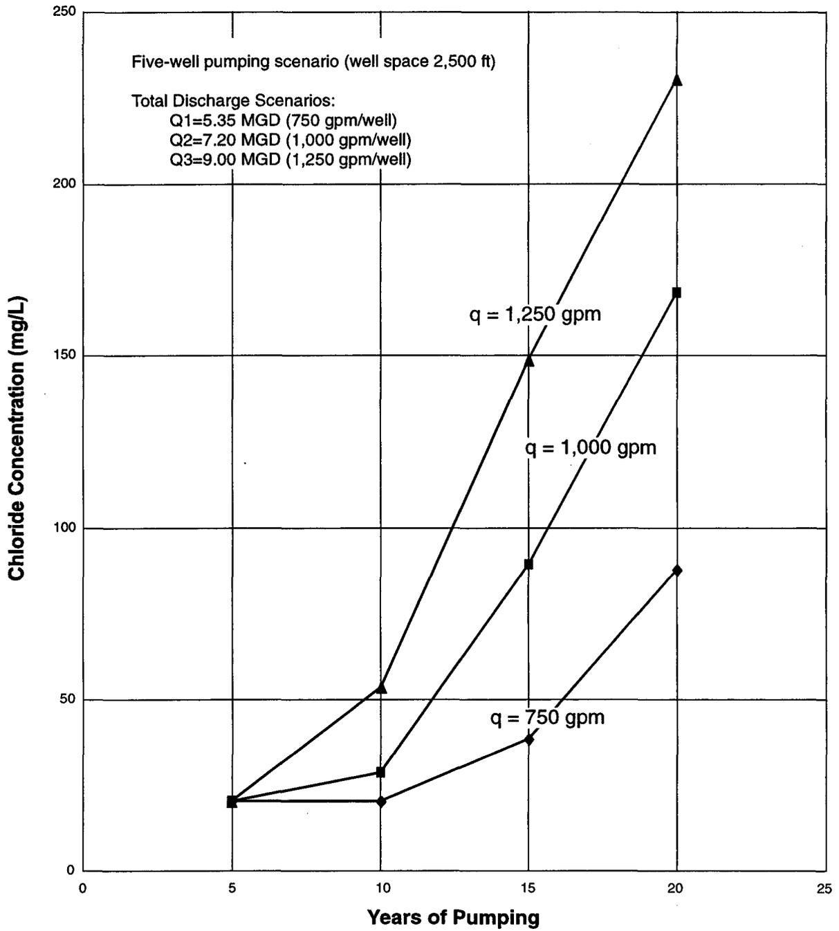
**Figure 45.** Chloride Concentration as a Function of Pumping Duration for the Lake Jessup Site—Five-Well Configuration
