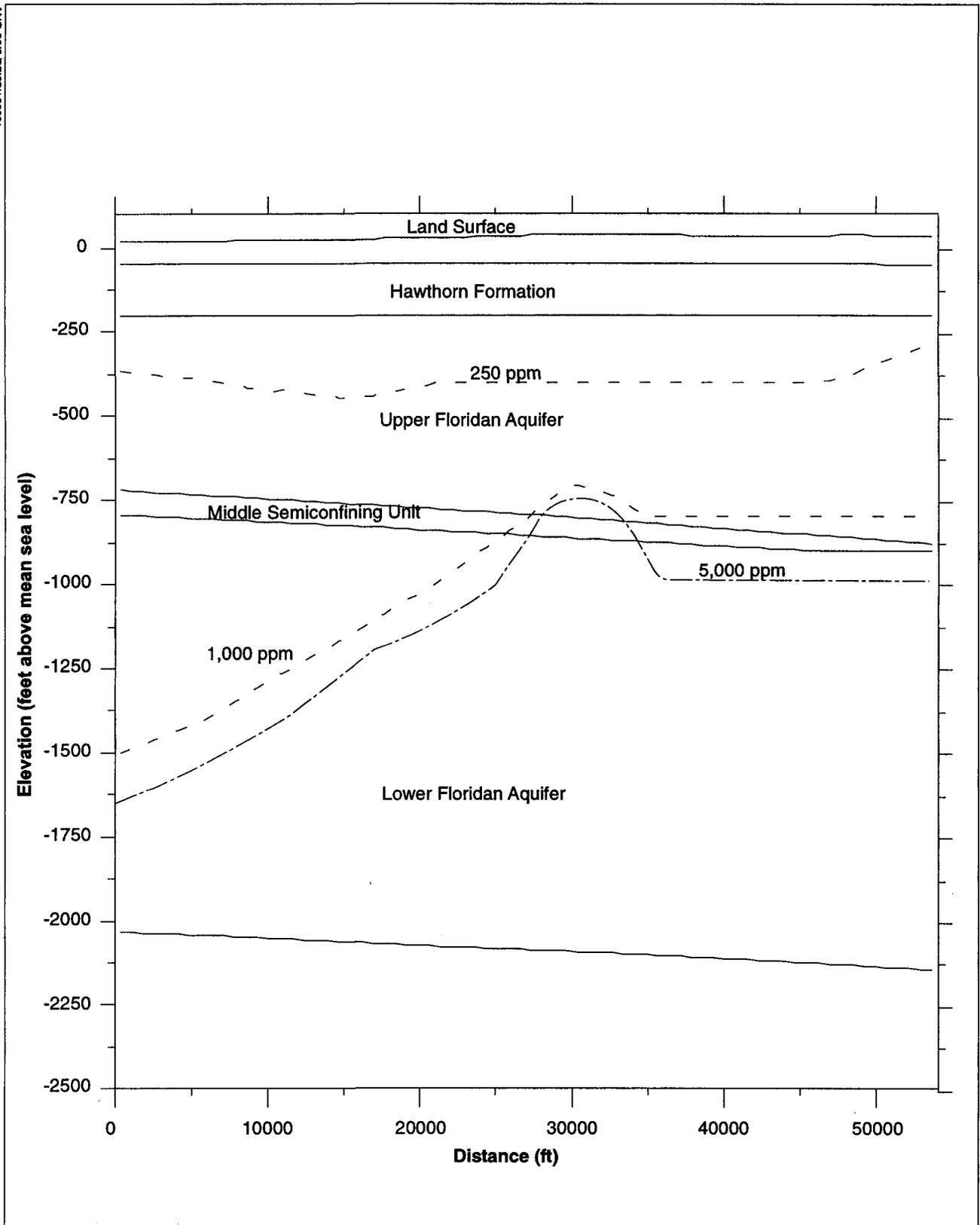
Figure 37. Typical Cross Section at the St. Johns County Site
