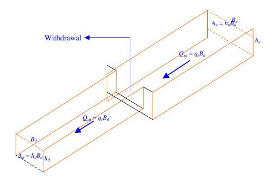
Figure F.3 Flow area and total load reduction due to water withdrawal.
