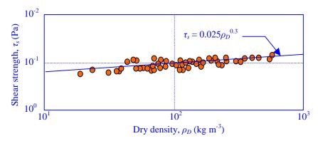
Fig. D.7 Shear strength variation with bed dry density.
