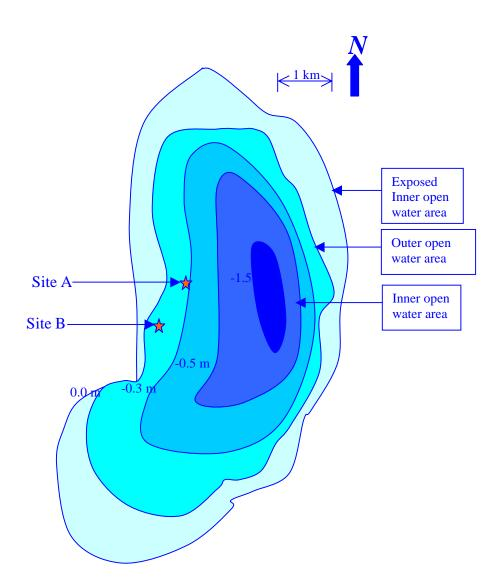
Fig. D.11 Newnans Lake zones based on bathymetry. Suspended sediment concentration was measured at Sites A and B.
