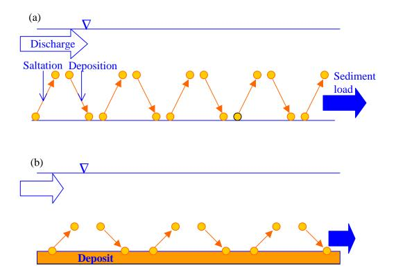
Figure F.1. Live-bed equilibrium in a channel: (a) Given discharge, and (b) deposition under reduced discharge.
