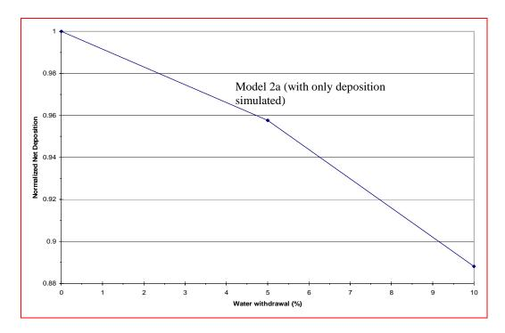
Figure C.14 Normalized net deposition downstream of the water withdrawal site as a function of percentage of water withdrawal for Model 2a.
