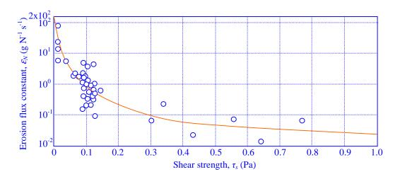
Fig. D.6 Variation of erosion flux constant with shear strength.
