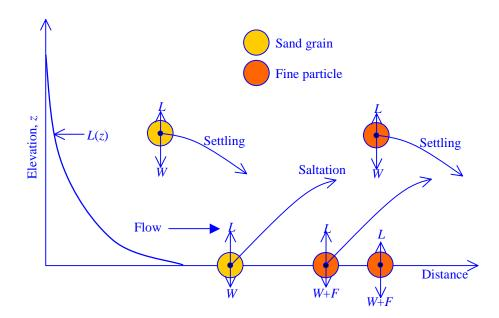
Figure F.4 Condition for incipient motion for sand grains and fine particles.
