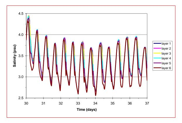
Figure C.8 Cedar River salinity time series at BC6, with layer 1 being the bottom layer.
