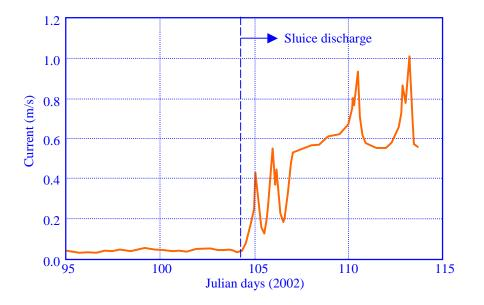
Figure B.2 Effect of S-46 operation (beginning April 14<sup>th</sup>, 2002) on the transport regime in the Southwest Fork: 12-hour-mean current speed derived from Aquadopp.
