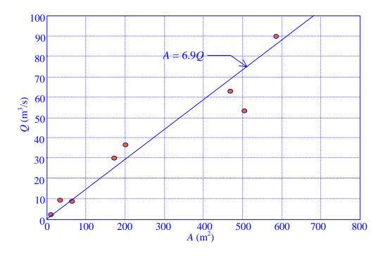
Figure F.2 Mean discharge versus flow area relationship for the Middle St. Johns River.
