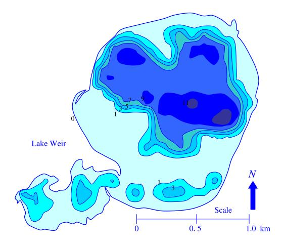
Figure 2.8 Bathymetry of Lake Weir (mud thickness is in feet) (Danek et al. 1991)
