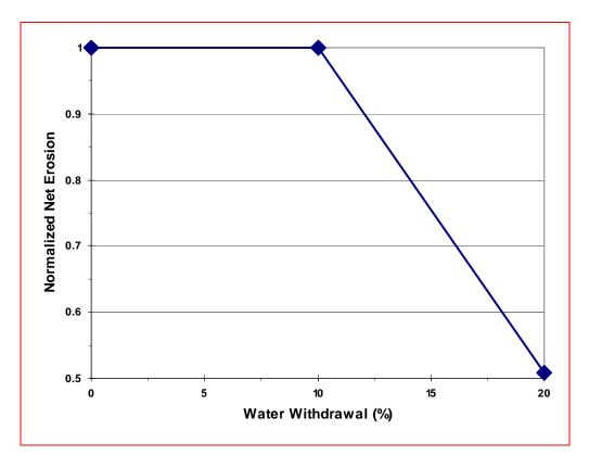
Figure C.17 Normalized net erosion downstream of the water withdrawal site as a function of percentage of water withdrawal for Model 2b with the unsteady hydrograph.
