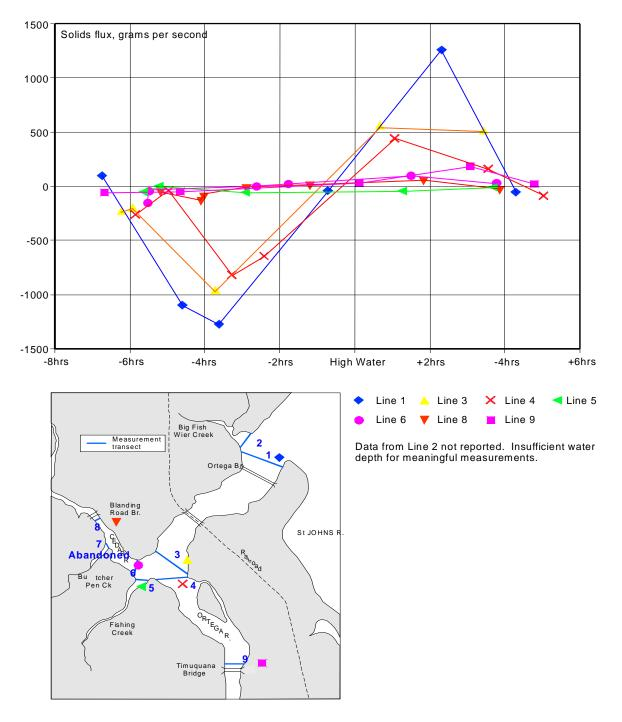
Figure 2.5 Sediment flux data measured with an Acoustic Doppler Current Profiler (ADCP) in Cedar and Ortega Rivers (Mehta et al. 2004)
