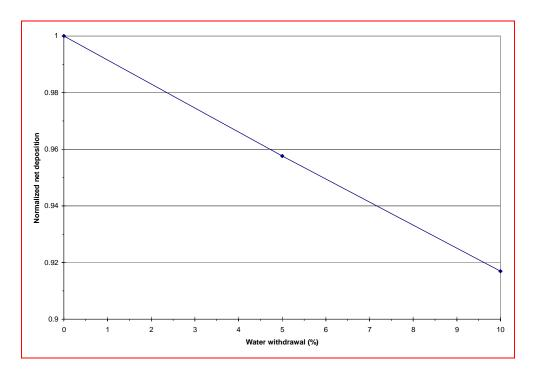
Figure C.16 Normalized net deposition downstream of the water withdrawal site as a function of percentage of water withdrawal for Model 2b.
