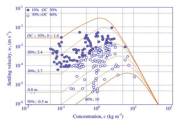
Fig. D.14 Settling velocity variation with concentration for Newnans Lake sediment.
