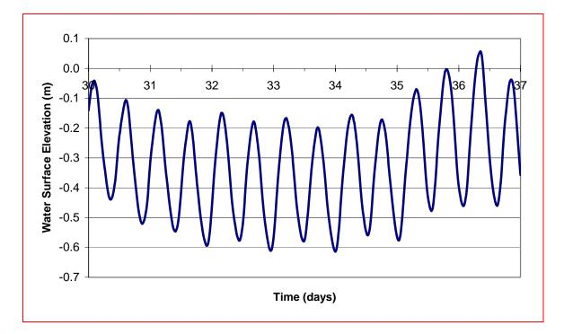
Figure C.7 Tidal signal used for the CR hydrodynamic boundary condition at BC6.
