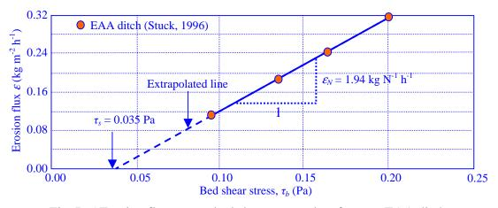
Fig. D.5 Erosion flux versus bed shear stress; data from an EAA ditch.
