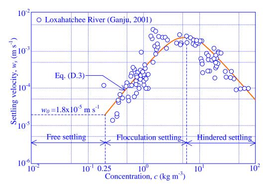
Fig. D.9 Settling velocity variation with concentration for Loxahatchee River sediment.
