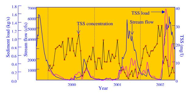
Figure 2.1 Stream flow discharge, total suspended solids concentration and sediment load data in St. Johns River near Christmas (Kroening 2004)
