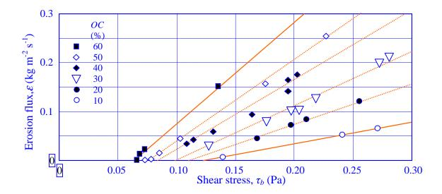
Fig. D.13 Erosion flux versus bed shear stress with lines of constant *OC*; data from Newnans Lake.
