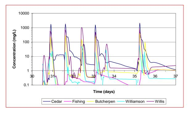
Figure C.6 Suspended sediment concentration time series for the Cedar River at BC1 – BC5.
