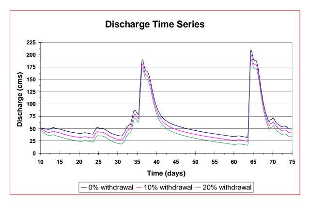
Figure C.10 Discharge time series at mid-channel for scenarios 16-18.
