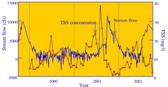
Figure 2.2 Stream flow discharge and total suspended solids concentration data in St. Johns River near Deland (Kroening 2004)
