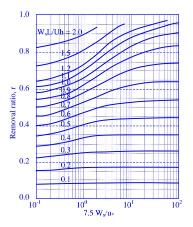
Figure C.20 Graph for calculating the removal ratio for a two-entrance basin.
