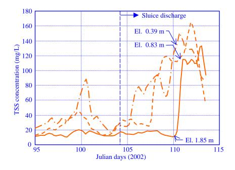
Figure B.5 Effect of S-46 operation on the transport regime in the Southwest Fork: 12-hour-mean TSS concentration data using OBS at three elevations from bottom.
