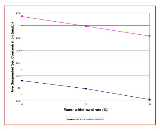
Figure C.15 Average suspended sediment concentration at downstream end of channel as a function of percentage of water withdrawal.
