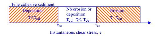
Figure F.5 Conditions for erosion and deposition of sand and fine cohesive sediment.
