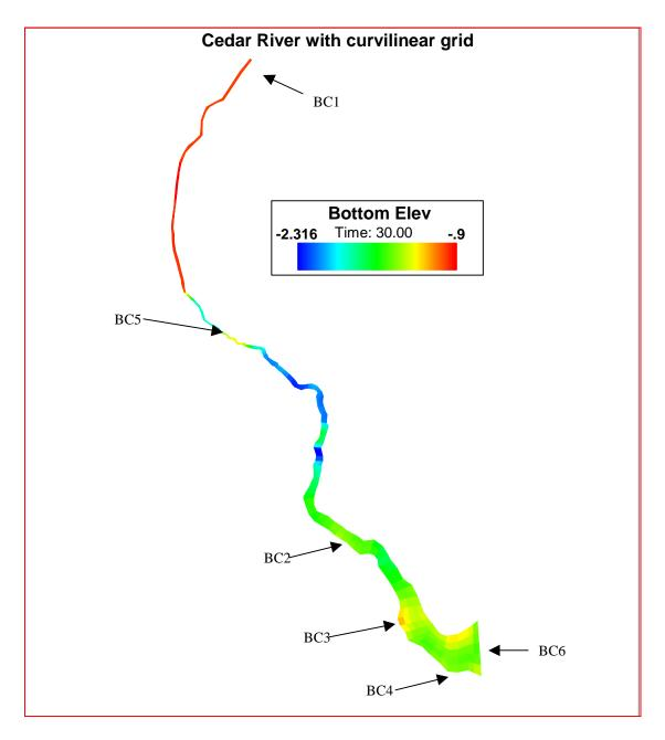
Figure C.2 Bathymetry of the Cedar River modeling domain. Bottom elevations are in meters with respect to NGVD. BC1 – Cedar River; BC2 – Williamson Creek; BC3 – Butcher Pen Creek; BC4 – Fishing Creek; BC5 – Willis Branch.
