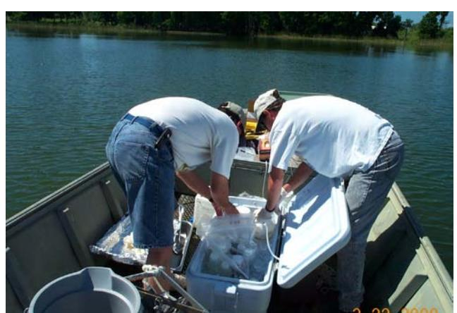
1 and 2. Subsampling sediment from mixing tray to sample jars; 3. Cleaning mixing tray for field blank sample; 4. Sand/sediment from rinse of sampling equipment for field blank sample; 5. Gathering field blank sample into jar; 6. Packing of coolers with sample jars for shipment to laboratory.
