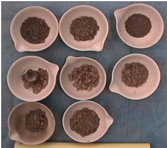
Figure B3. Cedar River sample residues after ignition
