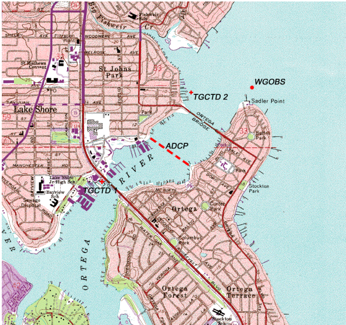
Figure 2 Ortega River mouth at the St. Johns River and instrument deployment. Legend: TGCTD 1 and TGCTD 2 = Locations of water level and CTD gages; WGOBS = Location of the wave gage point-current meter and OBS sensors; ADCP = ADCP transect.
