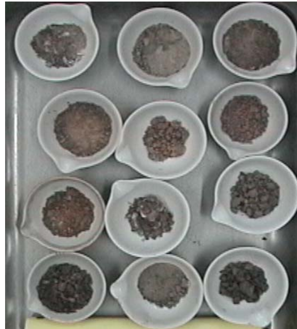
Figure B4. Ortega River sample residues after ignition
