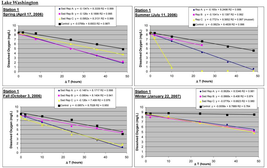
**Figure 12.** Seasonal dissolved oxygen concentration depletion in the sediment and control (surface water only) replicate cores collected at station 1 of Lake Washington.
