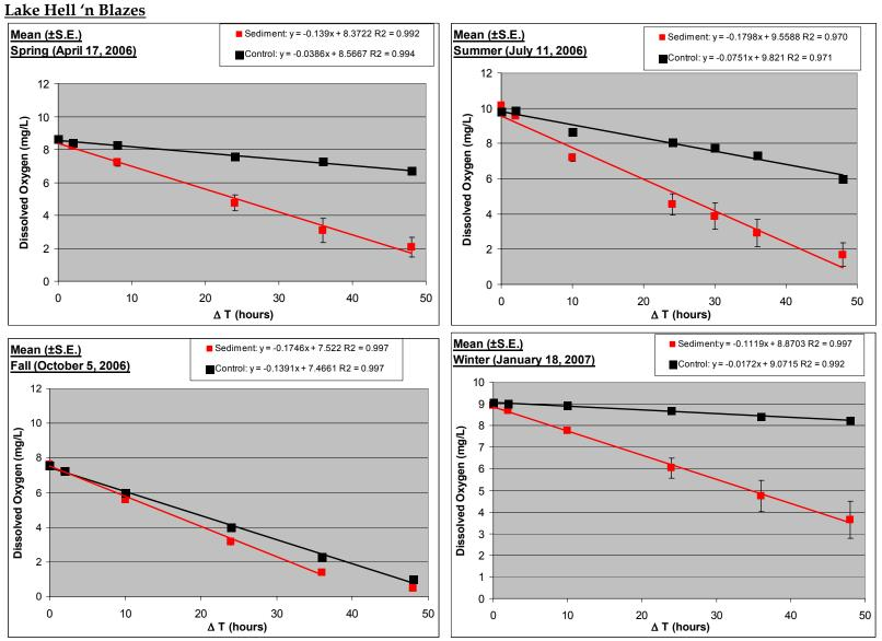
**Figure 11.** Mean and standard error (S.E.) seasonal dissolved oxygen concentration depletion in the sediment (n=3) and control (surface water only) (n=1) cores collected in Lake Hell 'n Blazes.
