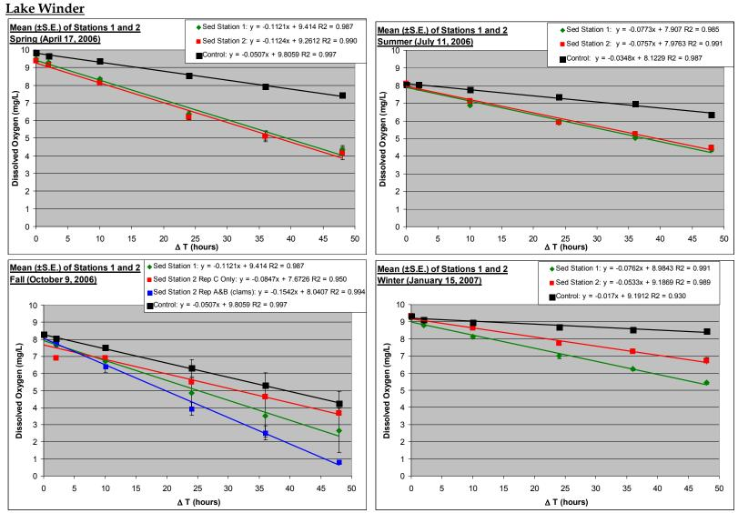
**Figure 4.** Mean and standard error (S.E.) seasonal dissolved oxygen concentration depletion in the sediment (n=3) and control (surface water only) (n=2) cores collected at stations 1 and 2 of Lake Winder.
