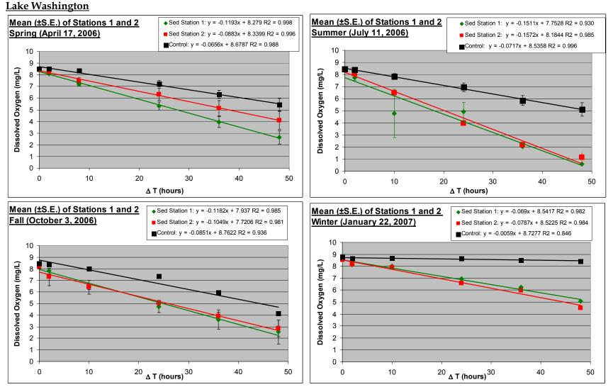
**Figure 14.** Mean and standard error (S.E.) seasonal dissolved oxygen concentration depletion in the sediment (n=3) and control (surface water only) (n=2) collected at both stations of Lake Washington.
