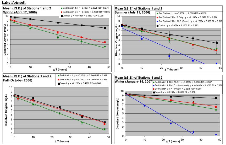
**Figure 7.** Mean and standard error (S.E.) seasonal dissolved oxygen concentration depletion in the sediment (n=3) and control (surface water only) (n=2) cores collected at stations 1 and 2 of Lake Poinsett.
