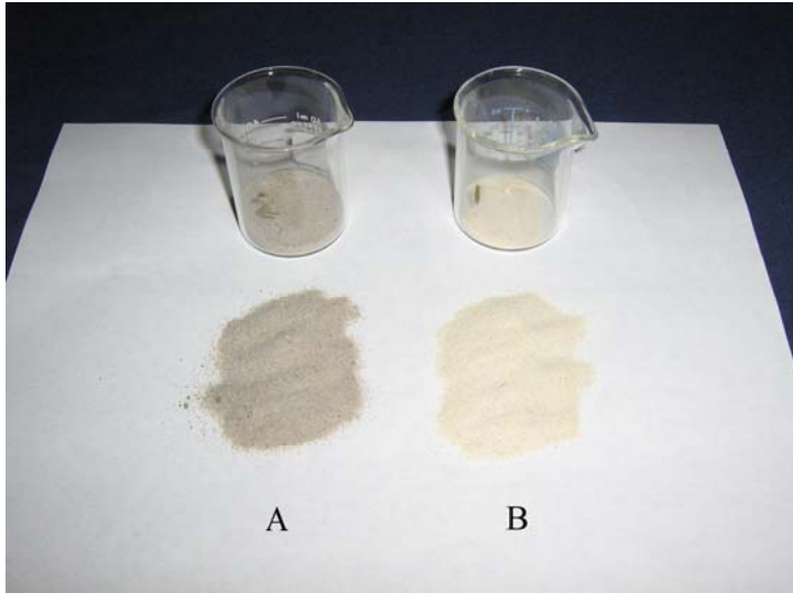
Figure 9. Soil sample combusted at 450°C for 8 h (A) and soil sample combusted at 550°C for 3 h (B)
