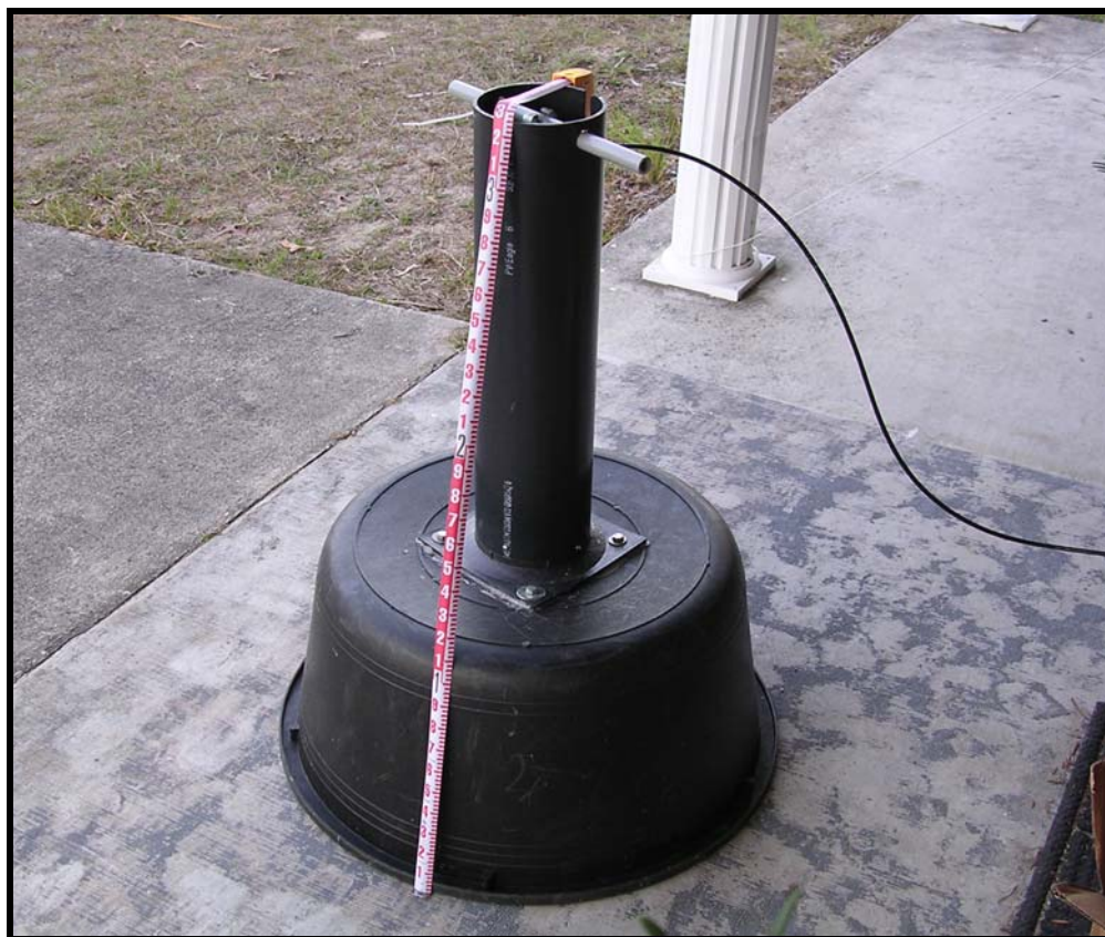
Figure 3. Vent Discharge Capture Device (VDCD). Sensor is attached to and centered on the gray PVC tube at the top of the 0.5 foot diameter pipe.
