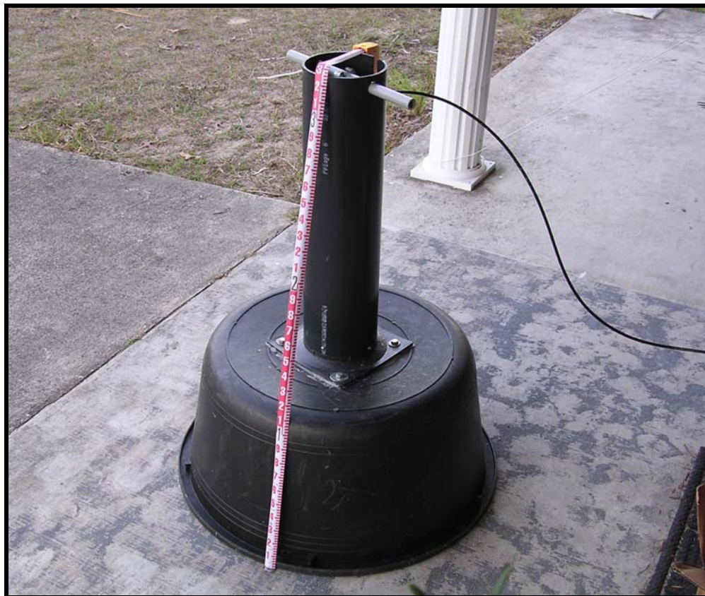
Figure 2. Vent Discharge Capture Device (VDCD). Sensor is attached to and centered on the gray PVC tube at the top of the 0.5 foot diameter pipe.
