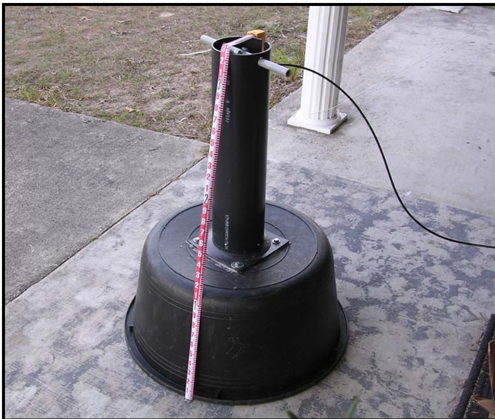
Figure 4. Vent Discharge Capture Device (VDCD). Sensor is attached to and centered on the gray PVC tube at the top of the 0.5 foot diameter pipe.
