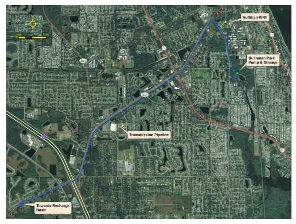
Figure 6. Conceptual pipeline for diversion of stormwater from Halifax Canal system
