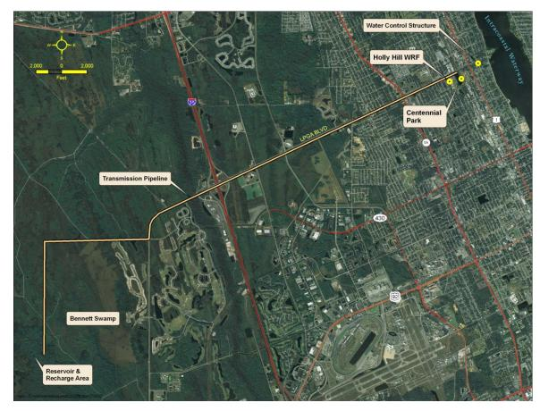
Figure 4. Conceptual pipeline for diversion of stormwater from 11th Street Canal system
