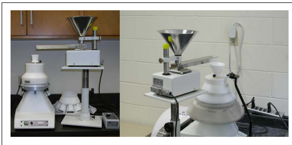
Figure 1. Fritsch rotary cone divider at FDEP/FGS Hydrogeochemistry Laboratory. This unit is accurate to within 0.42%, which is significantly better than the standard “cone and quarter” technique.
