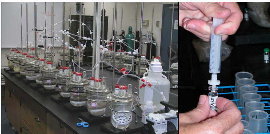
Figure 3. Sealed reaction vessels (mesocosms) with N 2 (gas) lines (left) and filtered sampling for anions analyses (right).
