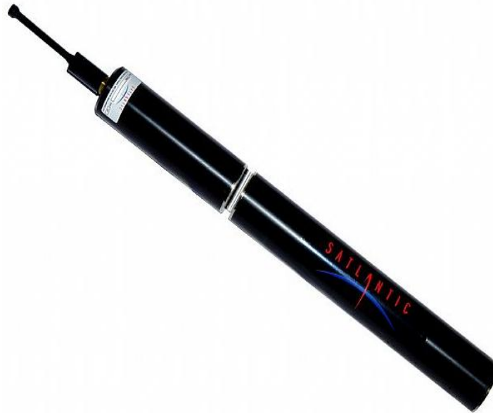
Fig. 2-2 – Photograph of the Satlantic Submersible UV Nitrate Analyzer (SUNA). Data communications occur via the port to the upper left; the sensor requires off-board power and data storage, and is therefore tethered during the entirety of each deployment. The UV-lamp irradiates across the 1-cm gap 1/3 rd down the sensor, passing through the ambient fluid; no flow cell was used during our deployments. A copper guard was inserted in the sensor gap to preclude biofilm development. In addition, the sensor was wrapped in Nitex mesh to prevent benthic invertebrate colonization. Power and data cables were reinforced using garden hoses to prevent impacts from turtles and other herbivores. (Photo Credit: www.satlantic.com/photos/513000_Plastic%20SUNA.jpg )
