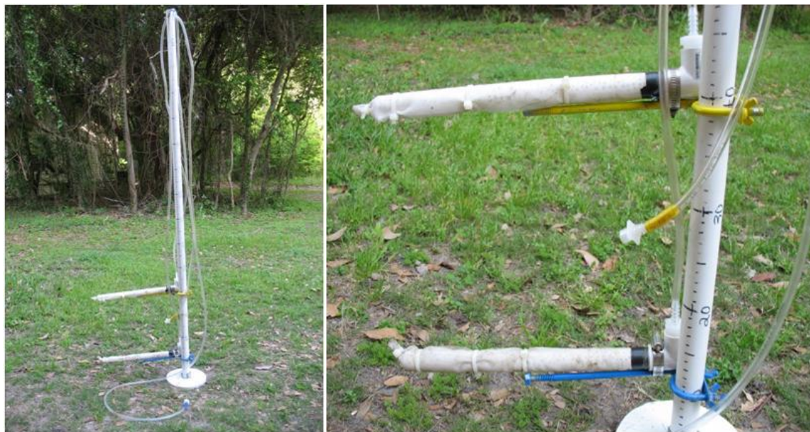
Fig. 7-2. Interstitial water sampler used to collect water within the benthic algal mat and overlying water column at Alexander Springs Creek.
