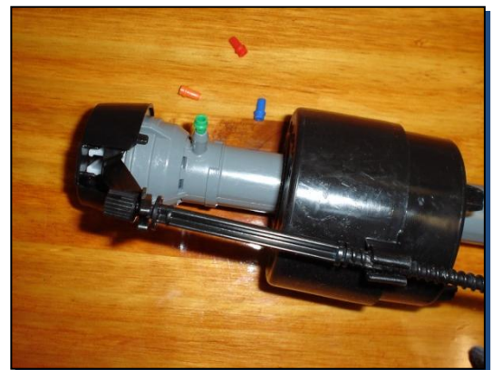
Fluidmaster 400-A fill valve with green flow restrictor inserted in fill tube attachment opening.
