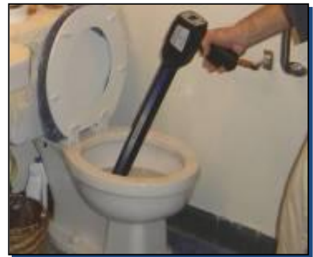
Auditor uses t-5 flushmeter to measure the flush volume of the toilet
