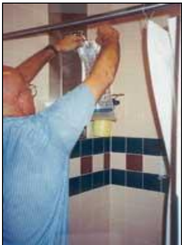
Auditor uses calibrated flow bag to measure showerhead flow rate.
