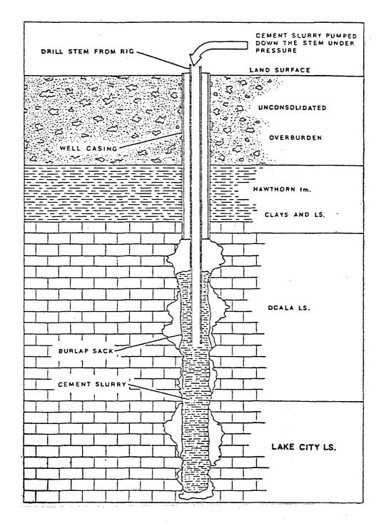
Figure 6. Generalized Cross Section Showing the Placement of the Plug within the Aquifer.
