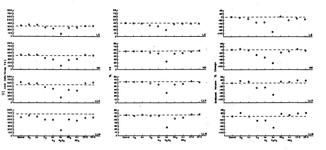
Figure 1. Results of Hanson's (1981) screening study of in situ sediment oxidation techniques. Removal of chemical oxygen demand (COD), percent volatile solids (%VS), and sediment volume change is plotted for each lake and treatment. Treatments are described in Tables 1 and 2.
