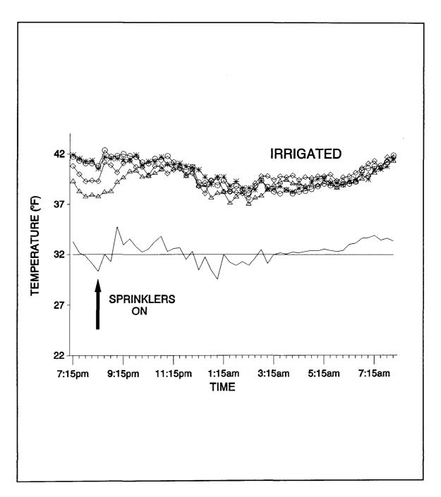
**Figure 6**. Air temperatures inside a shadehouse (-) and under crop covers of 0.62 oz/yd<sup>2</sup> [21  $g \cdot m^{-2}$ ] polyester ( $\Delta$ ) and 0.6 oz/yd<sup>2</sup> [20  $g \cdot m^{-2}$ ] (\*), 1.5 oz/yd<sup>2</sup> [51  $g \cdot m^{-2}$ ] ( $\diamond$ ), and 1.9 oz/yd<sup>2</sup> [64  $g \cdot m^{-2}$ ] ( $\bigcirc$ ) polypropylene (Stamps, 1991).
