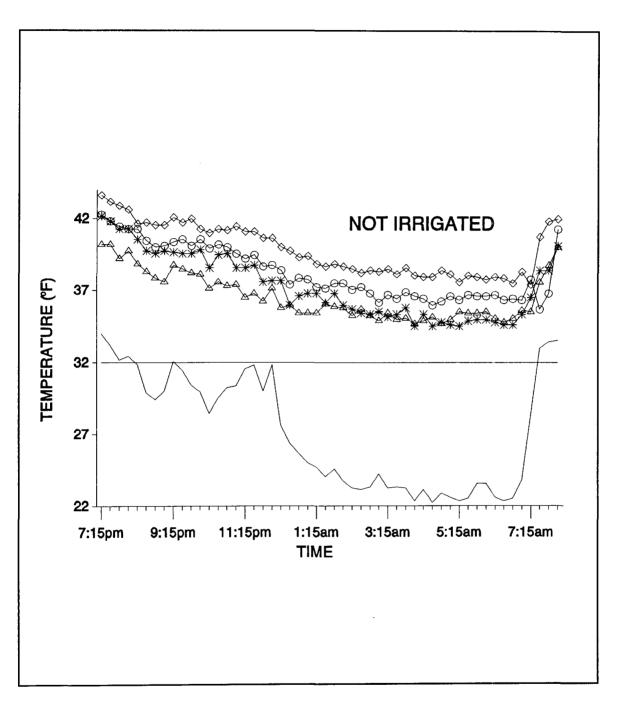
**Figure 5.** Air temperatures inside a shadehouse (-) and under crop covers of 0.62 oz/yd<sup>2</sup> [21 g·m<sup>-2</sup>] polyester ( $\Delta$ ) and 0.6 oz/yd<sup>2</sup> [20 g·m<sup>-2</sup>] (\*), 1.5 oz/yd<sup>2</sup> [51 g·m<sup>-2</sup>] ( $\diamond$ ), and 1.9 oz/yd<sup>2</sup> [64 g·m<sup>-2</sup>] ( $\bigcirc$ ) polypropylene (Stamps, 1991).
