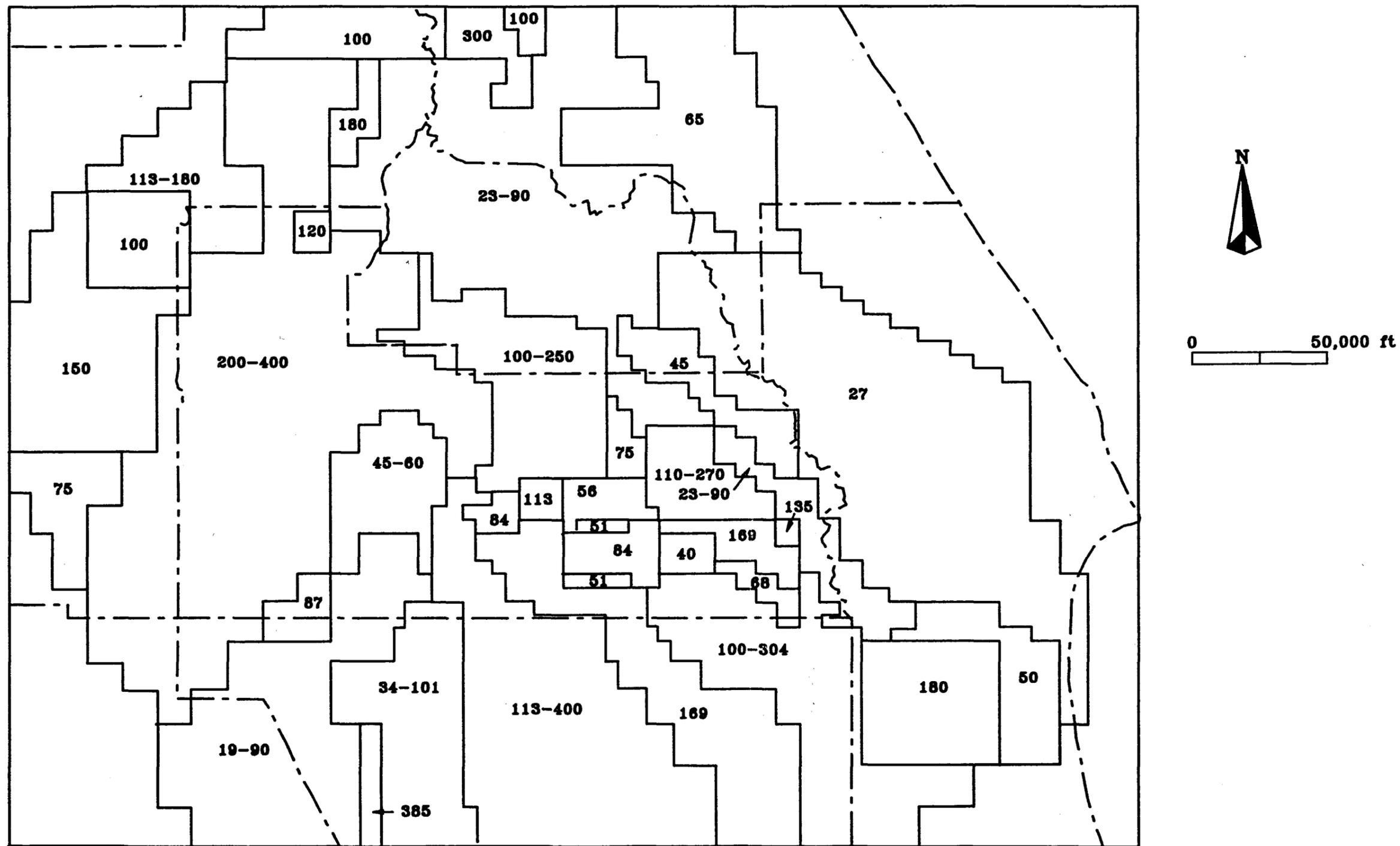
Figure 5.5b. Upper Floridan transmissivity in thousands of  $\text{ft}^2/\text{d}$ .
