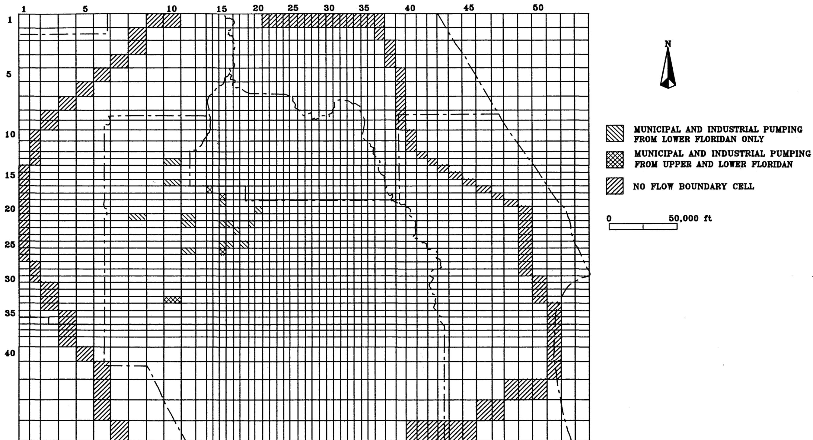
Figure 4.5. MI pumping locations and boundary conditions for Lower Floridan (model layer 2).
