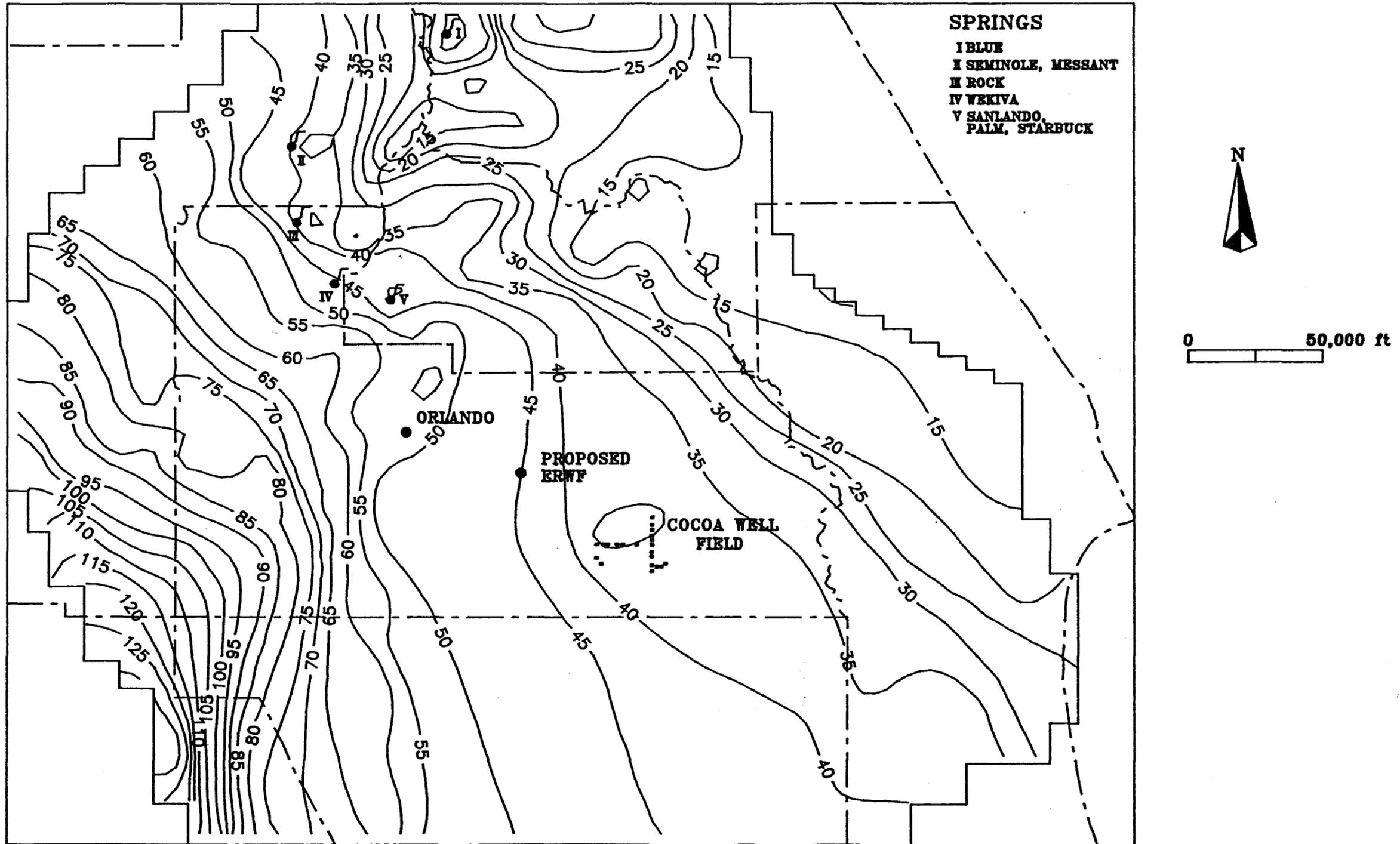
Figure 4.3. Upper Floridan potentiometric surface map for September, 1988 in feet above msl. Reproduced from Rodis, 1989.
