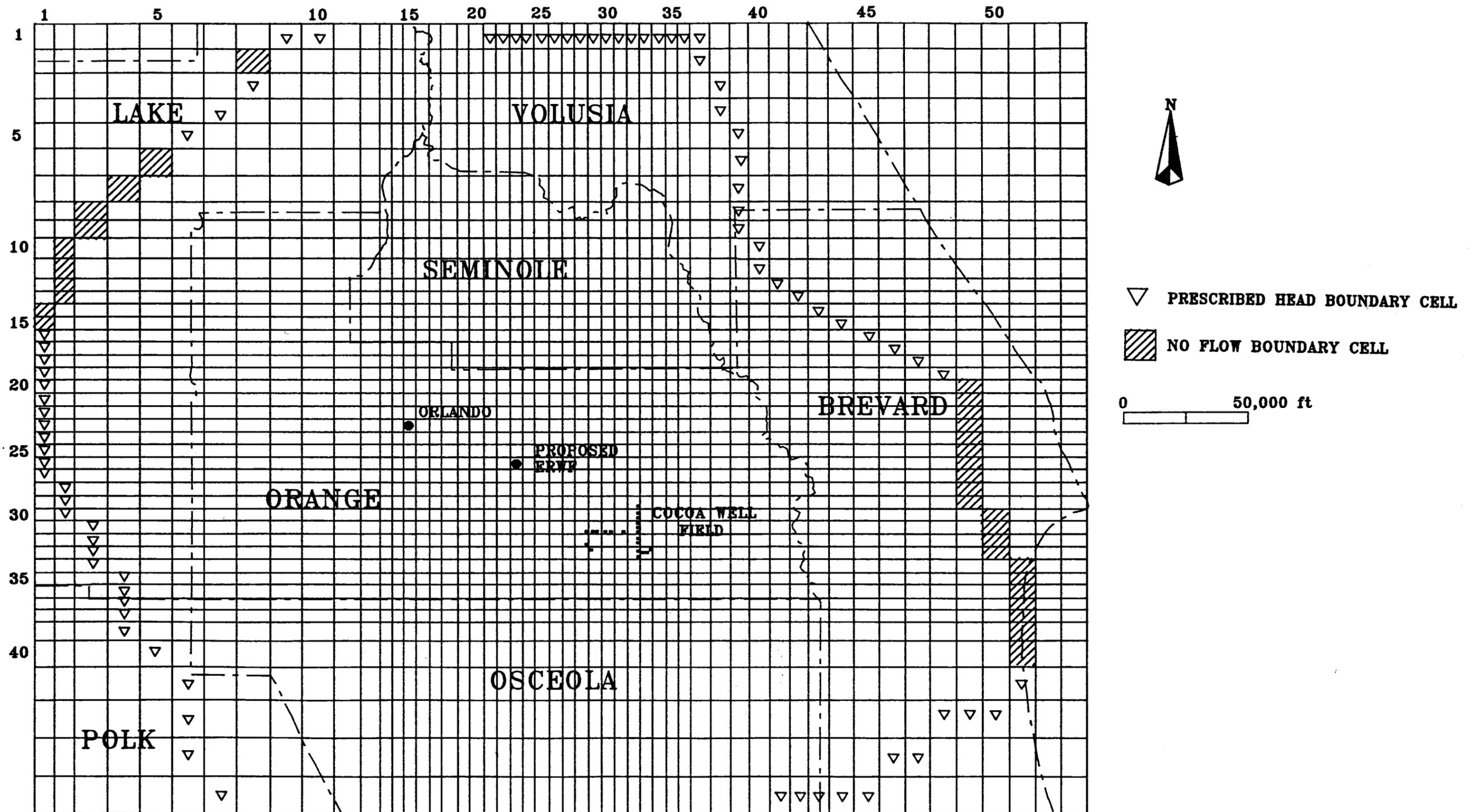
Figure 5.2. Model grid and Upper Floridan boundary conditions used in east-central Florida modeling study.
