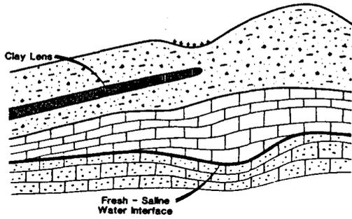
Fig. 9. Schematic geologic section of Floridan aquifer.
