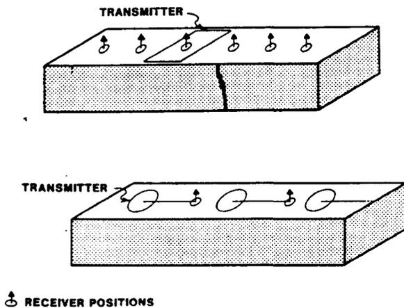
Fig. 12. Transmitter-receiver arrays useful in fracture mapping.
