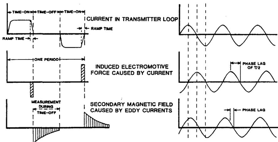
Fig. 1. System waveforms in time domain EM (TDEM) and frequency domain EM (FDEM).
