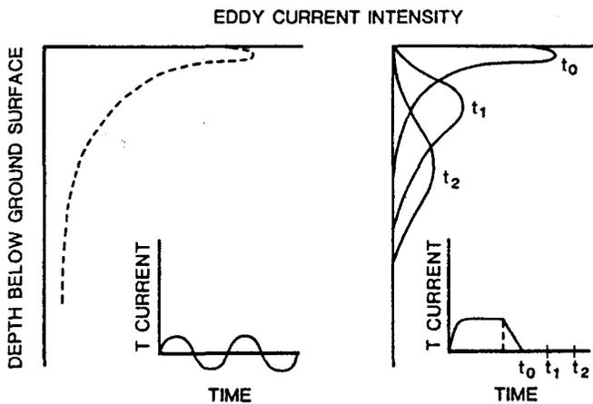
Fig. 10. Eddy current intensity in FDEM and TDEM.
