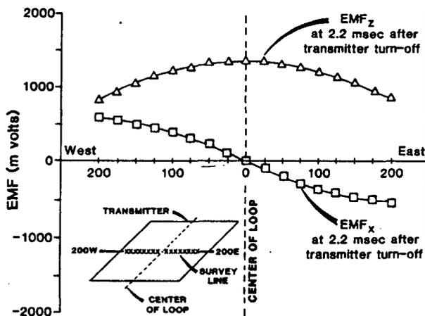
Fig. 5. Spatial behavior of emfs due to vertical ( $emf_z$ ) and horizontal ( $emf_x$ ) magnetic field on a profile through the center of square transmitter loop at one time (2.2 millisecond) after turn-off.
