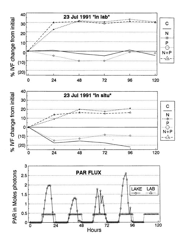
Figure 3.8. Comparison of results from nutrient enrichment bioassays run concurrently in situ and in laboratory. PAR=photosynthetic active radiation for 30 cm water depth in Lake Apopka, Florida and in a laboratory incubator. C=control treatment. N=400 µg N L<sup>-1</sup> as NO<sub>3</sub>. P=40 µg P L-1 as PO<sub>4</sub>. IVF=in vivo fluorescence used as relative biomass indicator.
