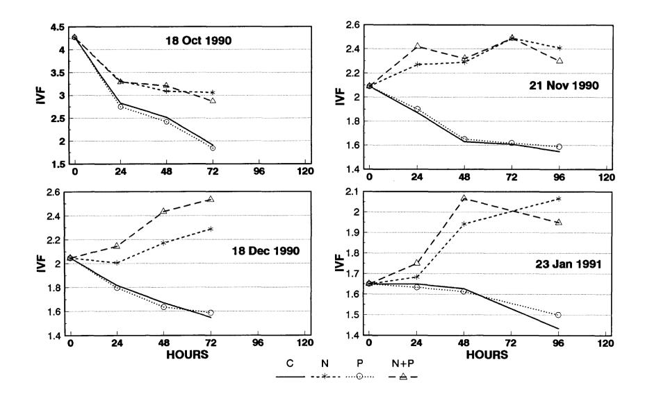
Figure 3.5. Results of nutrient enrichment bioassays run on water collected off Magnolia Park at Lake Apopka, Florida for the months of Oct. 1990-Jan. 1991. C=control. NO<sub>3</sub>=400  $\mu$ g N L<sup>-1</sup>. P=40  $\mu$ g P L<sup>-1</sup>. IVF=*in vivo* fluorescence used as relative biomass indicator for phytoplankton. Hours = time in hours from start of assay.
