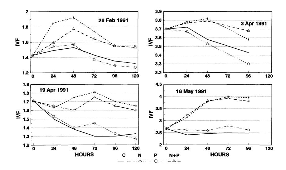
Figure 3.6. Results of nutrient enrichment bioassays run on water collected off Magnolia Park at Lake Apopka, Florida for the months of Feb.-May 1991. C=control.  $NO_3$ =400 µg  $N L^{-1}$ . P=40 µg  $P L^{-1}$ . IVF=*in vivo* fluorescence used as relative biomass indicator for phytoplankton. Hours = time in hours from start of assay.
