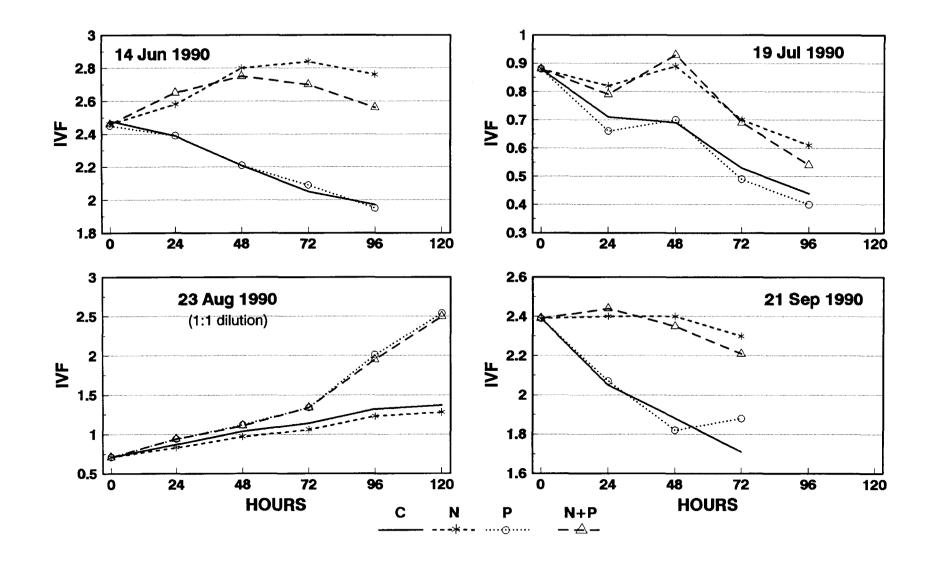
Figure 3.4. Results of nutrient enrichment bioassays run on water collected off Magnolia Park at Lake Apopka, Florida for the months of June-Sept., 1990. C=control. NO<sub>3</sub>=400  $\mu$ g N L<sup>-1</sup>. P=40  $\mu$ g P L<sup>-1</sup>. IVF=*in vivo* fluorescence used as relative biomass indicator for phytoplankton. Hours = time in hours from start of assay.
