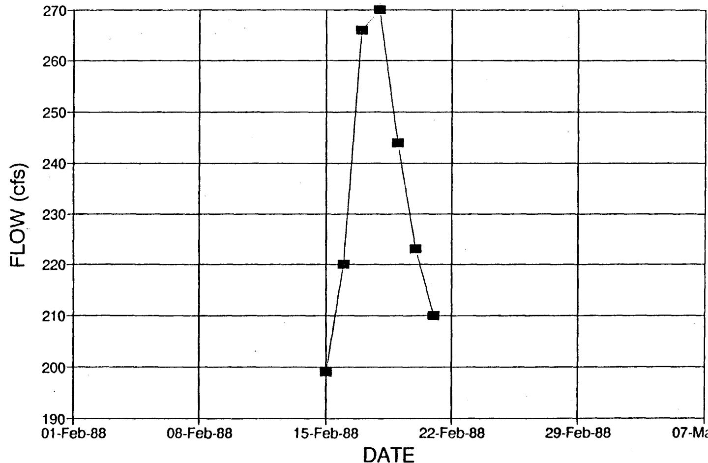
Figure E.1.6 Hydrograph For Estimating Attenuation at Chuluota (February 1988)
