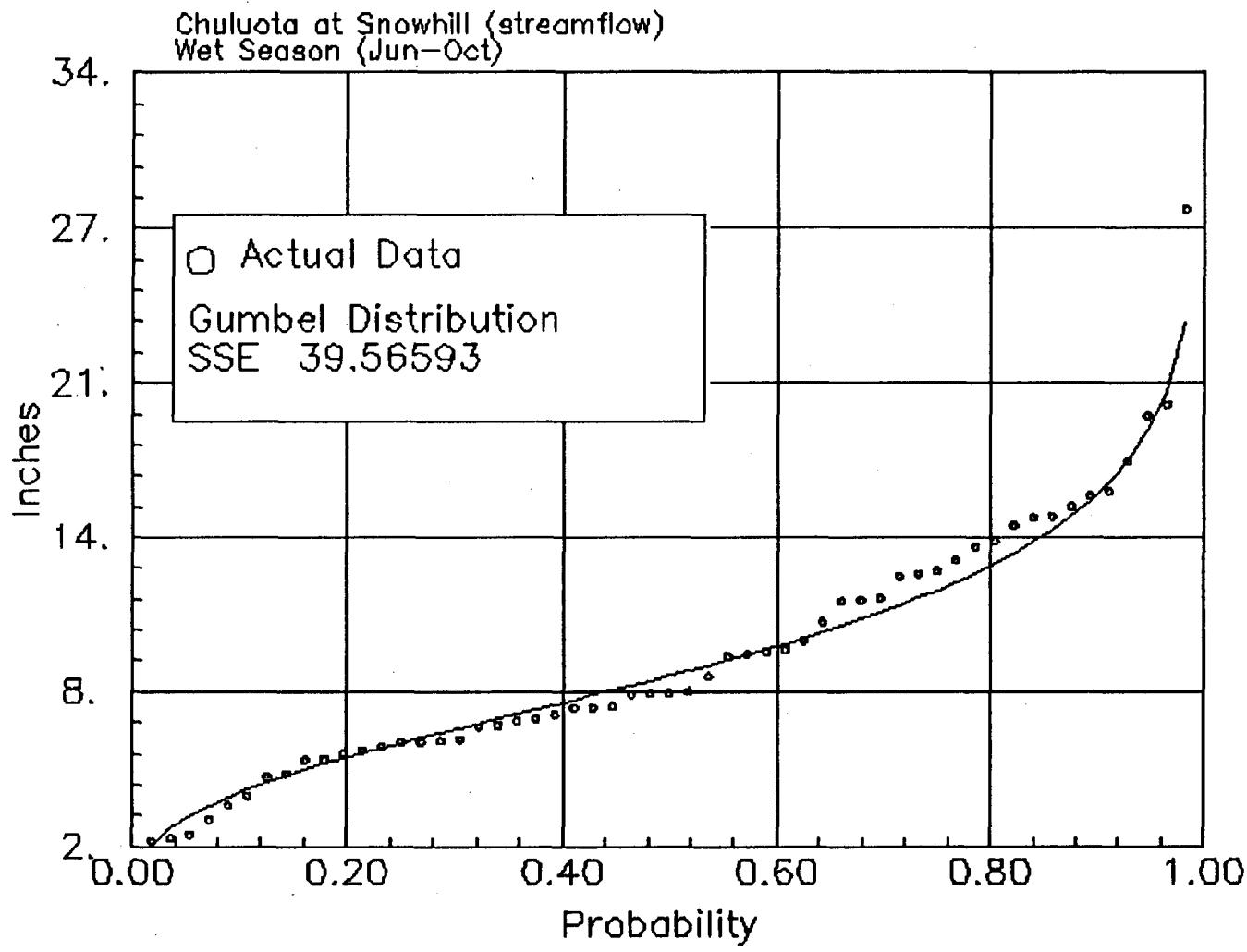
Figure G.1.4 Culuota at Snowhill, Wet Season streamflow distribution for the years of (1936-1990)
