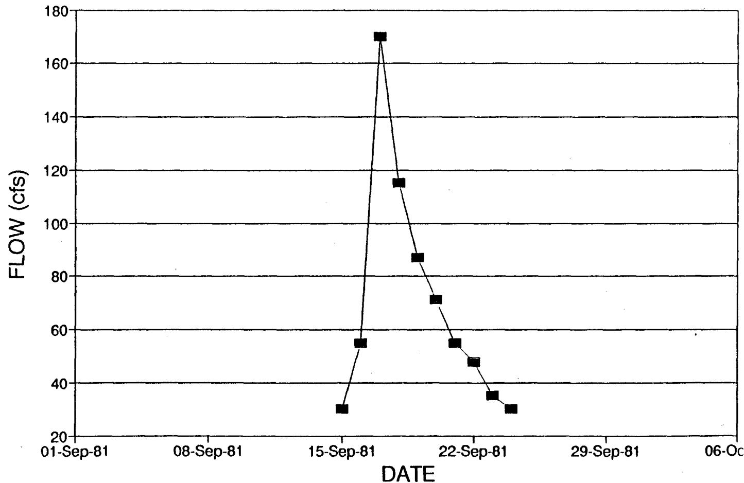
Figure E.3.1 Hydrograph For Estimating Attenuation at Union Park (September 1981)
