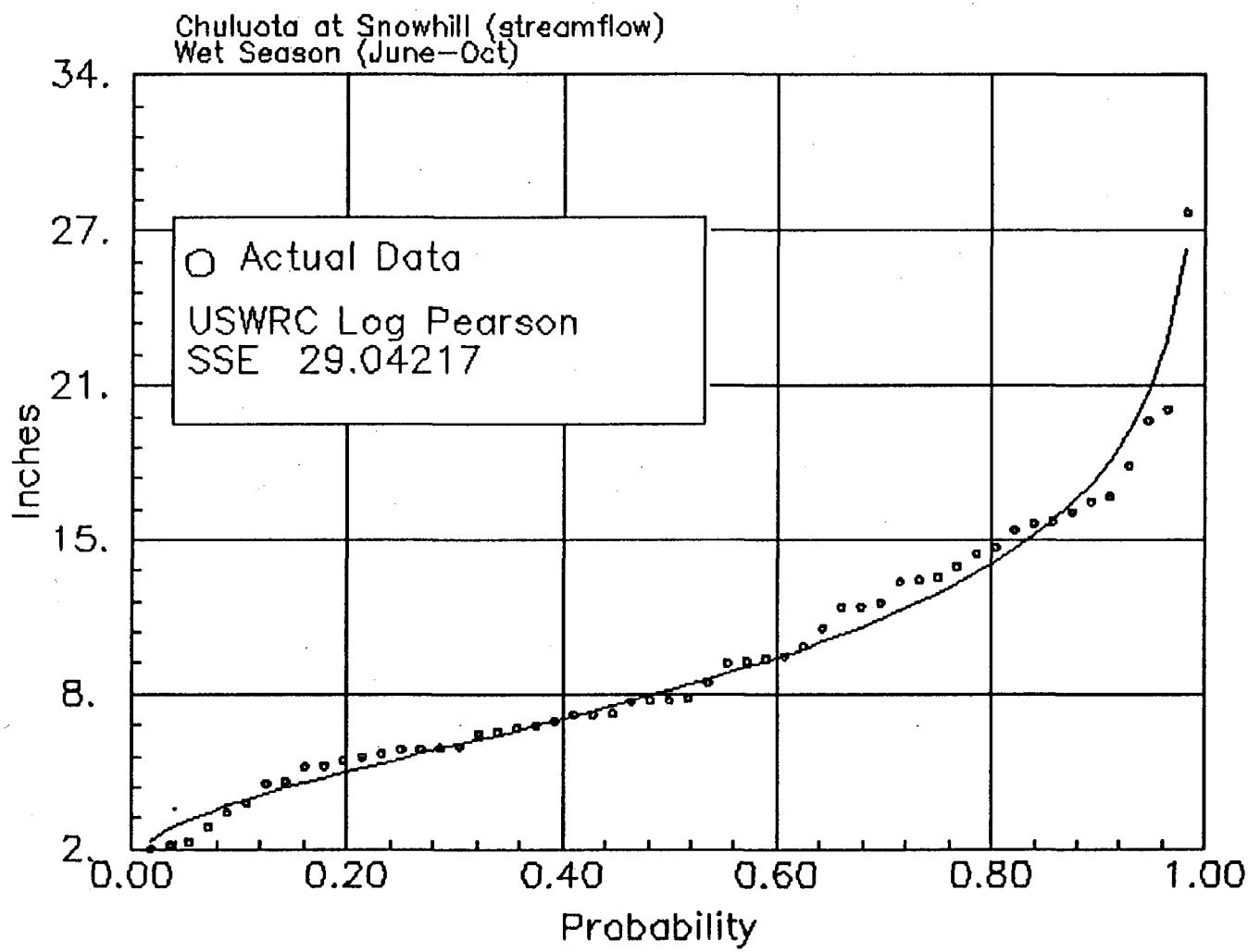
Figure G.1.5 Chuluota at Snowhill, Wet Season streamflow distribution for the years of (1960-1990)
