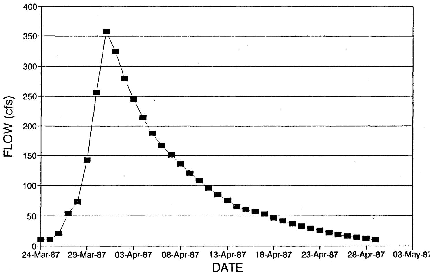
Figure E.2.3 Hydrograph For Estimating Attenuation at Magnolia Ranch (March 1987)
