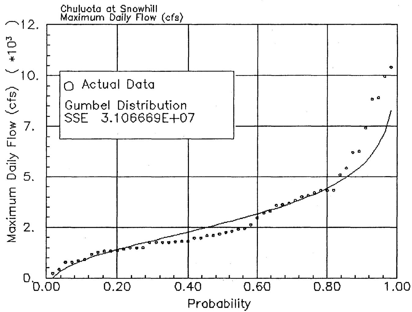
Figure F.1.16 Chuluota at Snowhill, Maximum Daily Flow (cfs) for the Years of 1936–1989.
