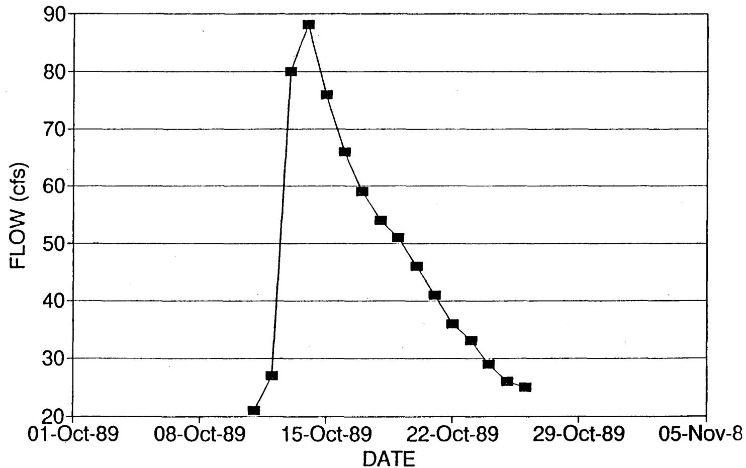
Figure E.2.4 Hydrograph For Estimating Attenuation at Magnolia Ranch (October 1989)
