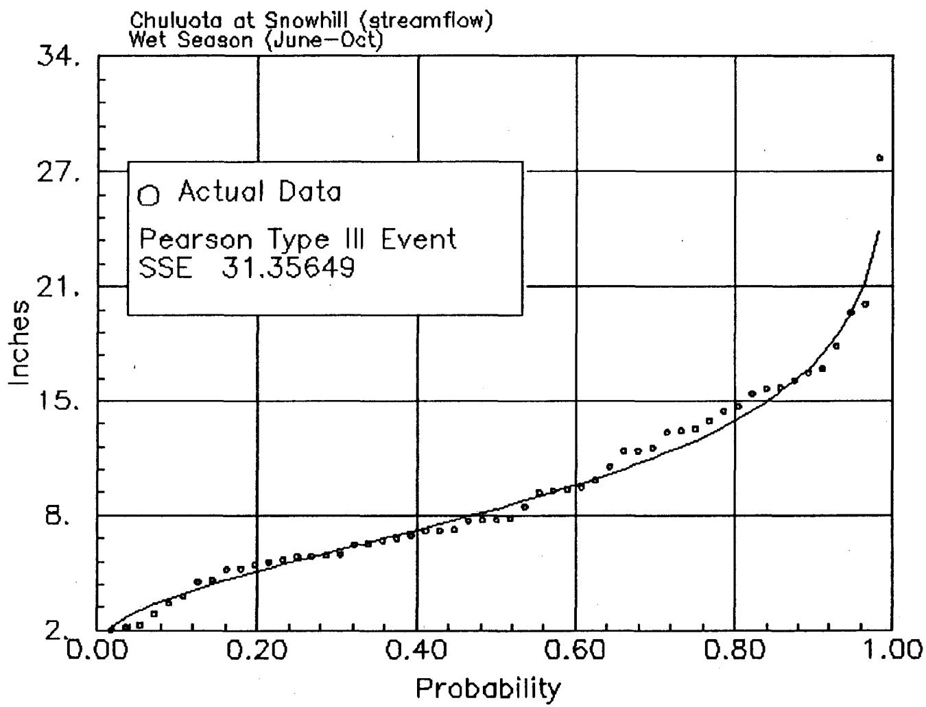
Figure G.1.5 Chuluota at Snowhill, Wet Season streamflow distribution for the years of (1936–1990)
