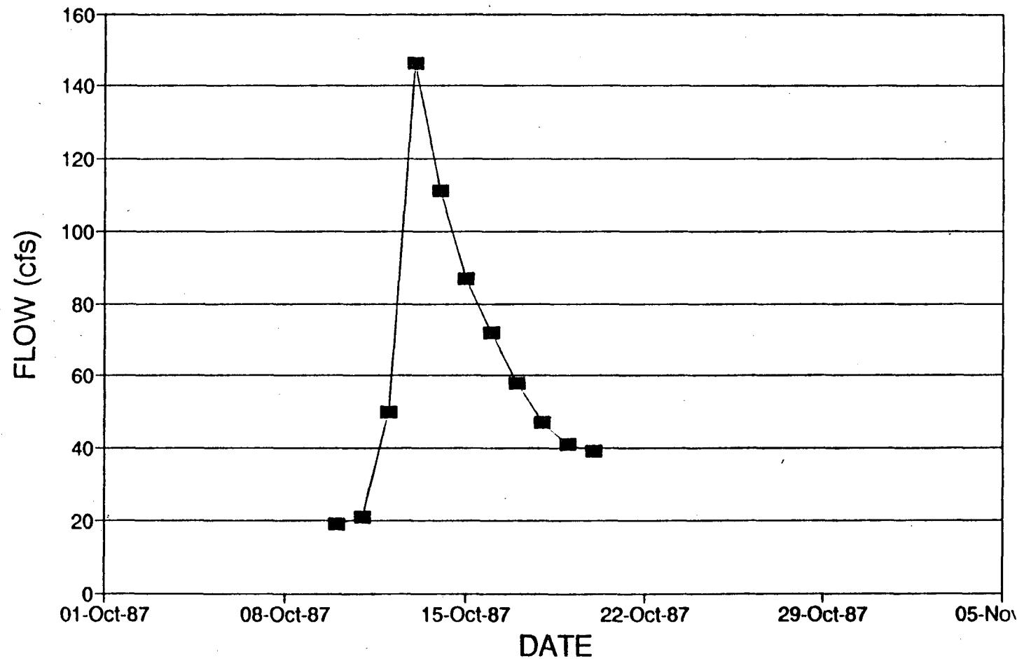
Figure E.3.3 Hydrograph For Estimating Attenuation at Union Park (October 1987)
