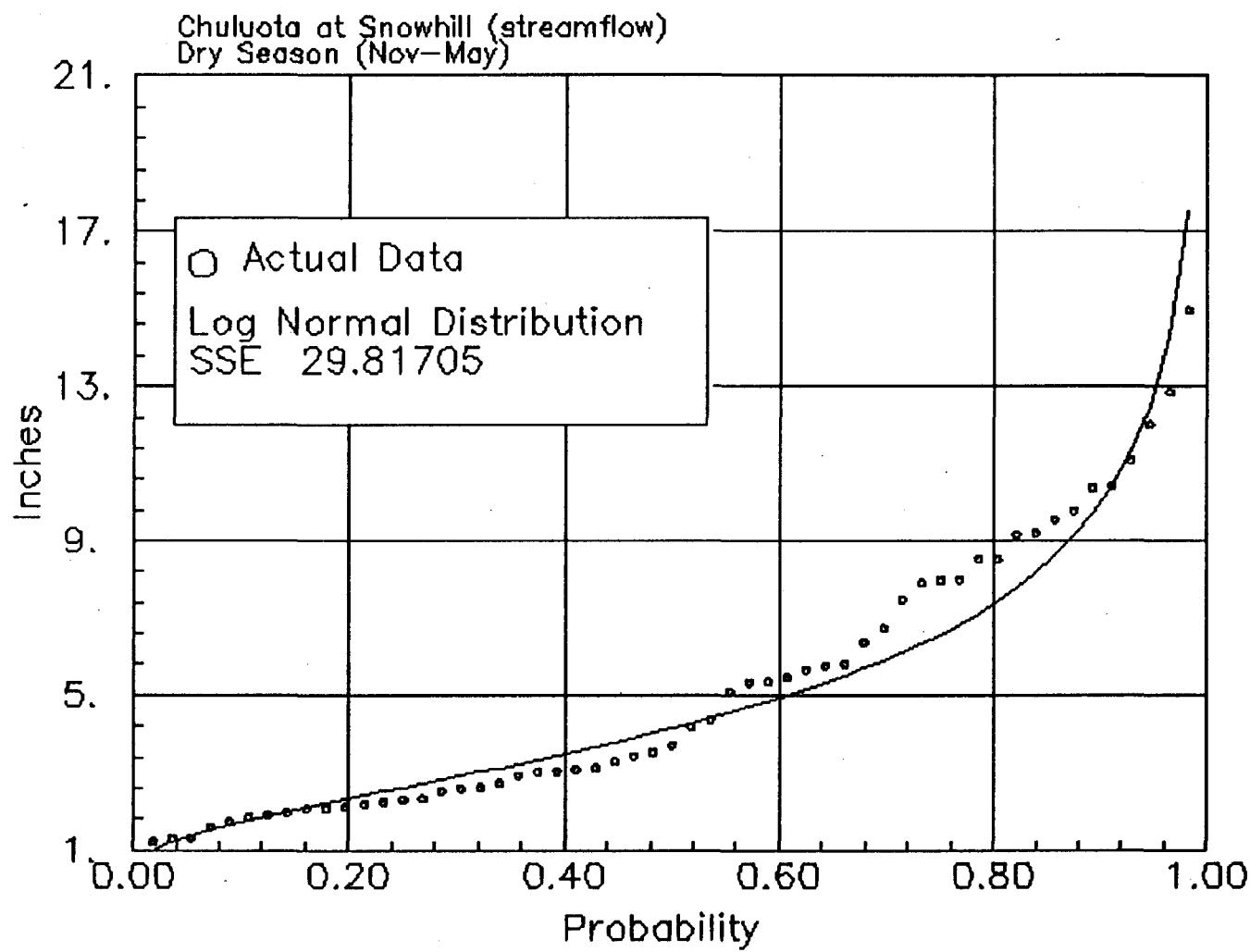
Figure H.1.2 Chuluota at Snowhill, Dry Season streamflow distribution for the years of (1936–1990)
