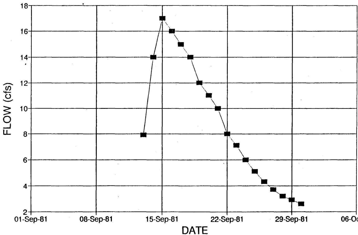
Figure E.2.1 Hydrograph For Estimating Attenuation at Magnolia Ranch (September 1981)
