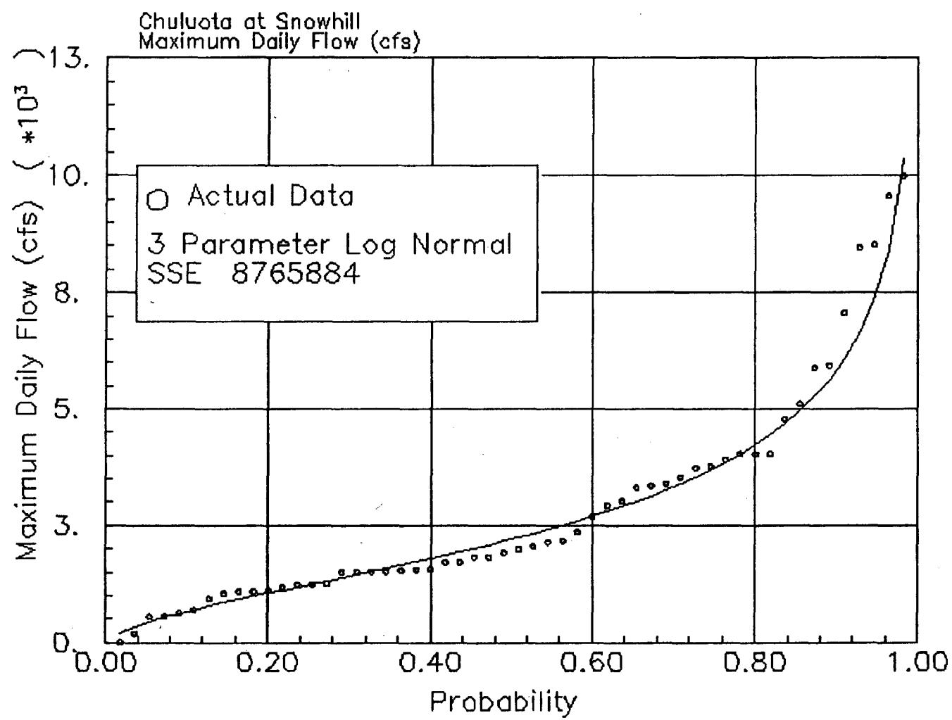
Figure F.1.15 Chuluota at Snowhill, Maximum Daily Flow (cfs) for the Years of 1936-1989.
