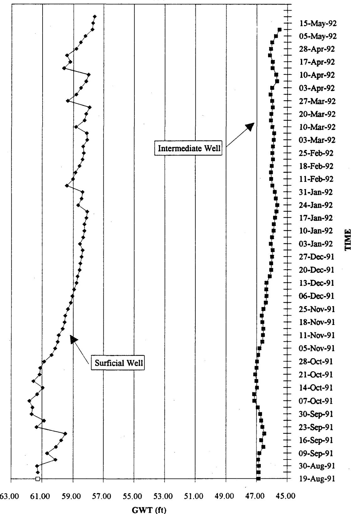
**FIGURE 4.5 Aquifer Elevation Difference at Bithlo 3**
