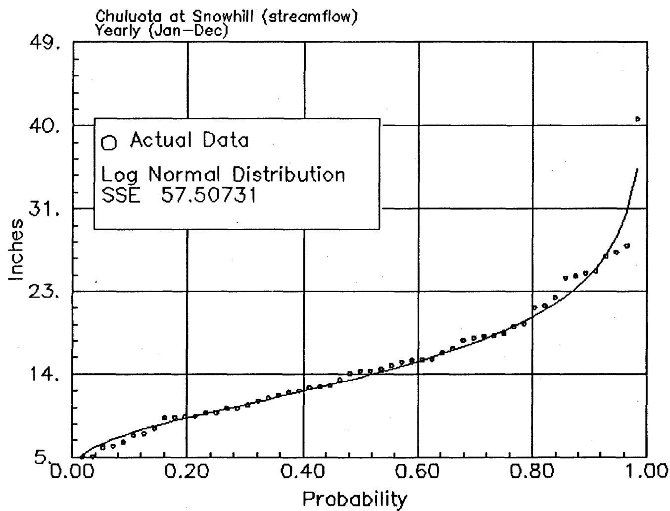
Figure F.1.2 Chuluota at Snowhill, Yearly streamflow distribution for the years of (1936–1990)
