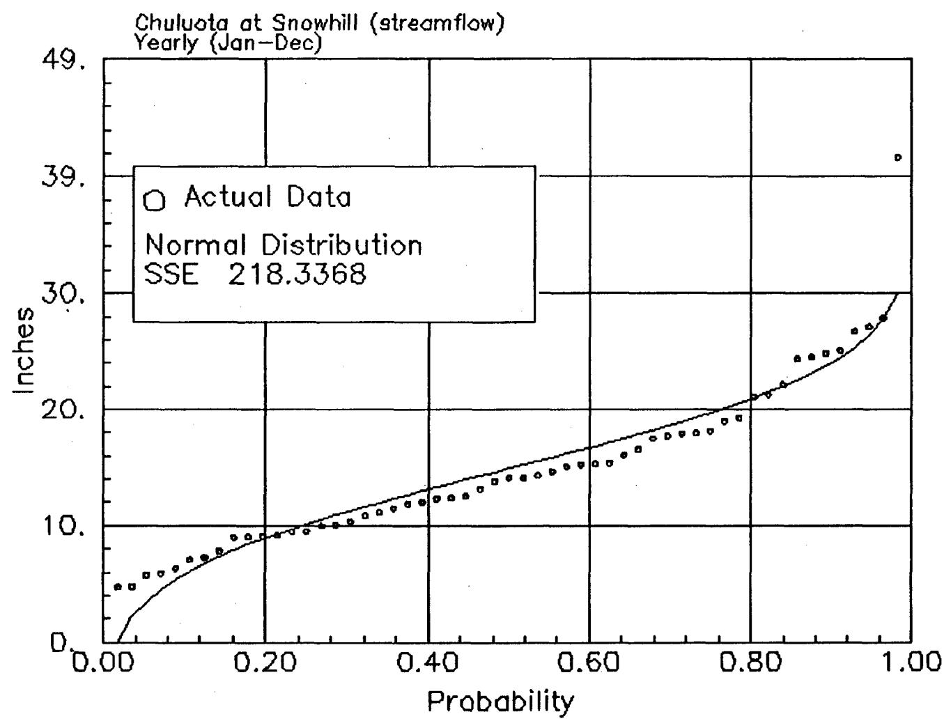
Figure F.1.1 Chuluota at Snowhill, Yearly streamflow distribution for the years of (1936–1990)
