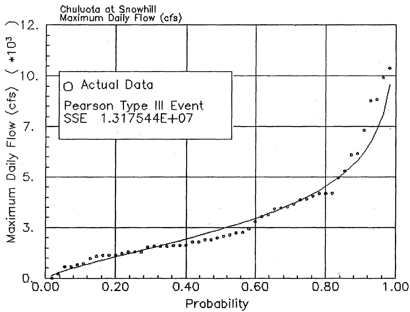
Figure F.1.17 Chuluota at Snowhill, Maximum Daily Flow (cfs) for the Years of 1936–1989.
