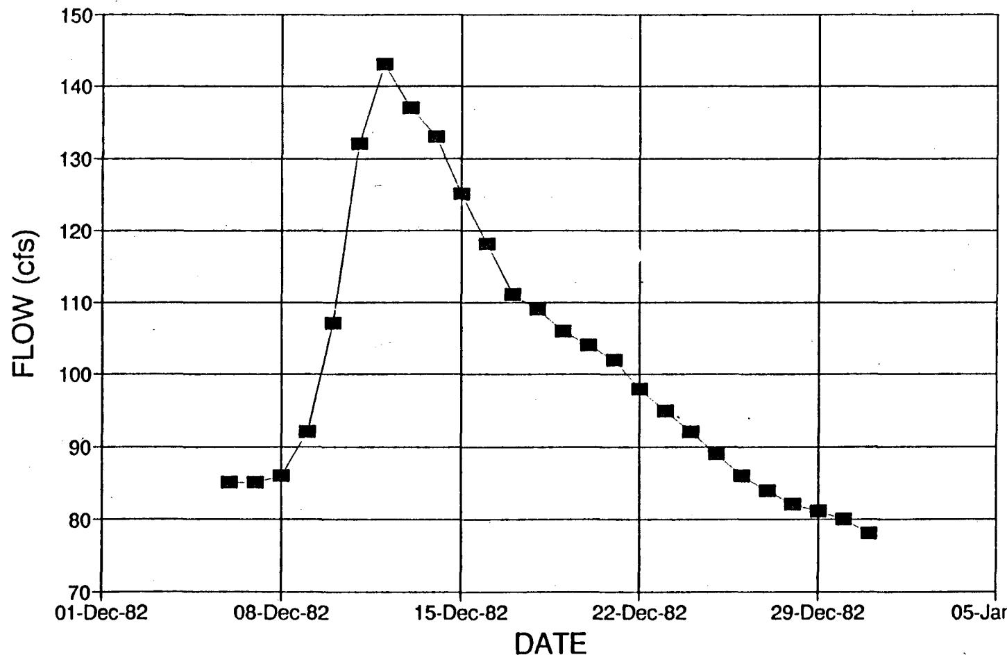
Figure E.1.3 Hydrograph For Estimating Attenuation at Chuluota (December 1982)
