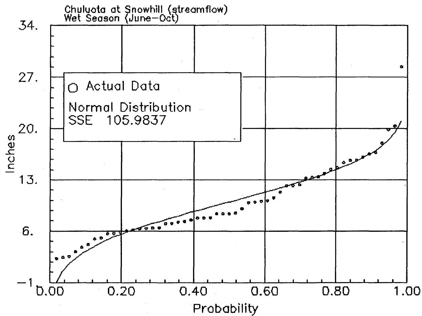
Figure G.1.1 Chuluota at Snowhill, Wet Season streamflow distribution for the years of (1936–1990)
