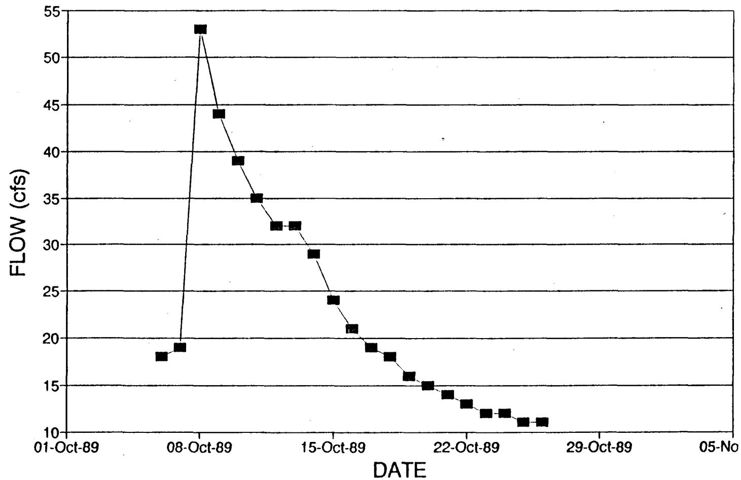
Figure E.3.4 Hydrograph For Estimating Attenuation at Union Park (October 1989)
