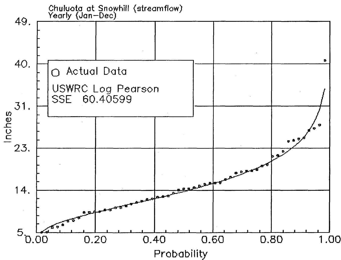
Figure F.1.6 Chuluota at Snowhill, Yearly streamflow distribution for the years of (1936–1990)
