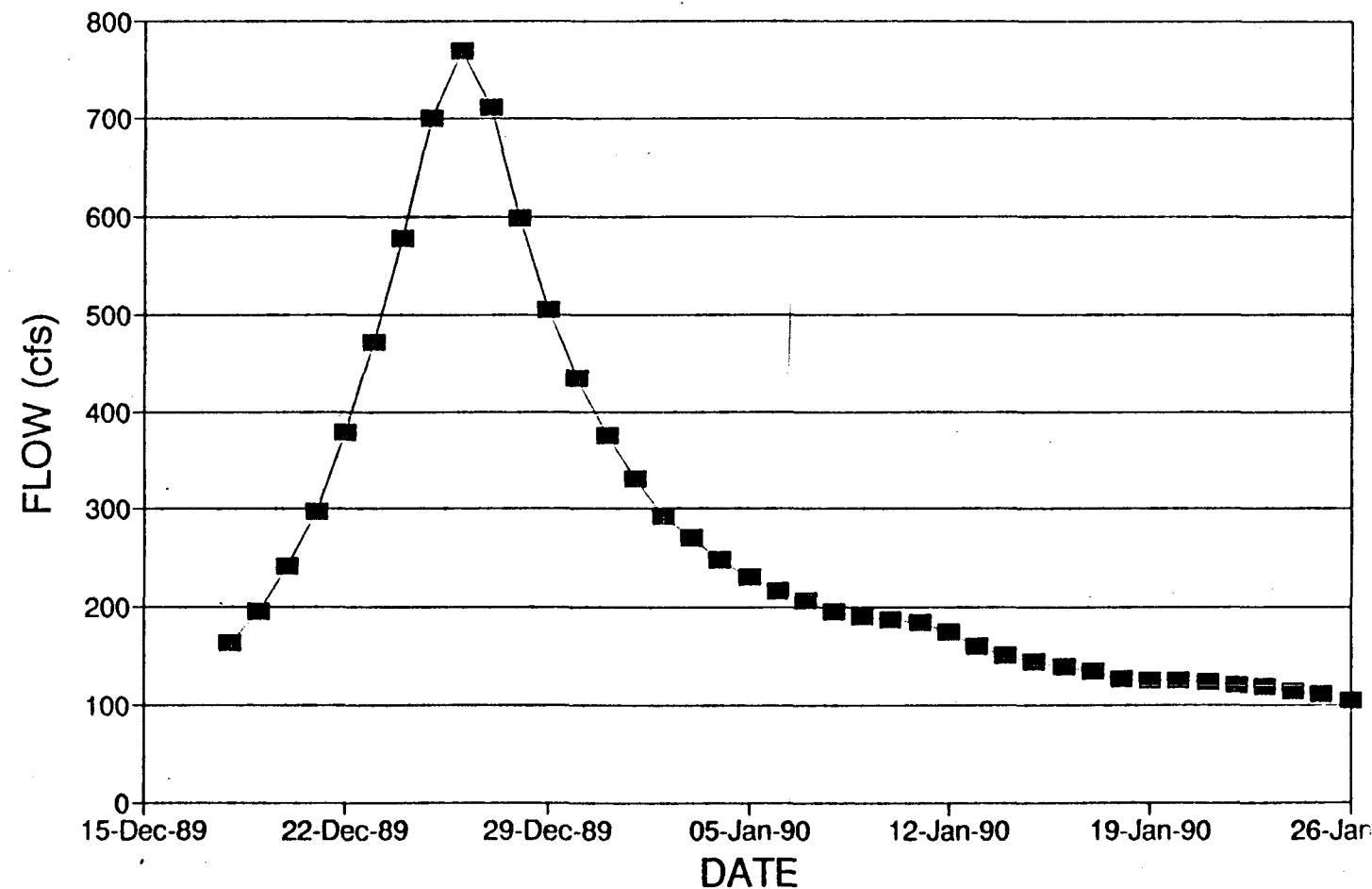
Figure E.1.8 Hydrograph For Estimating Attenuation at Chuluota (December 1989)
