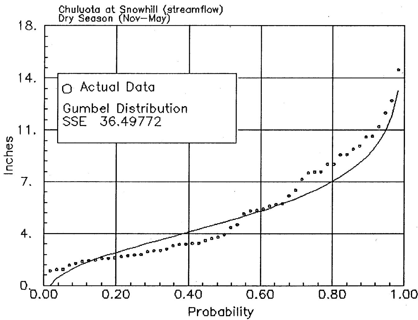
Figure H.1.4 Chuluota at Snowhill, Dry Season streamflow distribution for the years of (1936–1990)
