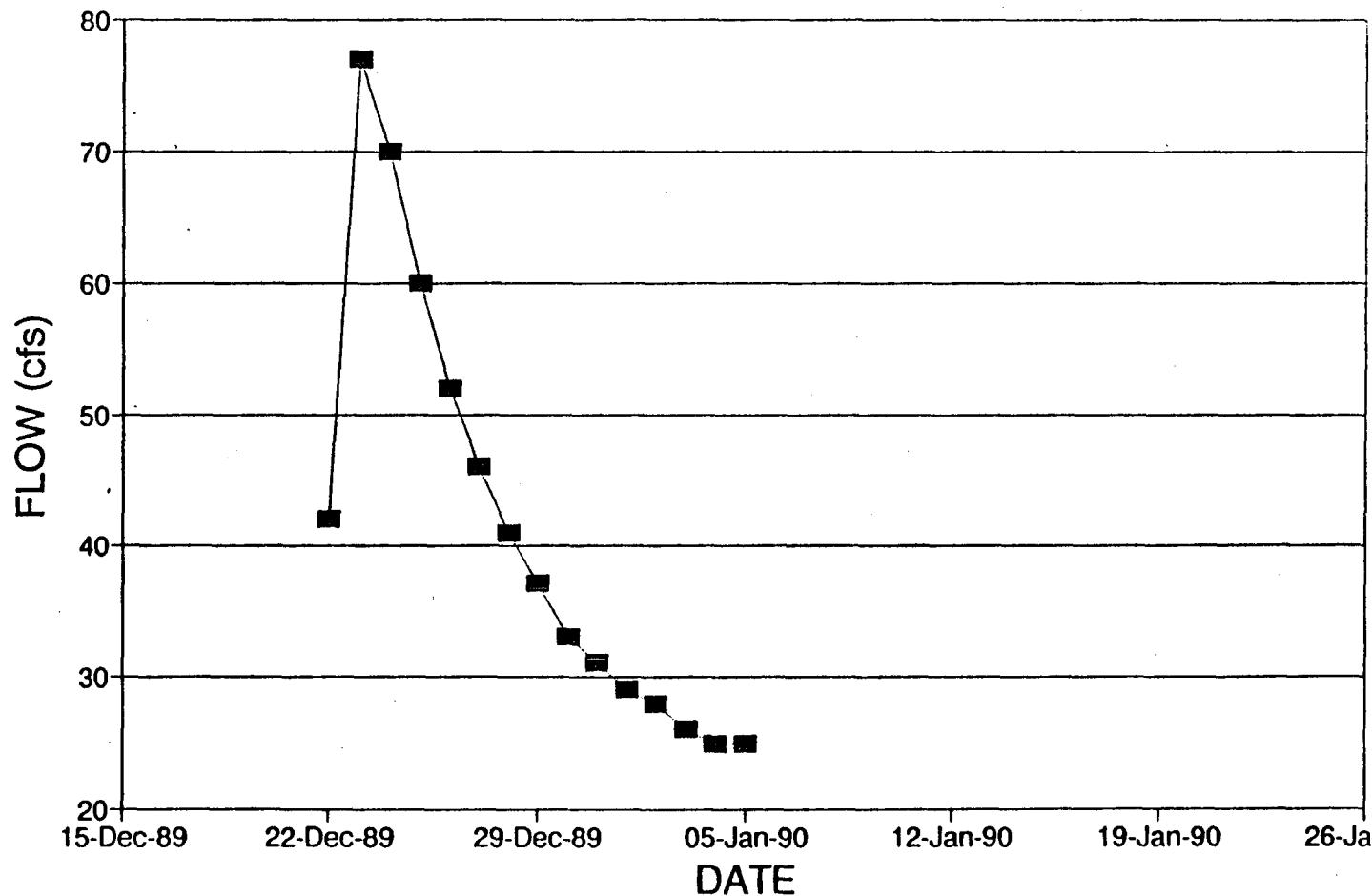
Figure E.3.5 Hydrograph For Estimating Attenuation at Union Park (December 1989)
