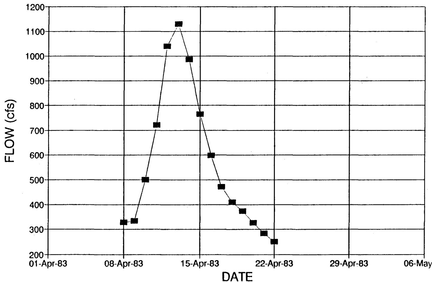
Figure E.1.4 Hydrograph For Estimating Attenuation at Chuluota (April 1983)
