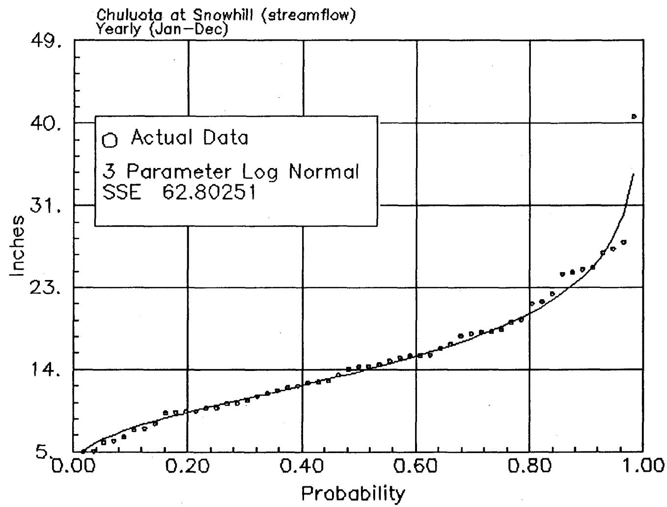
Figure F.1.3 Chuluota at Snowhill, Yearly streamflow distribution for the years of (1936–1990)
