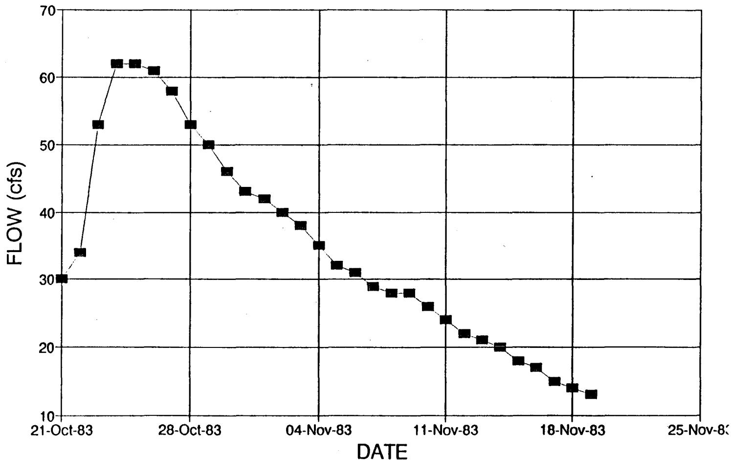
Figure E.2.2 Hydrograph For Estimating Attenuation at Magnolia Ranch (October 1983)
