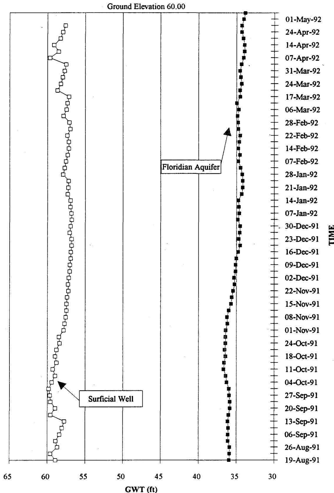
**FIGURE 4.6 Aquifer Elevation Difference at Cocoa K**
