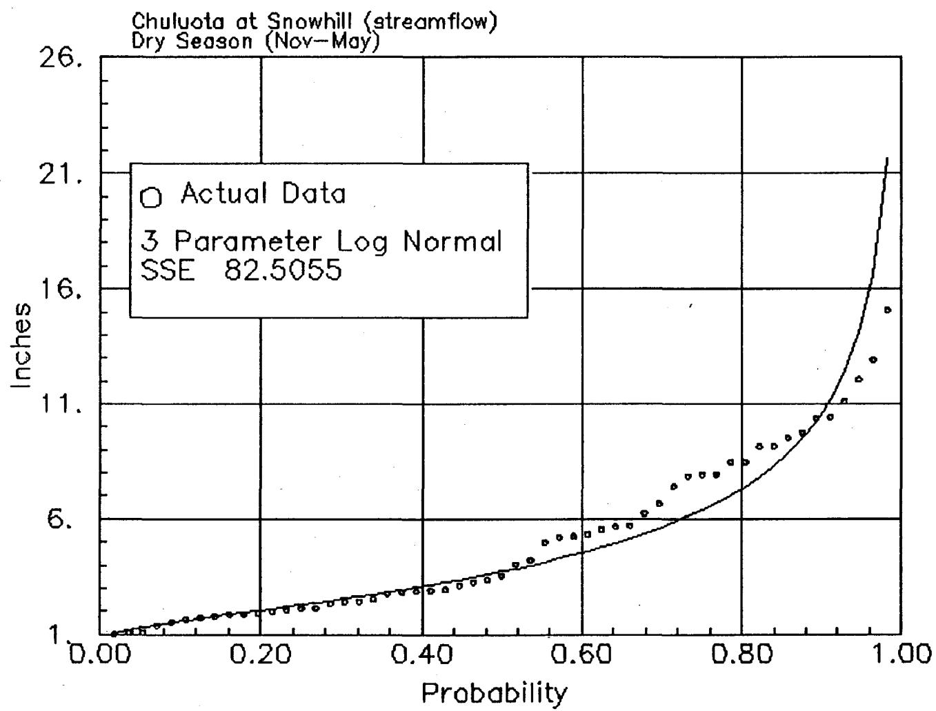
Figure H.1.3 Chuluota at Snowhill, Dry Season streamflow distribution for the years of (1936–1990)
