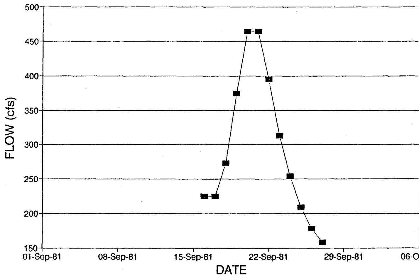
Figure E.1.1 Hydrograph For Estimating Attenuation at Chuluota (September 1981)
