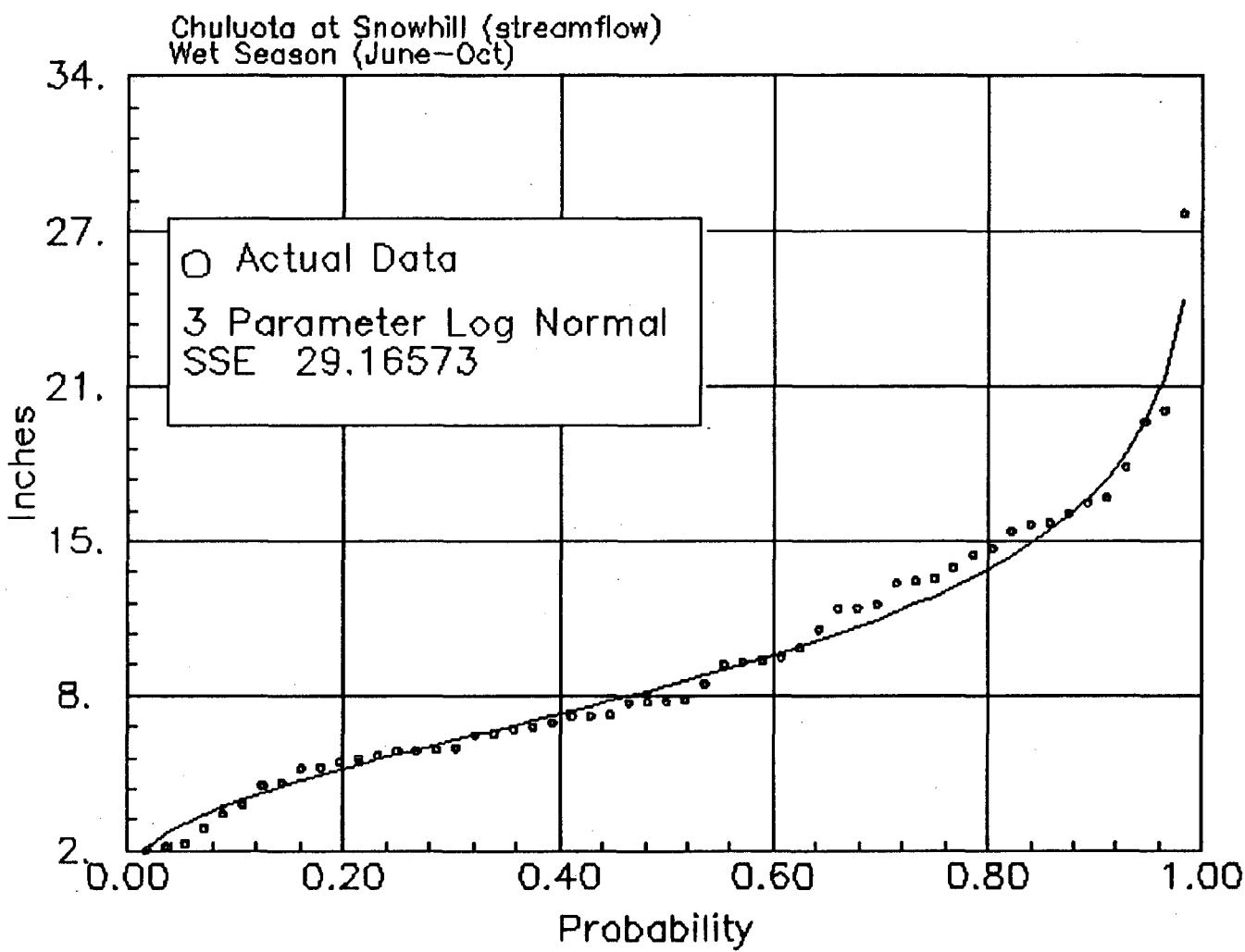
Figure G.1.3 Chuluota at Snowhill, Wet Season streamflow distribution for the years of (1936–1990)
