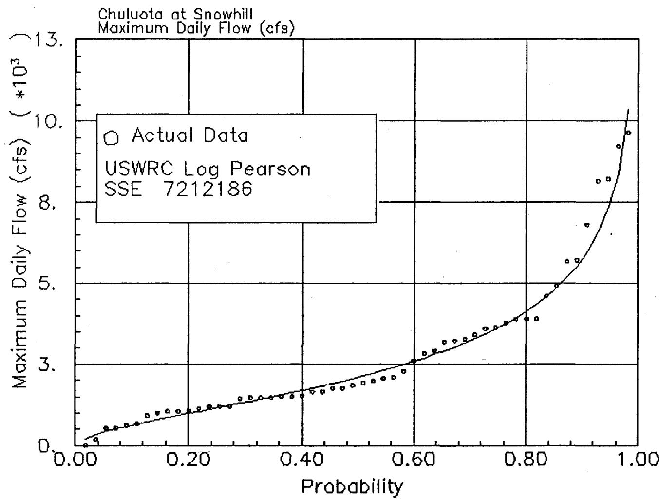
Figure F.1.18 Chuluota at Snowhill, Maximum Daily Flow (cfs) for the Years of 1936–1989.
