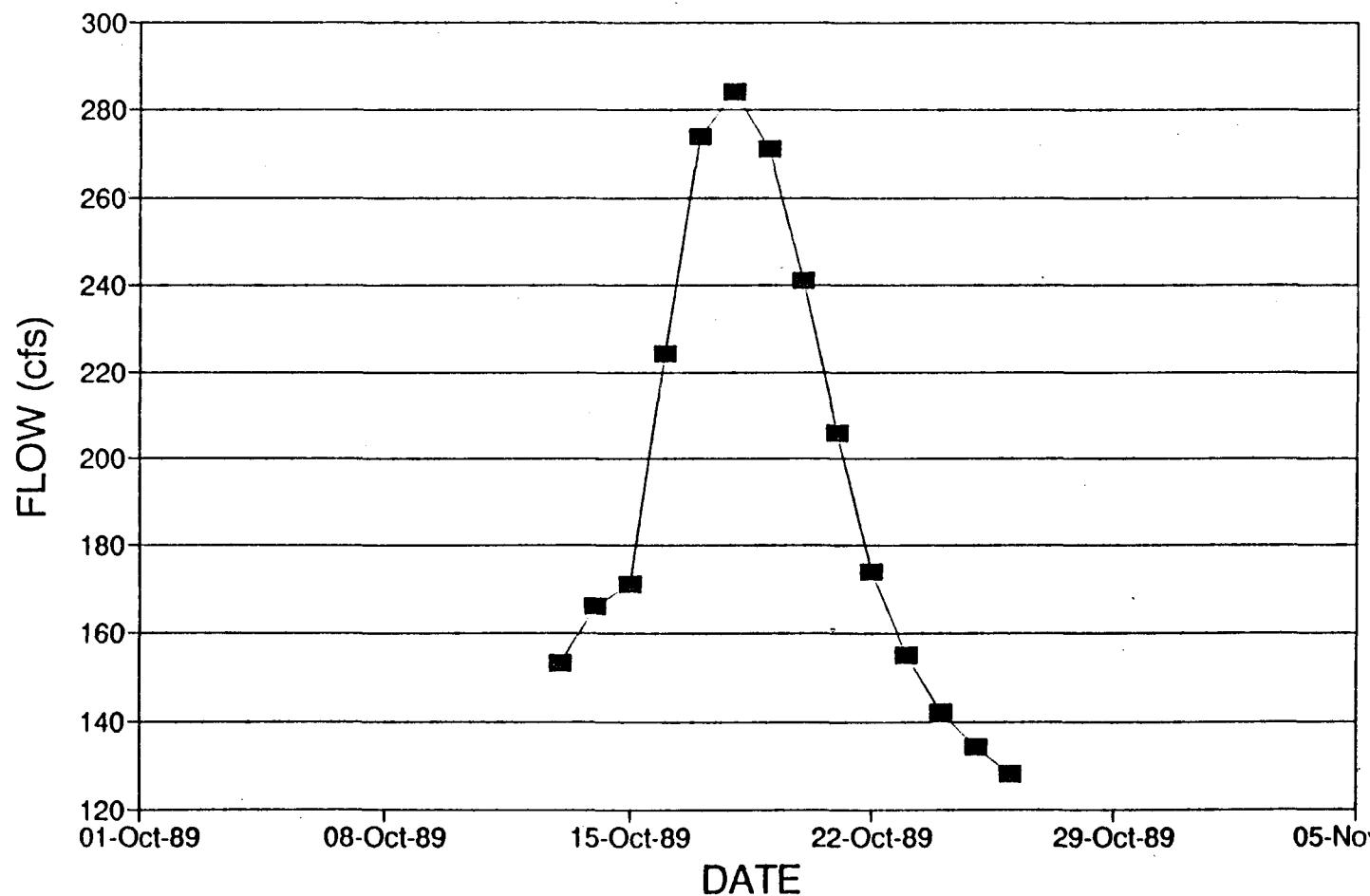
Figure E.1.7 Hydrograph For Estimating Attenuation at Chuluota (October 1989)
