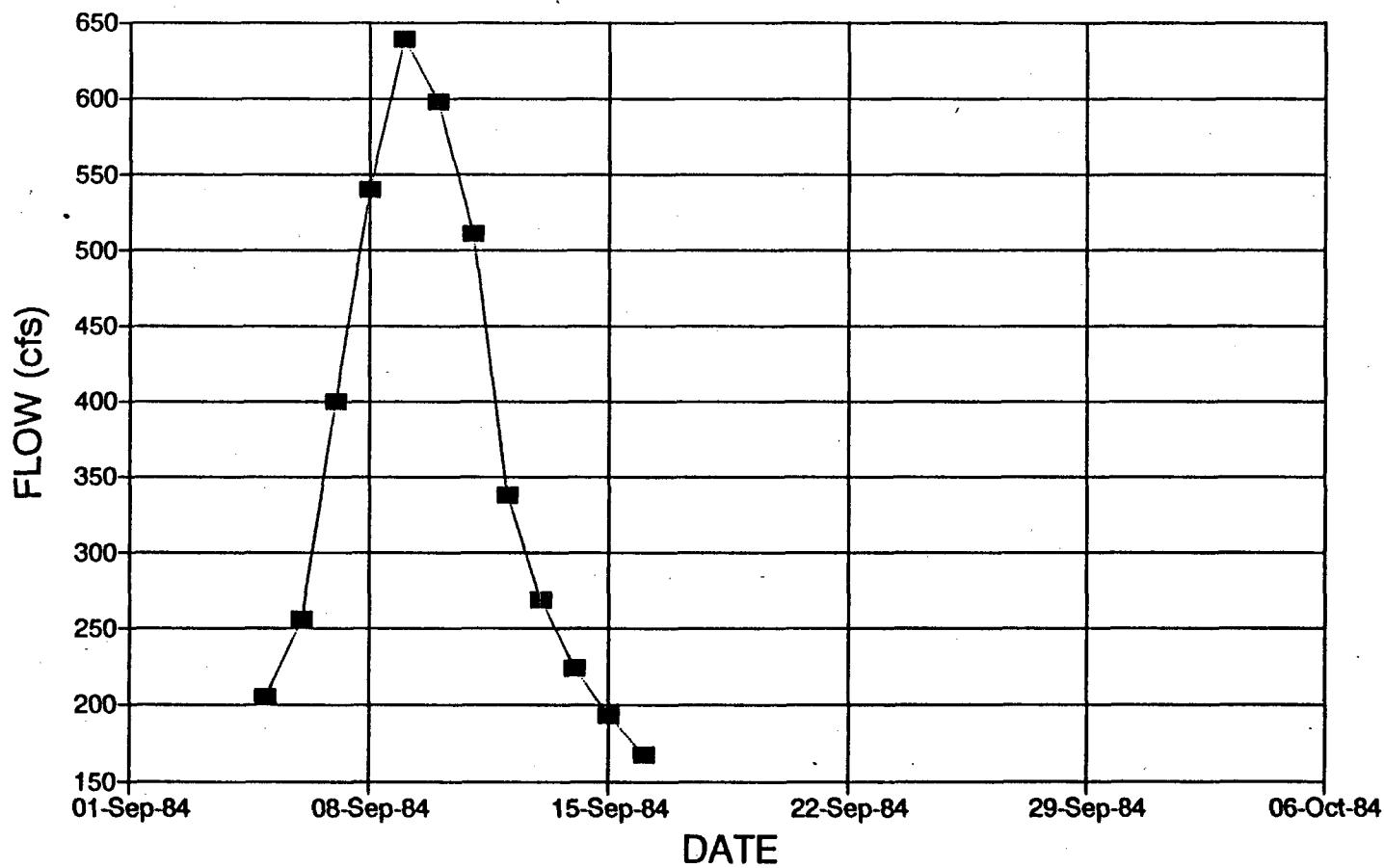
Figure 3.2 Typical Hydrograph Used For Estimating Attenuation at Chuluota
