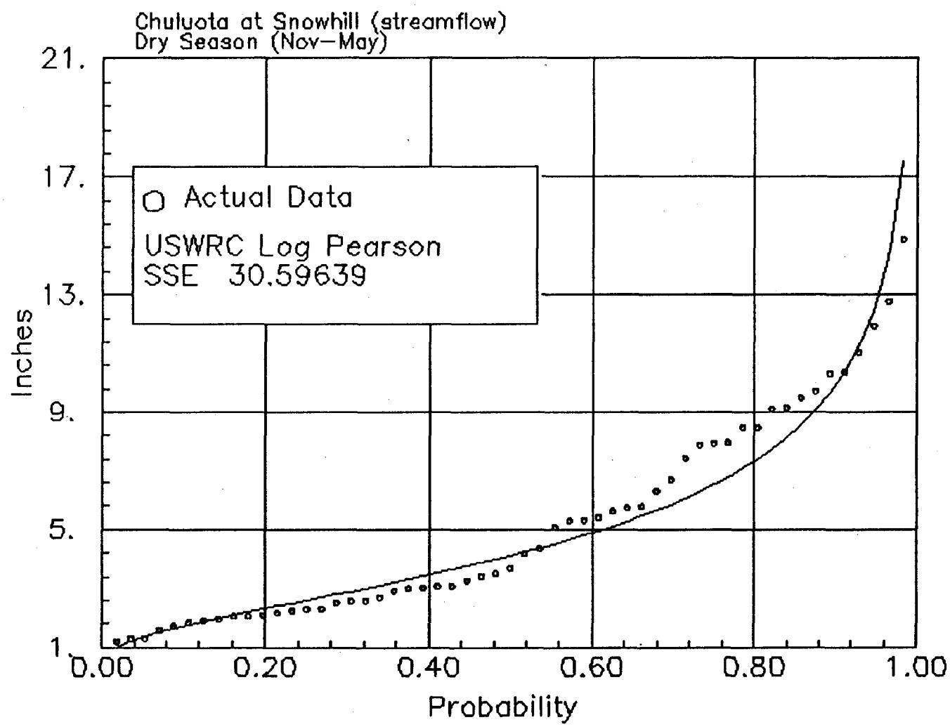
Figure H.1.6 Chuluota at Snowhill, Dry Season streamflow distribution for the years of (1936–1990)
