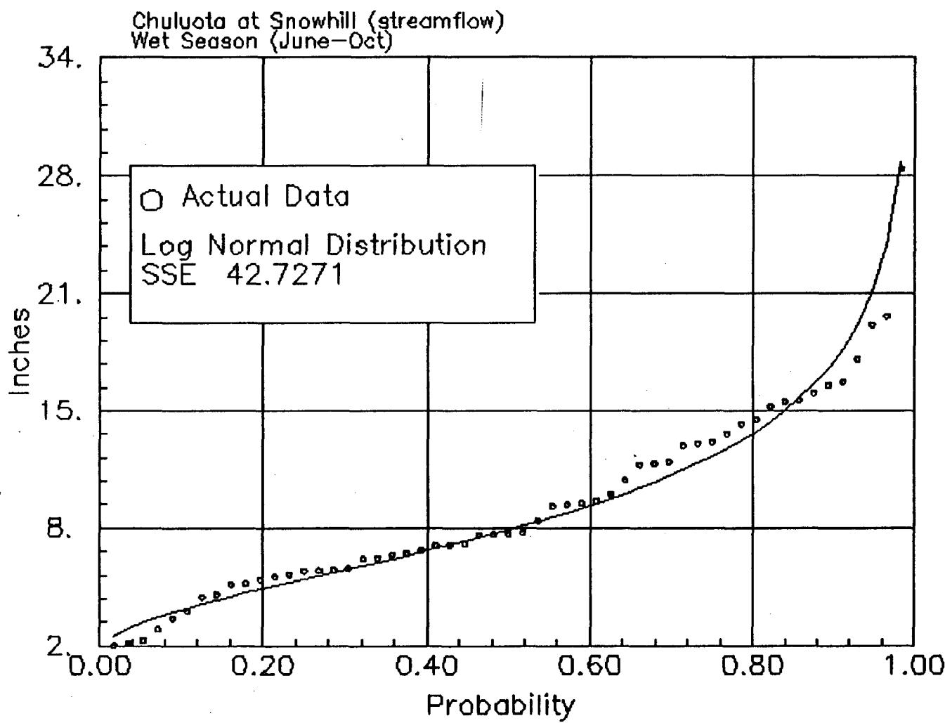
Figure G.1.2 Chuluota at Snowhill, Wet Season streamflow distribution for the years of (1936–1990)
