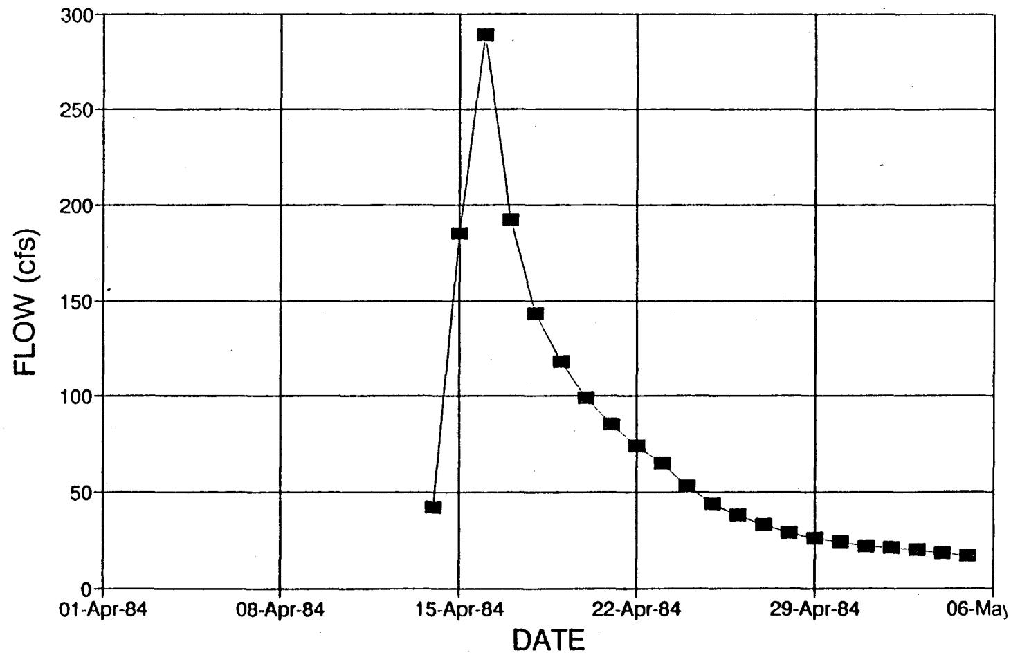
Figure E.3.2 Hydrograph For Estimating Attenuation at Union Park (April 1984)
