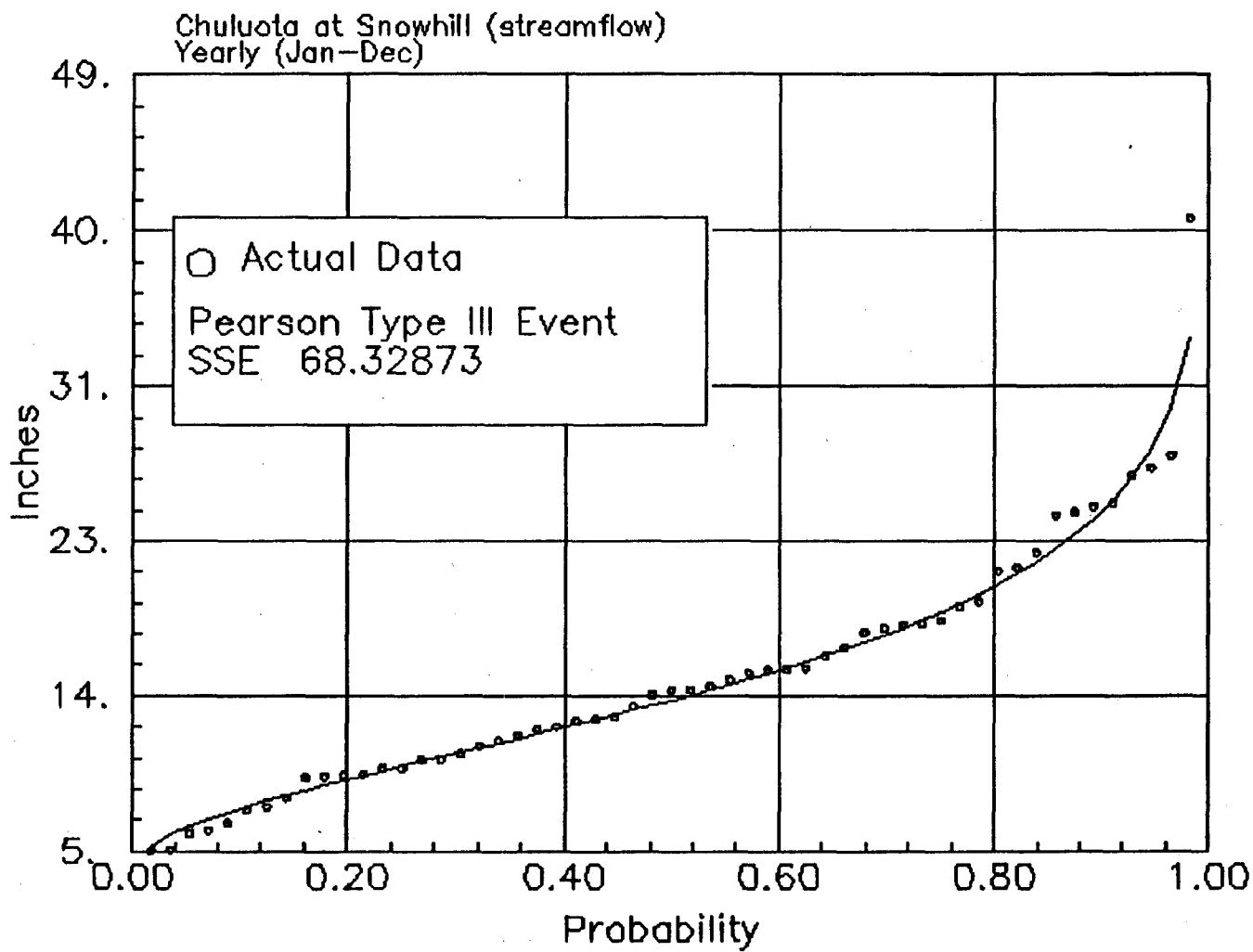
Figure F.1.5 Chuluota at Snowhill, Yearly streamflow distribution for the years of (1936–1990)
