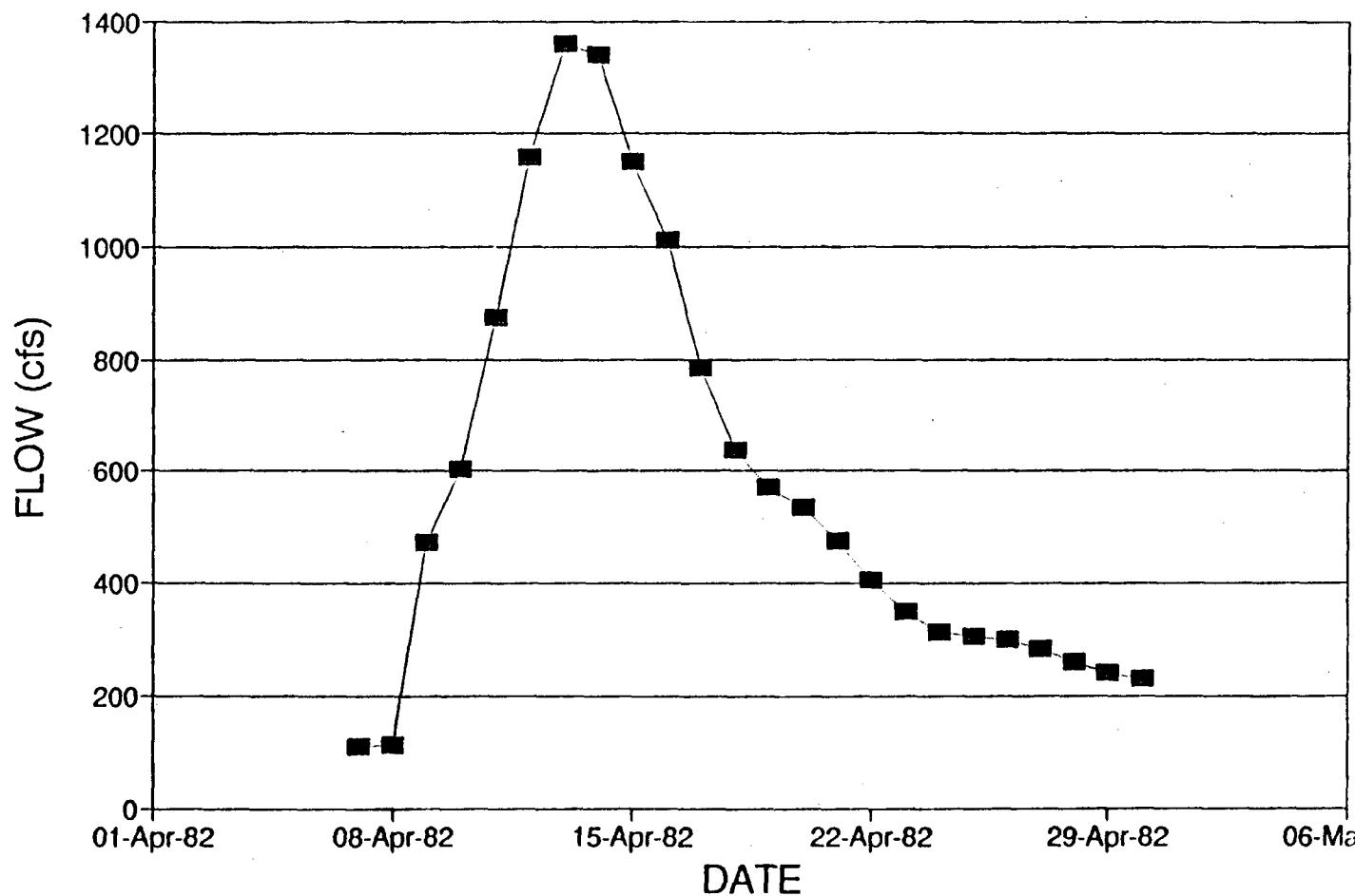
Figure E.1.2 Hydrograph For Estimating Attenuation at Chuluota (April 1982)
