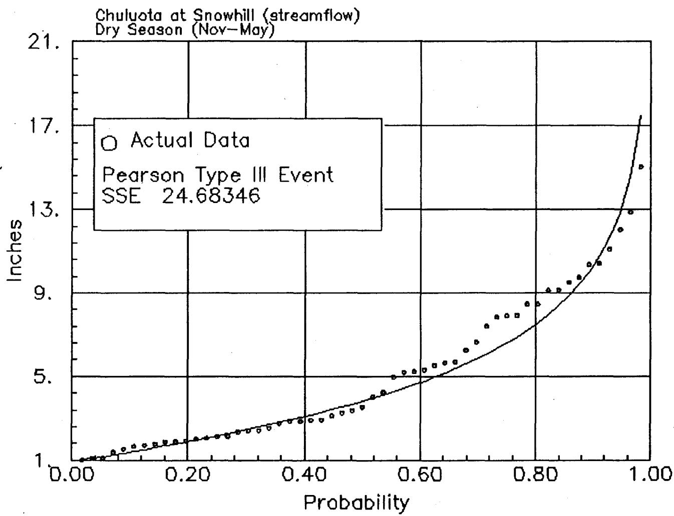
Figure H.1.5 Chuluota at Snowhill, Dry Season streamflow distribution for the years of (1936-1990)
