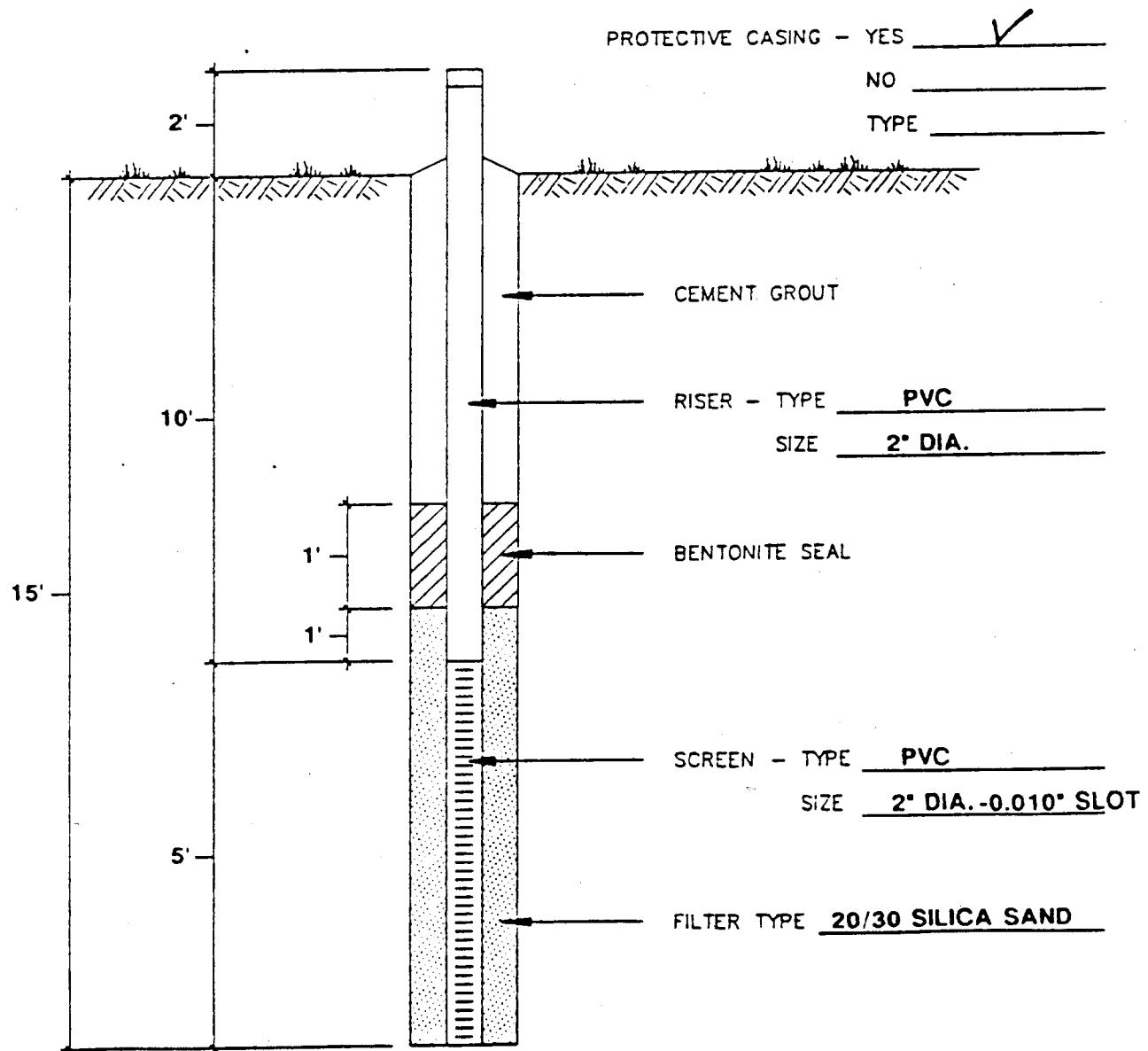
Figure 4.2 Well Completion Diagram - Site MW-5
