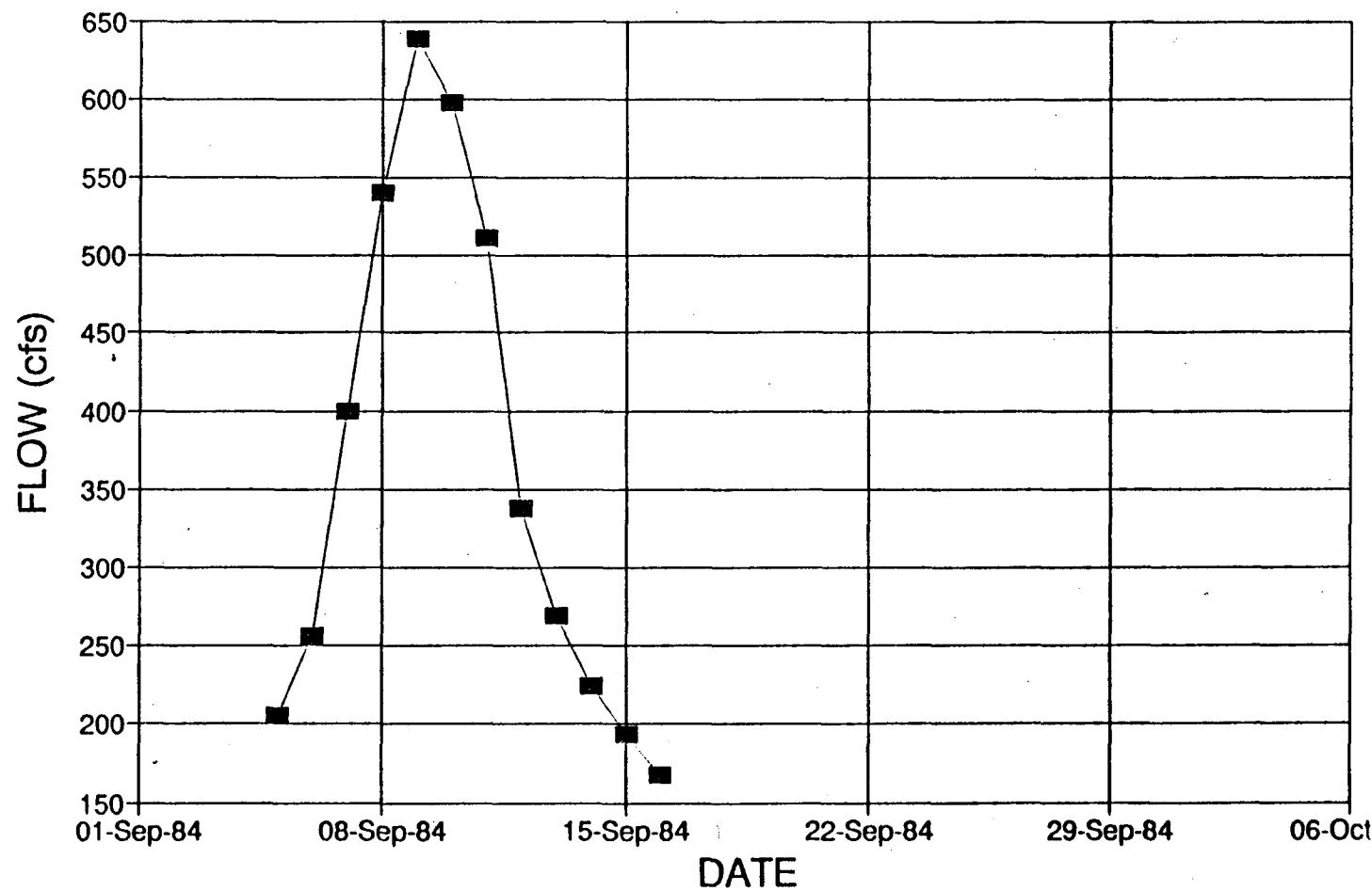
Figure E.1.5 Hydrograph For Estimating Attenuation at Chuluota (September 1984)
