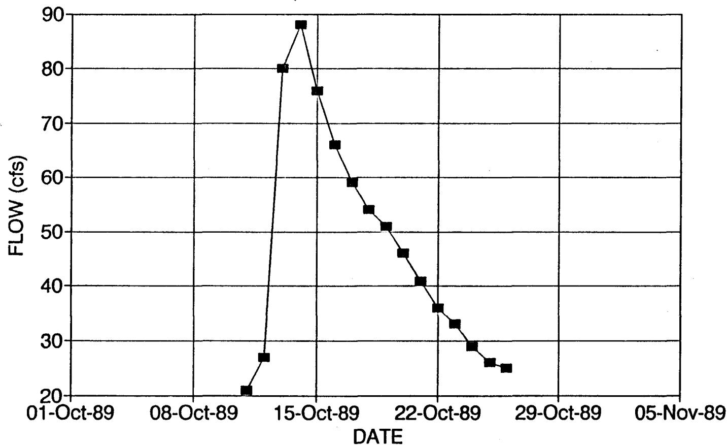
Figure 3.3 Typical Hydrograph Used For Estimating Attenuation at Magnolia Ranch
