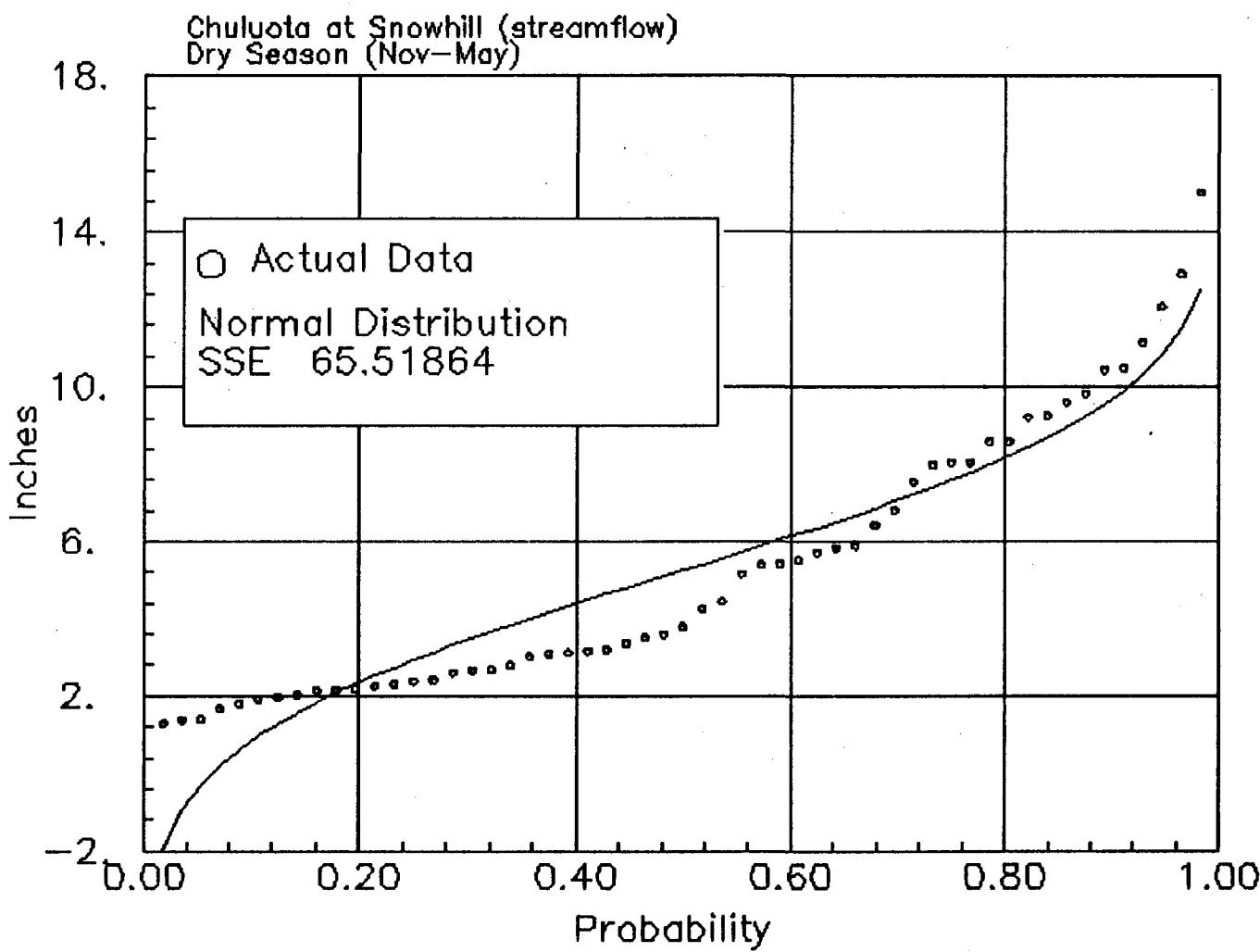
Figure H.1.1 Chuluota at Snowhill, Dry Season streamflow distribution for the years of (1936–1990)
