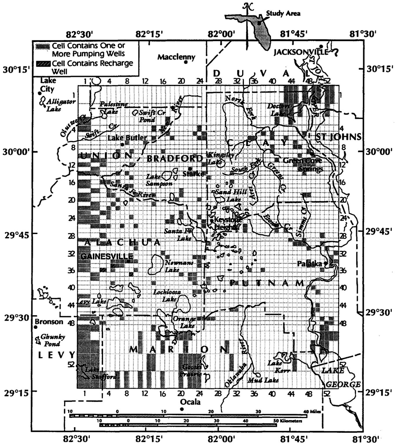
Figure 9-6. Pumping Wells (All Categories) and Recharge Wells in Layer Three in the May 1985 Simulation
