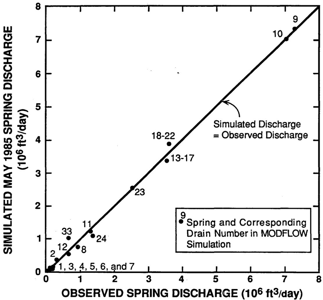
Figure 9-9. Simulated Versus Observed Spring Discharge in the May 1985 Simulation
