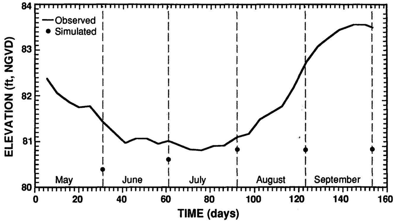
Figure 9-19. Observed and Simulated Water Levels for May-September 1985 for USGS Well at Keystone Heights
