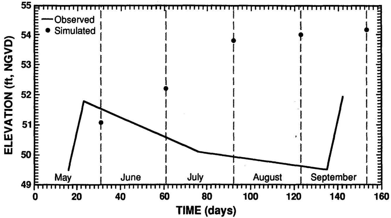
Figure 9-18. Observed and Simulated Water Levels for May-September 1985 for Sperry Rand Well at Gainesville
