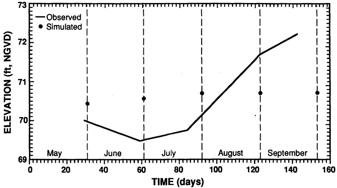
Figure 9-17. Observed and Simulated Water Levels for May-September 1985 for Well A-0005
