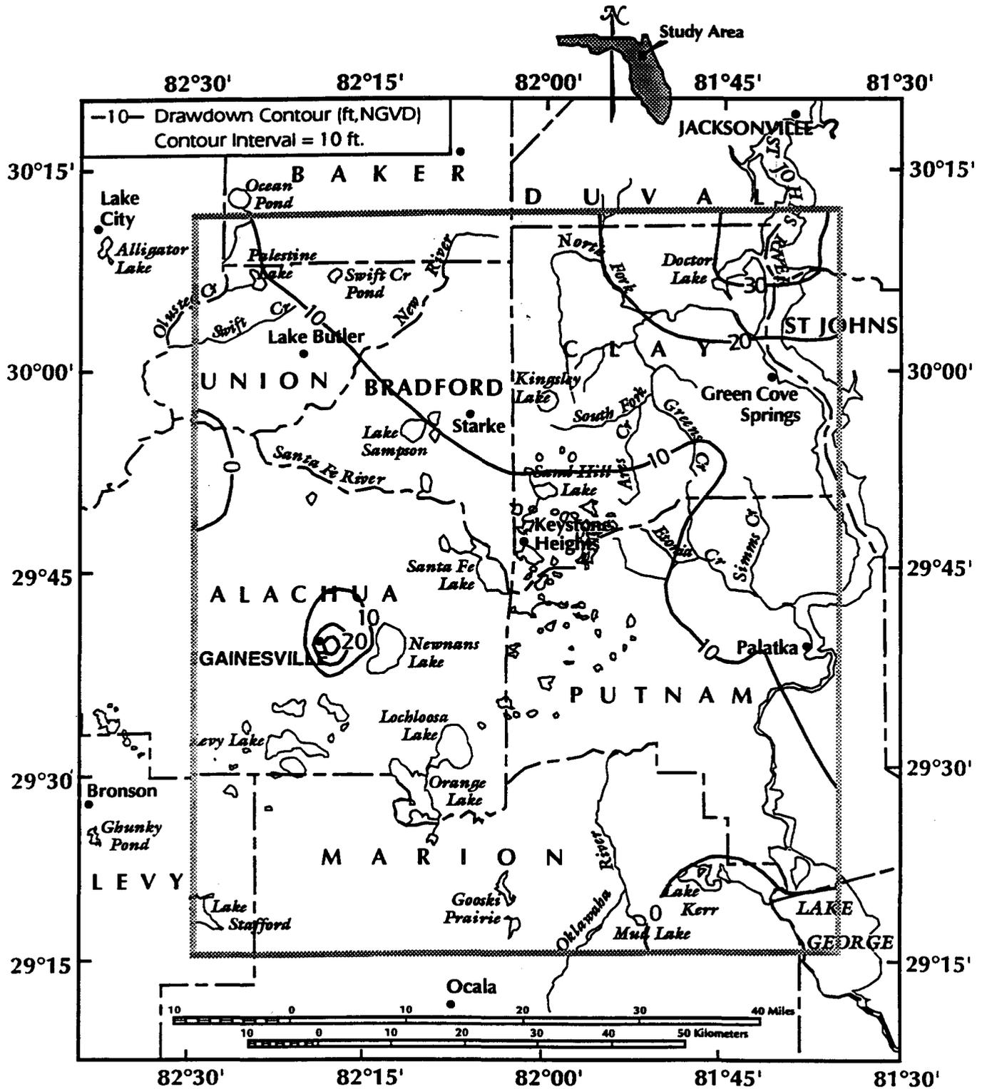
Figure 9-13. Difference Between the Modified Predevelopment and Calculated May 1985 Potentiometric Surfaces (Calculated Drawdowns)
