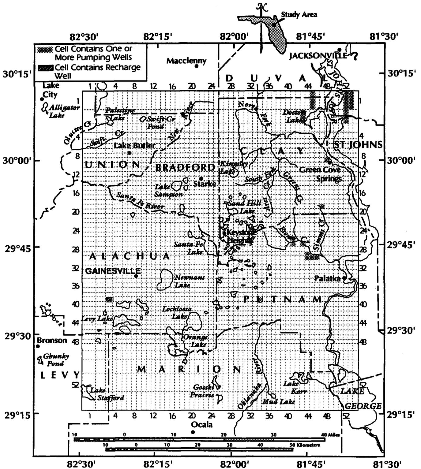
Figure 9-7. Pumping Wells (All Categories) and Recharge Well in Layer Four in the May 1985 Simulation
