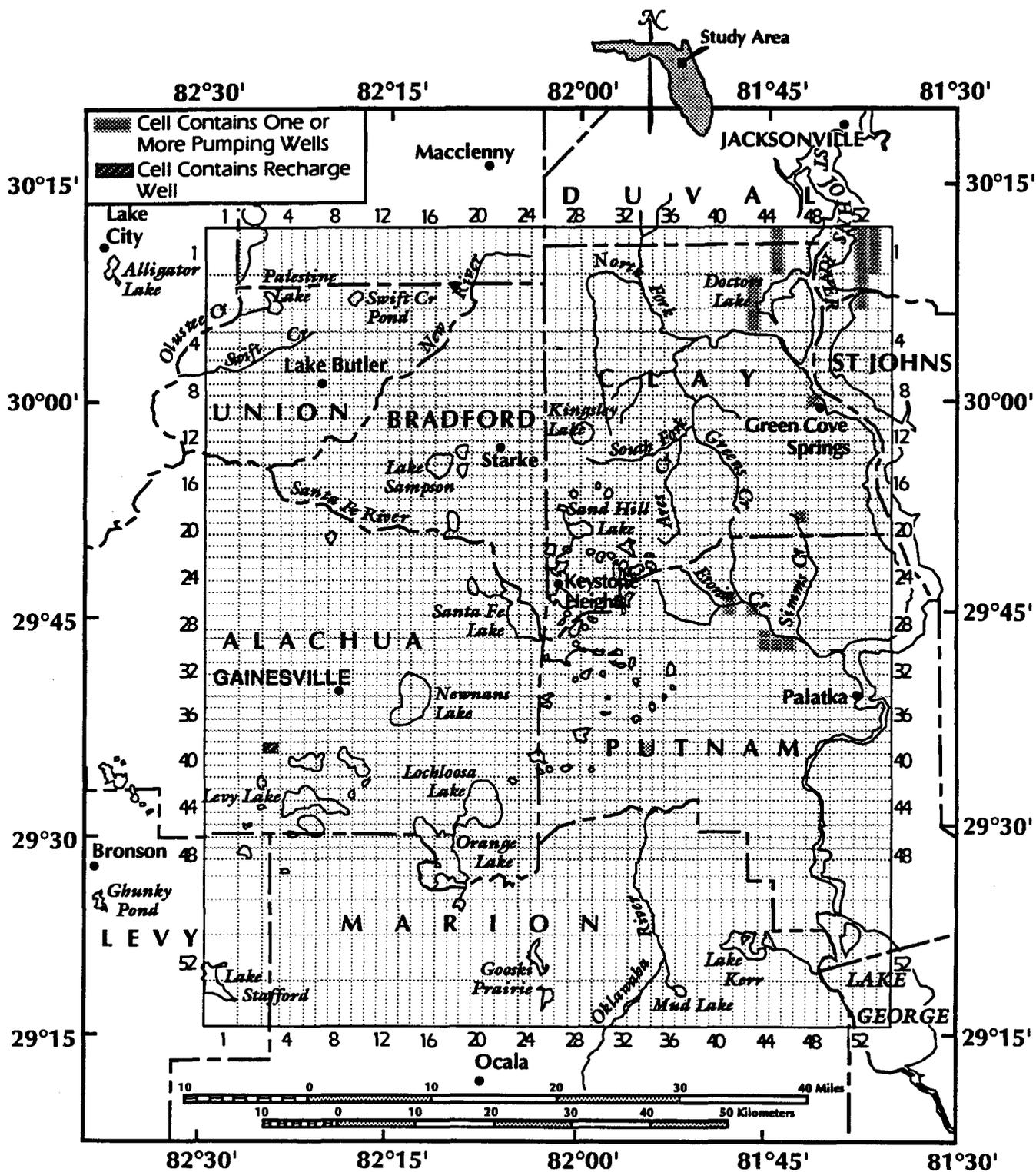
Figure 10-7. Pumping Wells (All Categories) and Recharge Wells in Layer Four in the May 2010 Simulation
