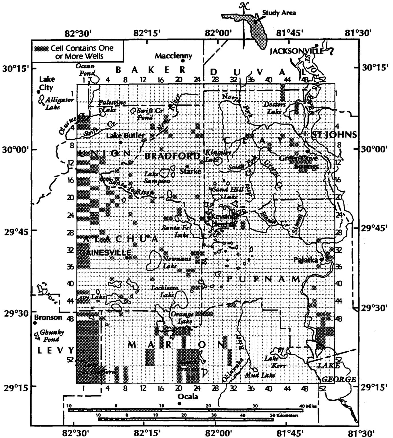
Figure 10-3. Agricultural Wells in Layers Three and Four in the May 2010 Simulation
