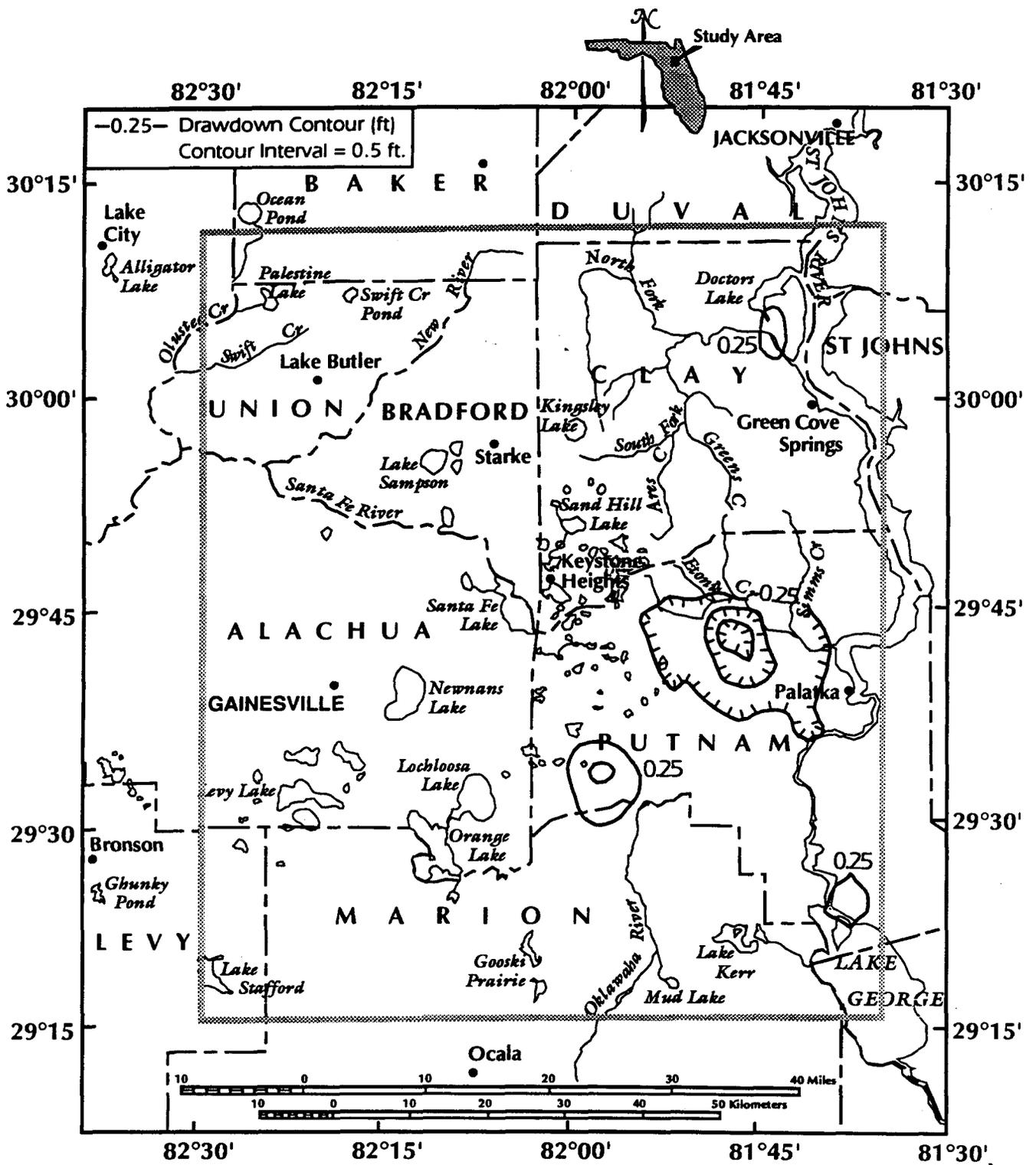
Figure 10-10. Predicted Drawdowns in the Water Table in the Surficial Aquifer Due to Changes in Pumping from May 1985 to May 2010
