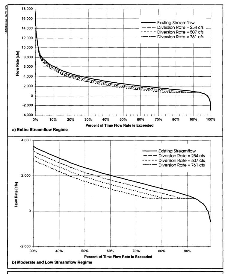
Figure 14. Maximum Effect of Water Supply Withdrawal on Flow Duration Curve for the St. Johns River at De Land, Florida.
