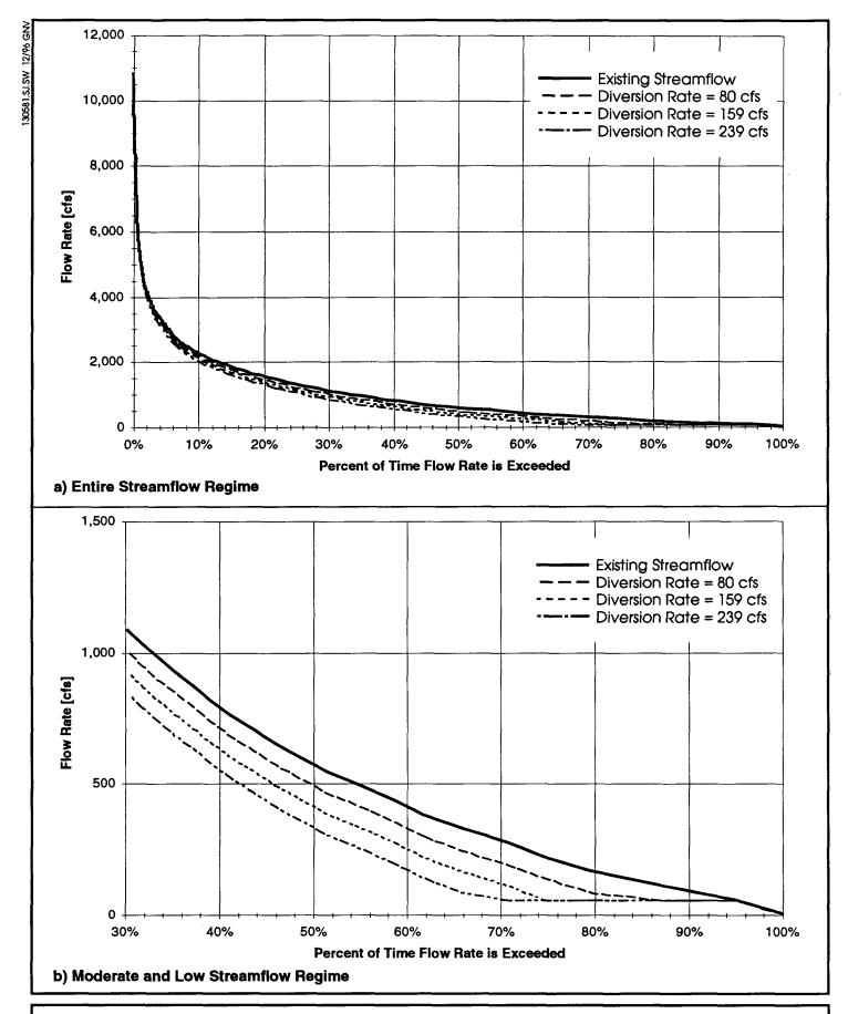
Figure 11. Maximum Effect of Water Supply Withdrawal on Flow Duration Curve for the St. Johns River near Cocoa, Florida.
