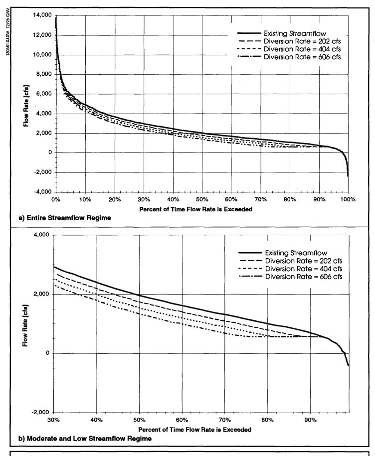
Figure 13. Maximum Effect of Water Supply Withdrawal on Flow Duration Curve for the St. Johns River at Sanford, Florida.
