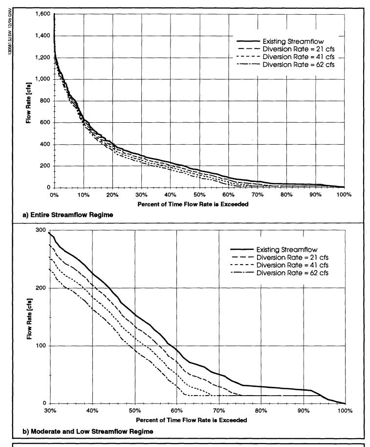
Figure 10. Maximum Effect of Water Supply Withdrawal on Flow Duration Curve for Haines Creek at Lisbon, Florida.
