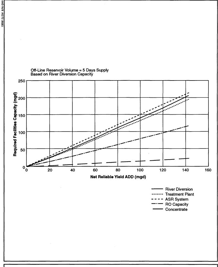
Figure 24. Surface Water Facility Requirements for St. Johns River near Titusville.
