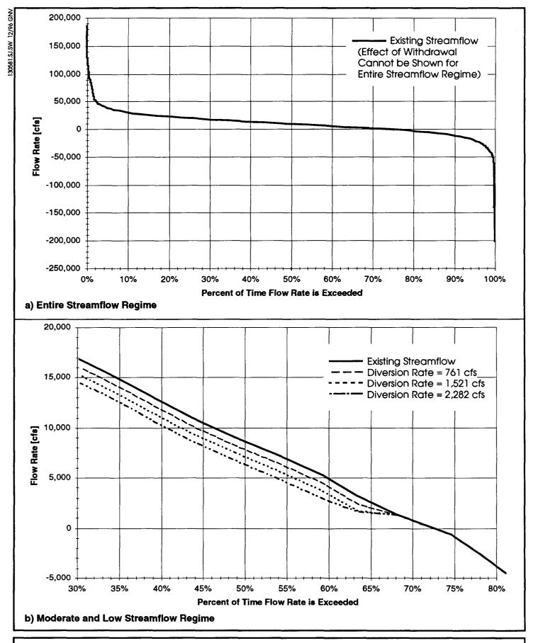
Figure 15. Maximum Effect of Water Supply Withdrawal on Flow Duration Curve for the St. Johns River above Jacksonville, Florida.
