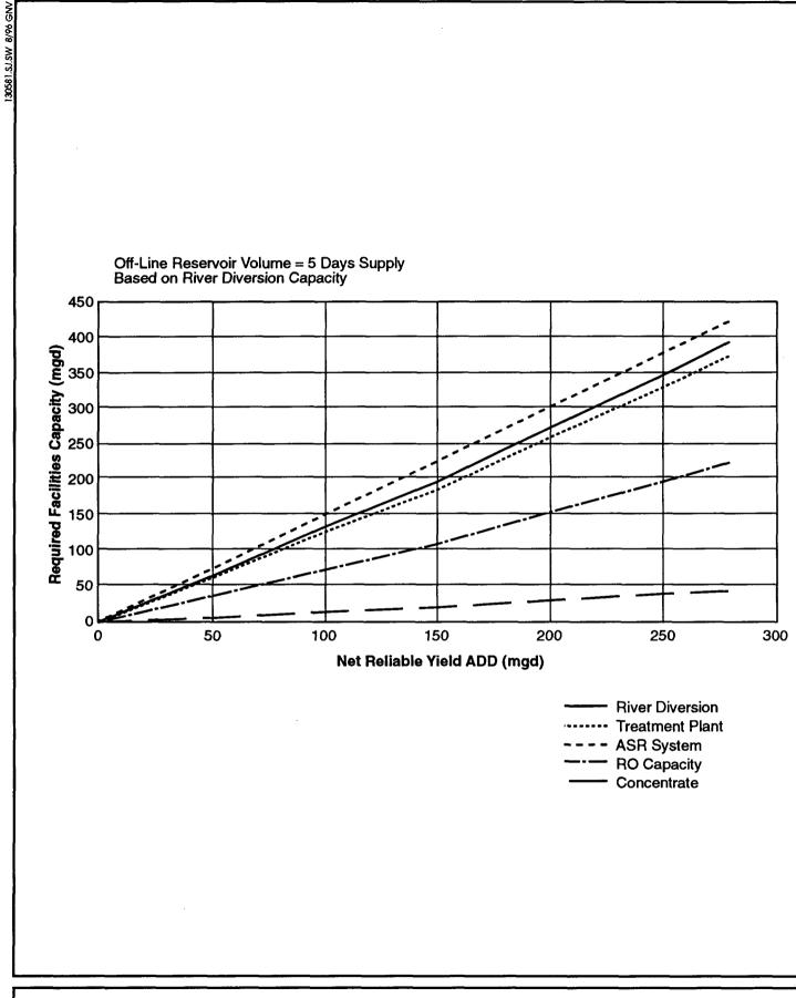
Figure 25. Surface Water Facility Requirements for St. Johns River at Sanford.
