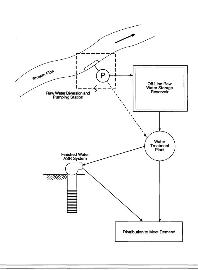
Figure 1. Facilities Required to Develop Reliable Surface Water Supply to Meet Urban Demands.
