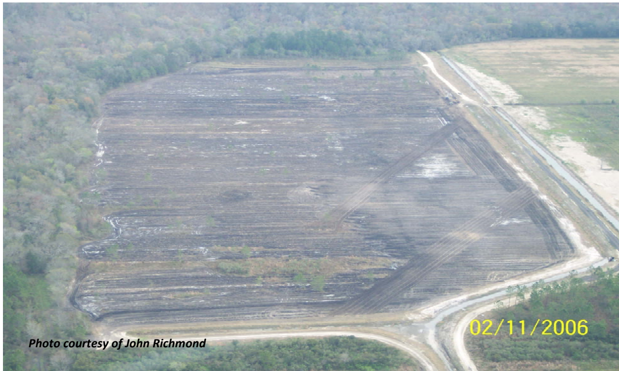
Figure 7. Aerial photo of alum water treatment residual (WTR) application
