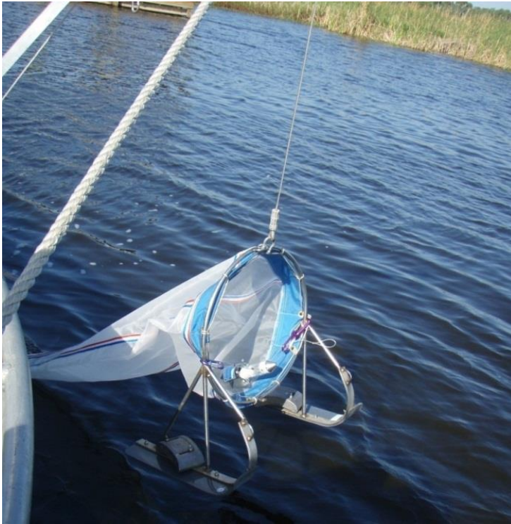
Figure 10. Plankton net (0.5-m diameter, 500-µm mesh) mounted on a towing sled used to collect ichthyoplankton samples from the St. Johns River. A mounted flowmeter is visible in the bottom of the net opening
