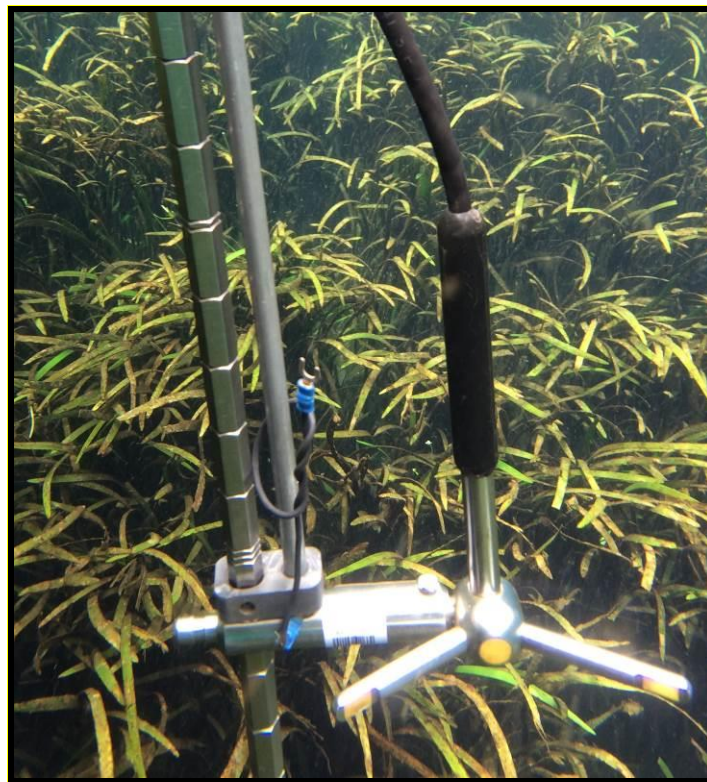
Figure 3 Photo of SonTek Flow Tracker-ADV Unit Used to Collect Point Velocity Measurements above Substrate and Velocity Profiles across the Channel
