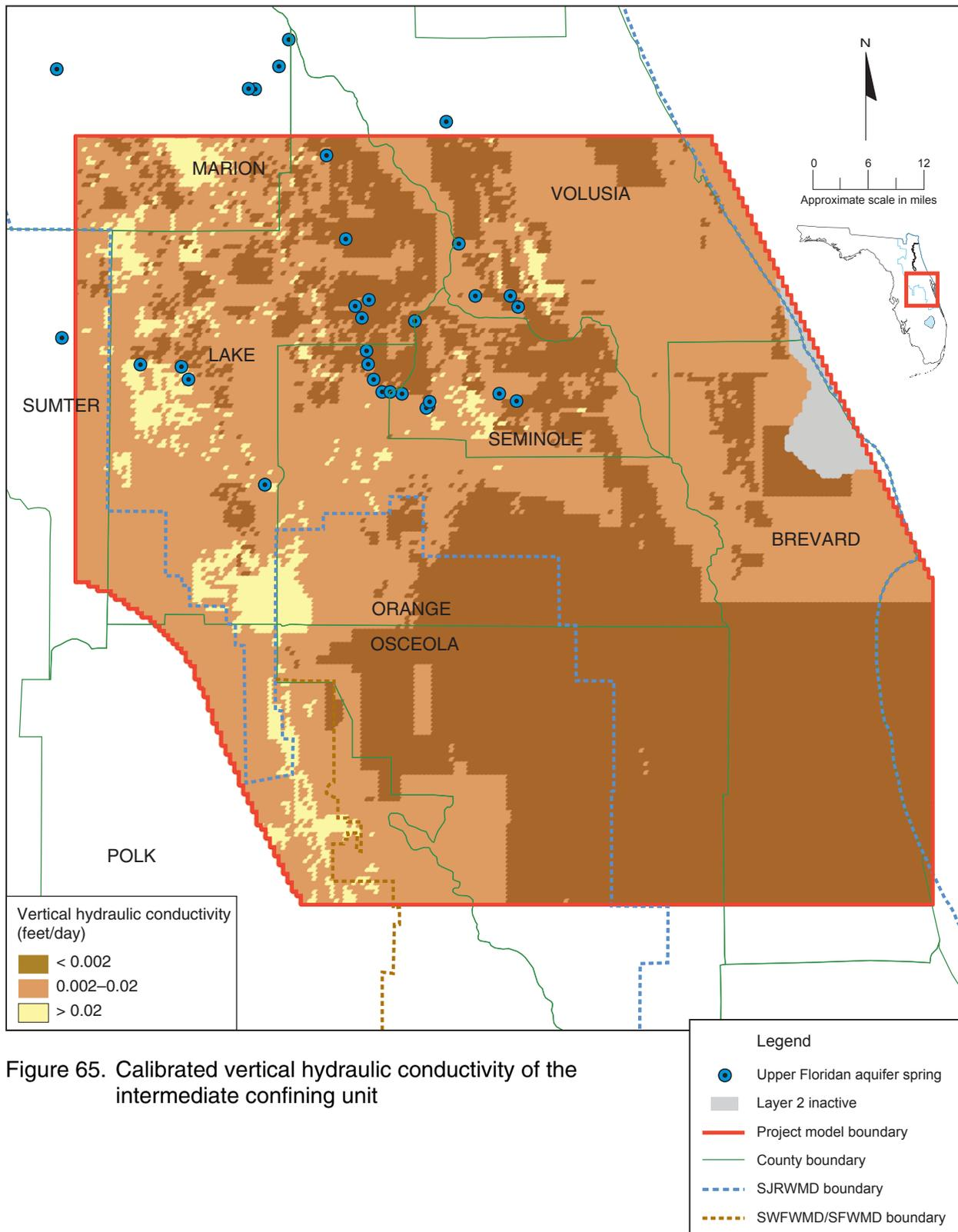
Figure 65. Calibrated vertical hydraulic conductivity of the intermediate confining unit
