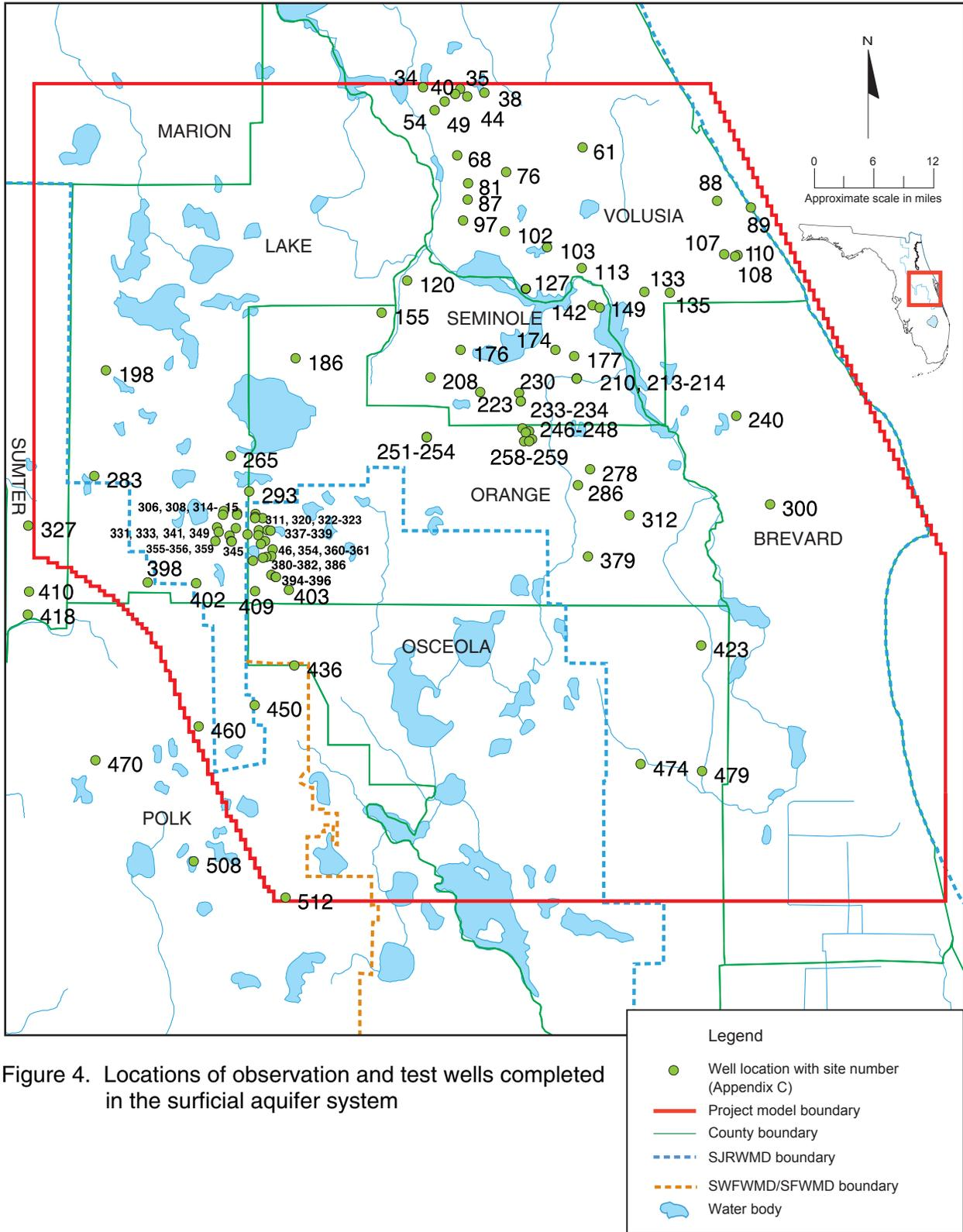
Figure 4. Locations of observation and test wells completed in the surficial aquifer system
