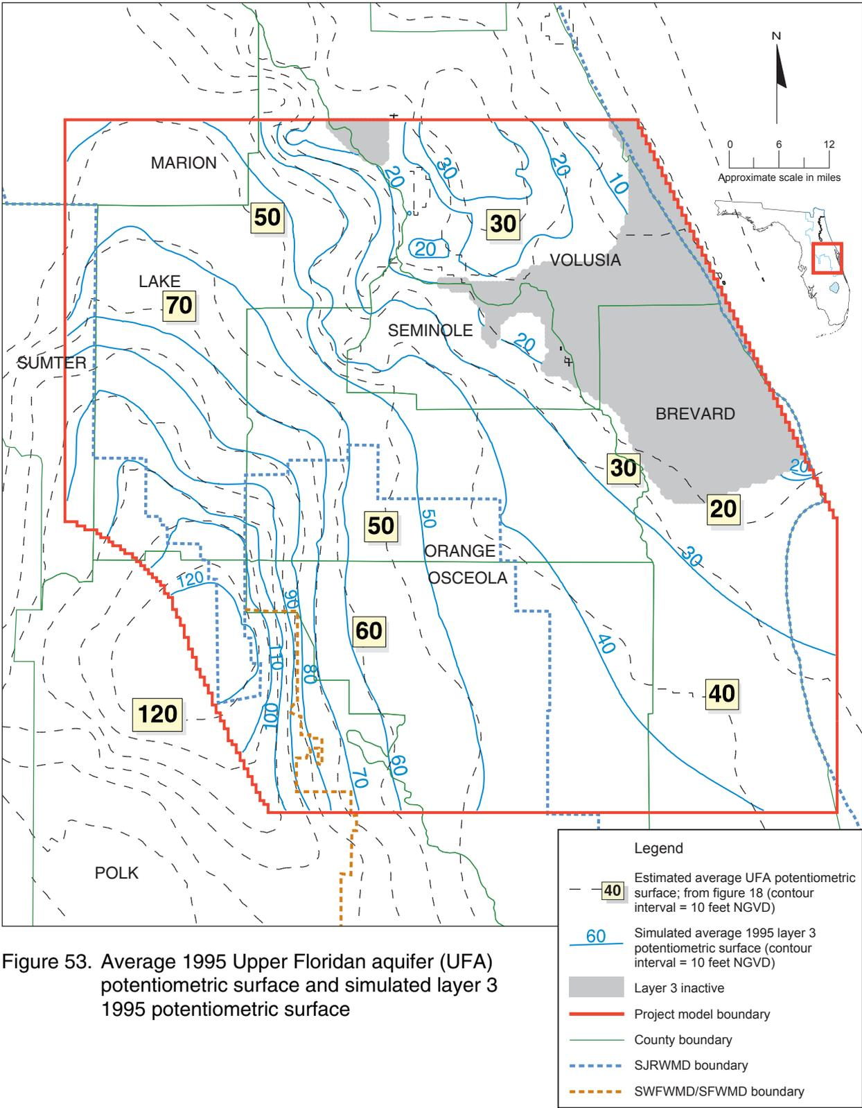
Figure 53. Average 1995 Upper Floridan aquifer (UFA) potentiometric surface and simulated layer 3 1995 potentiometric surface
