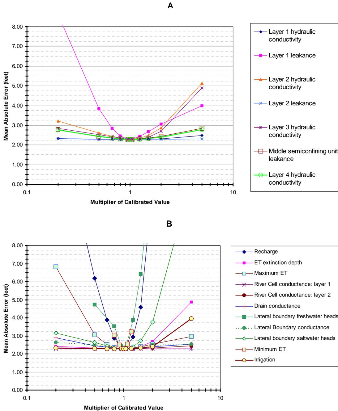
Figure 78. Sensitivity of Upper Floridan aquifer (layer 2) simulated heads to changes in (A) aquifer confining unit parameters and (B) selected boundary conditions
