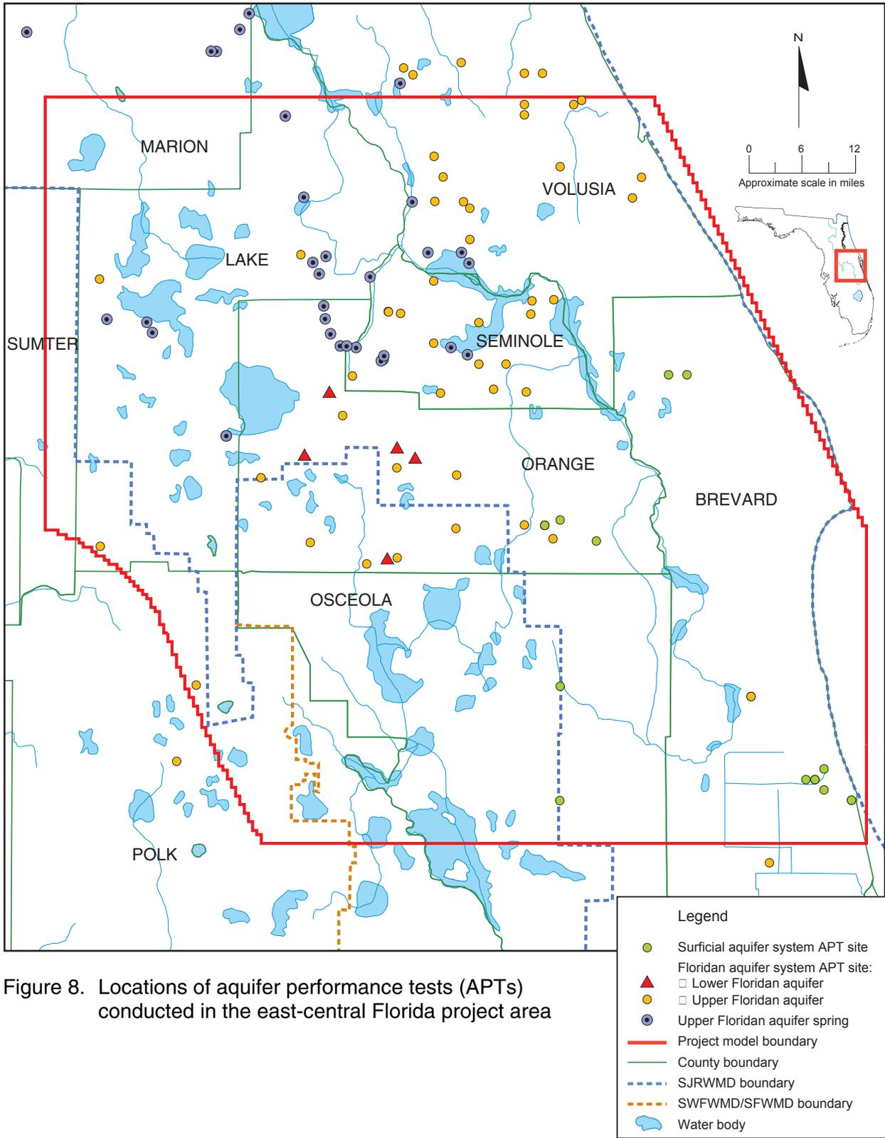
Figure 8. Locations of aquifer performance tests (APTs) conducted in the east-central Florida project area
