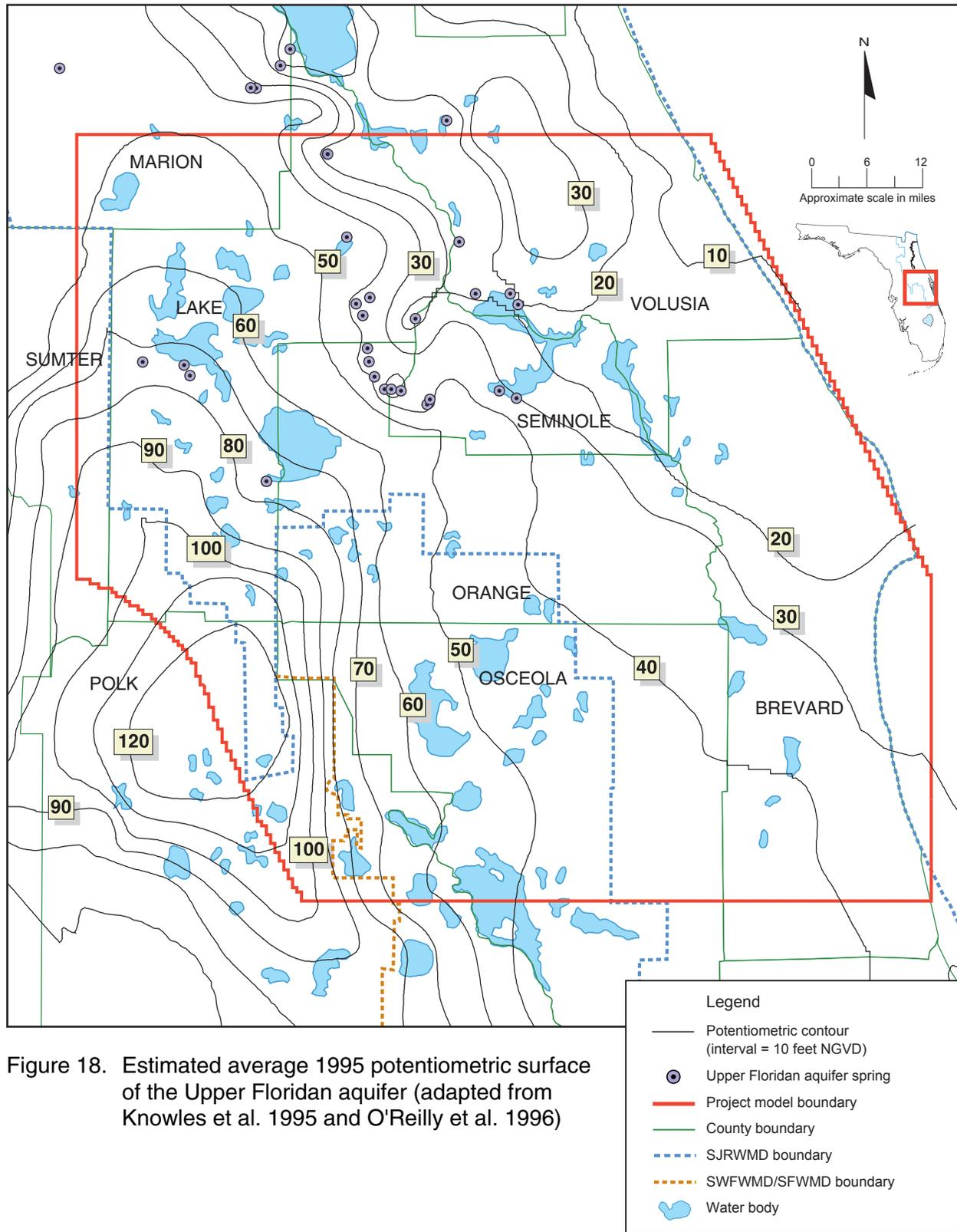
Figure 18. Estimated average 1995 potentiometric surface of the Upper Floridan aquifer (adapted from Knowles et al. 1995 and O'Reilly et al. 1996)
