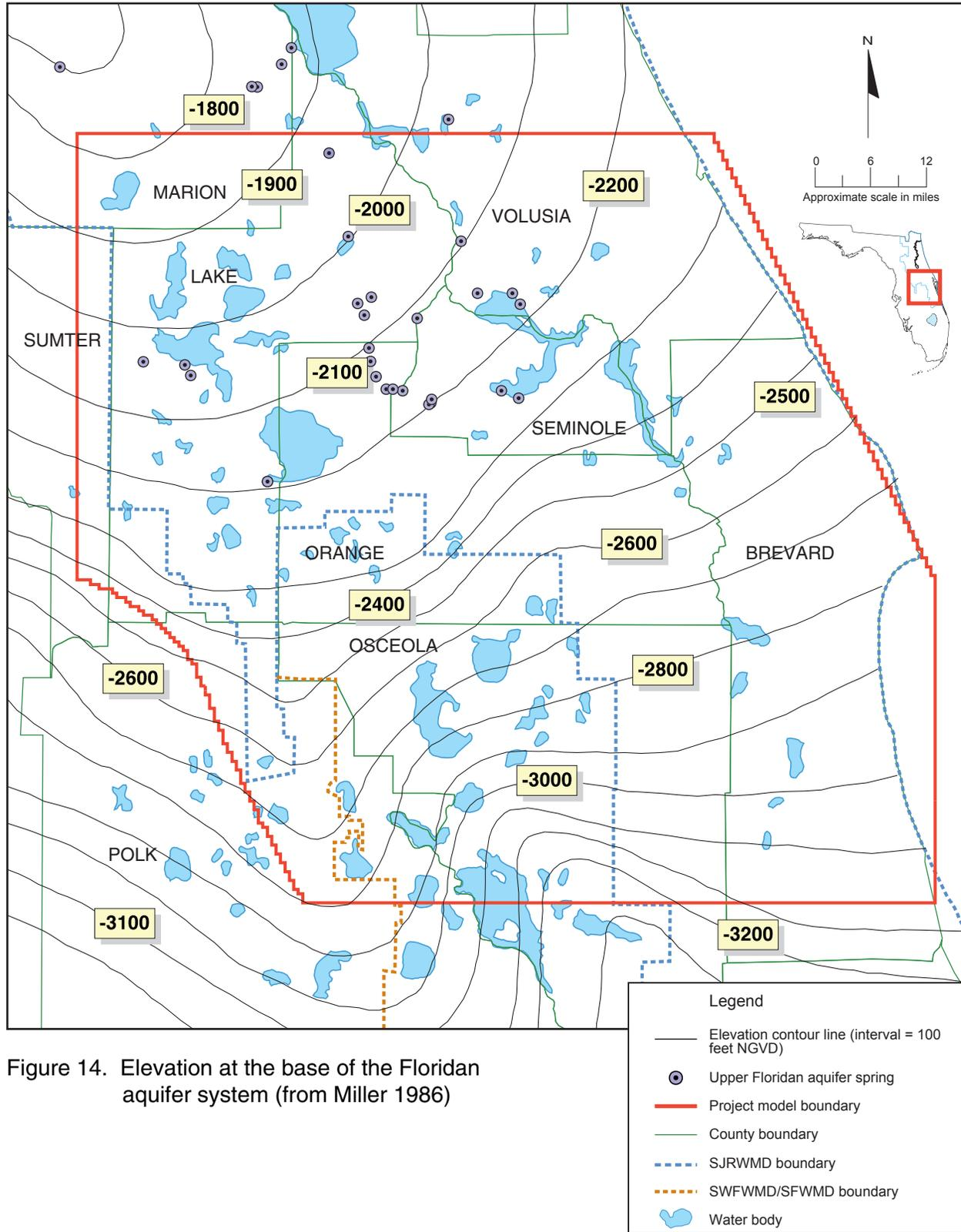
Figure 14. Elevation at the base of the Floridan aquifer system (from Miller 1986)
