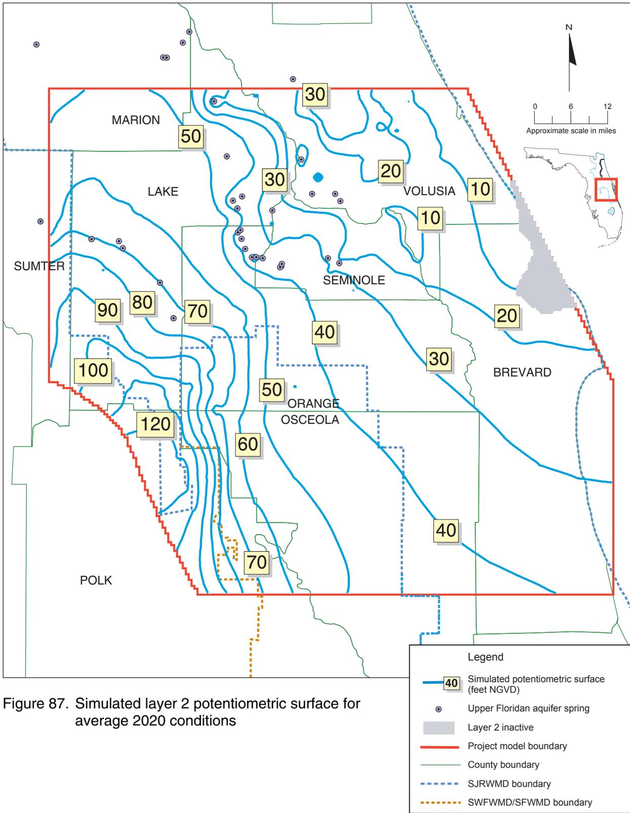
Figure 87. Simulated layer 2 potentiometric surface for average 2020 conditions
