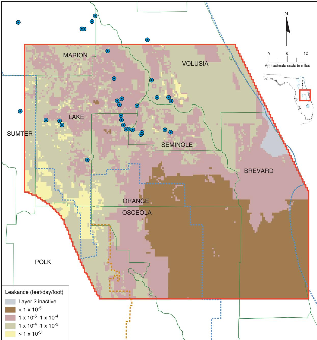
Figure 66. Calibrated leakance of the intermediate confining unit
