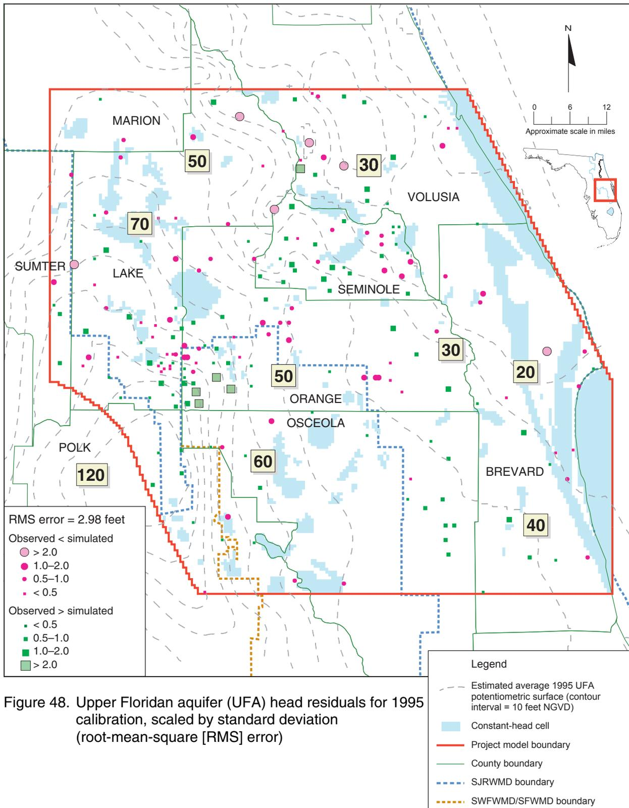
Figure 48. Upper Floridan aquifer (UFA) head residuals for 1995 calibration, scaled by standard deviation (root-mean-square [RMS] error)
