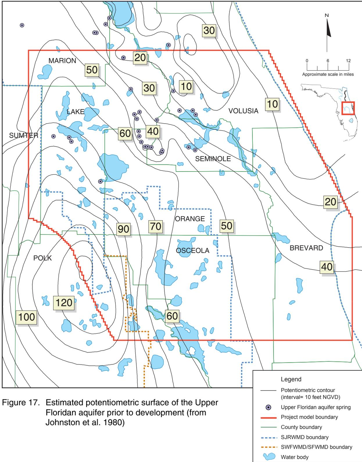
Figure 17. Estimated potentiometric surface of the Upper Floridan aquifer prior to development (from Johnston et al. 1980)
