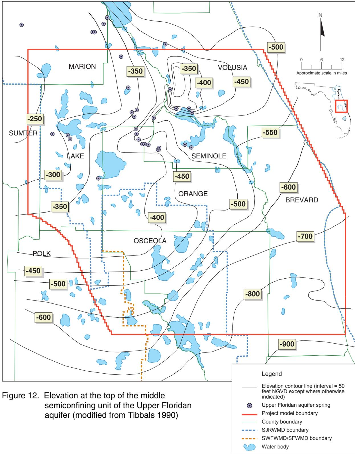
Figure 12. Elevation at the top of the middle semiconfining unit of the Upper Floridan aquifer (modified from Tibbals 1990)
