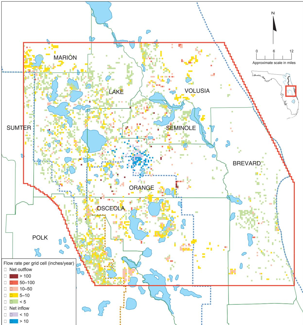
Figure 30. Average 1995 withdrawals applied to model layer 2
