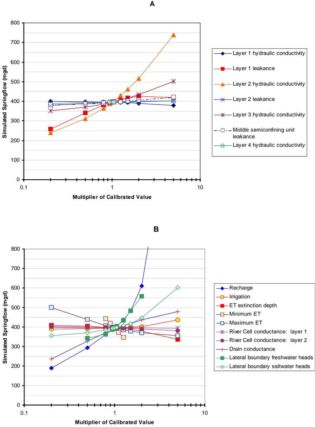
Figure 79. Sensitivity of simulated spring flow to changes in (A) aquifer and confining unit parameters and (B) selected boundary conditions
