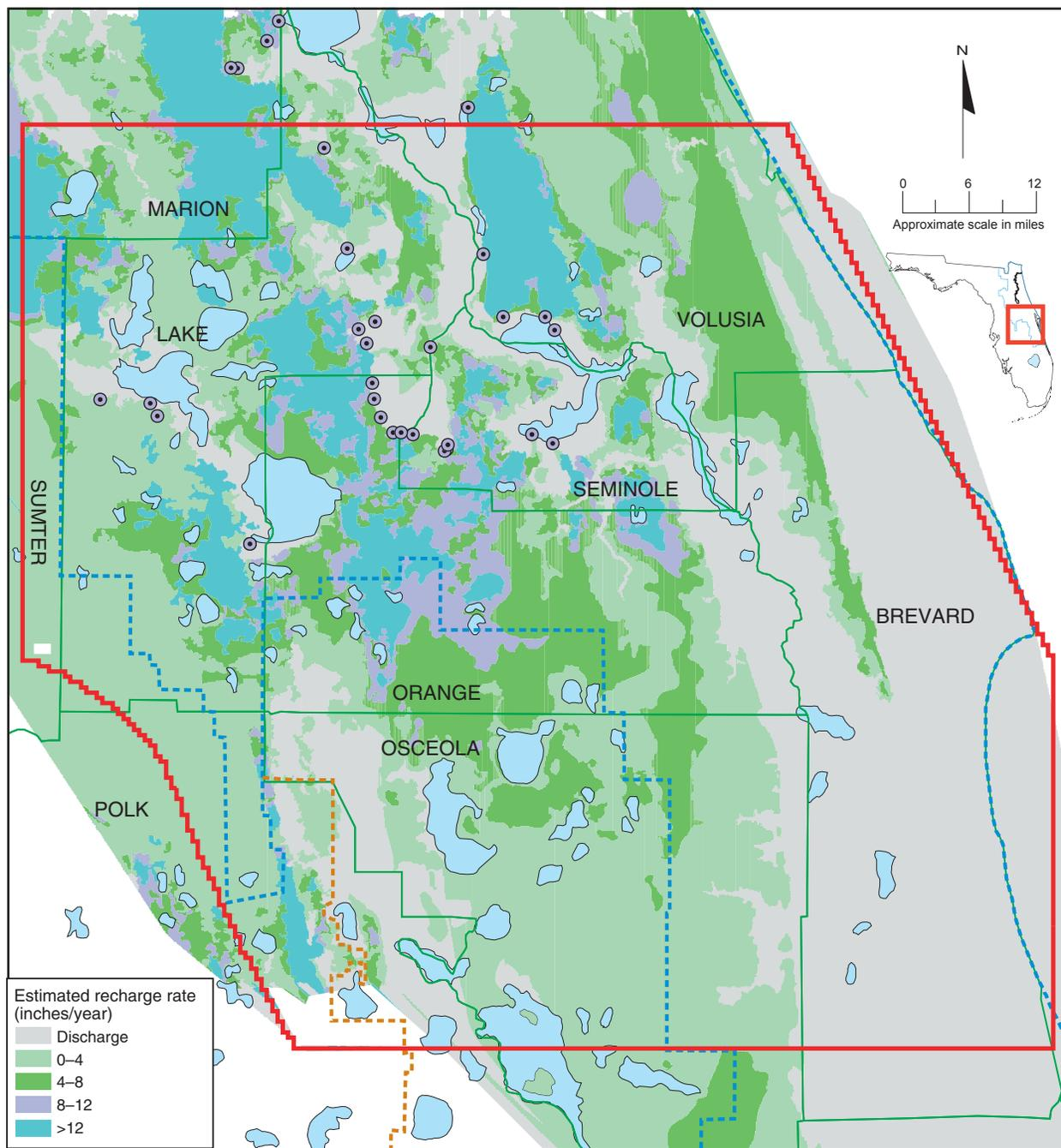
Figure 15. Areas of recharge to and discharge from the Floridan aquifer system (modified from Boniol et al. 1993)
