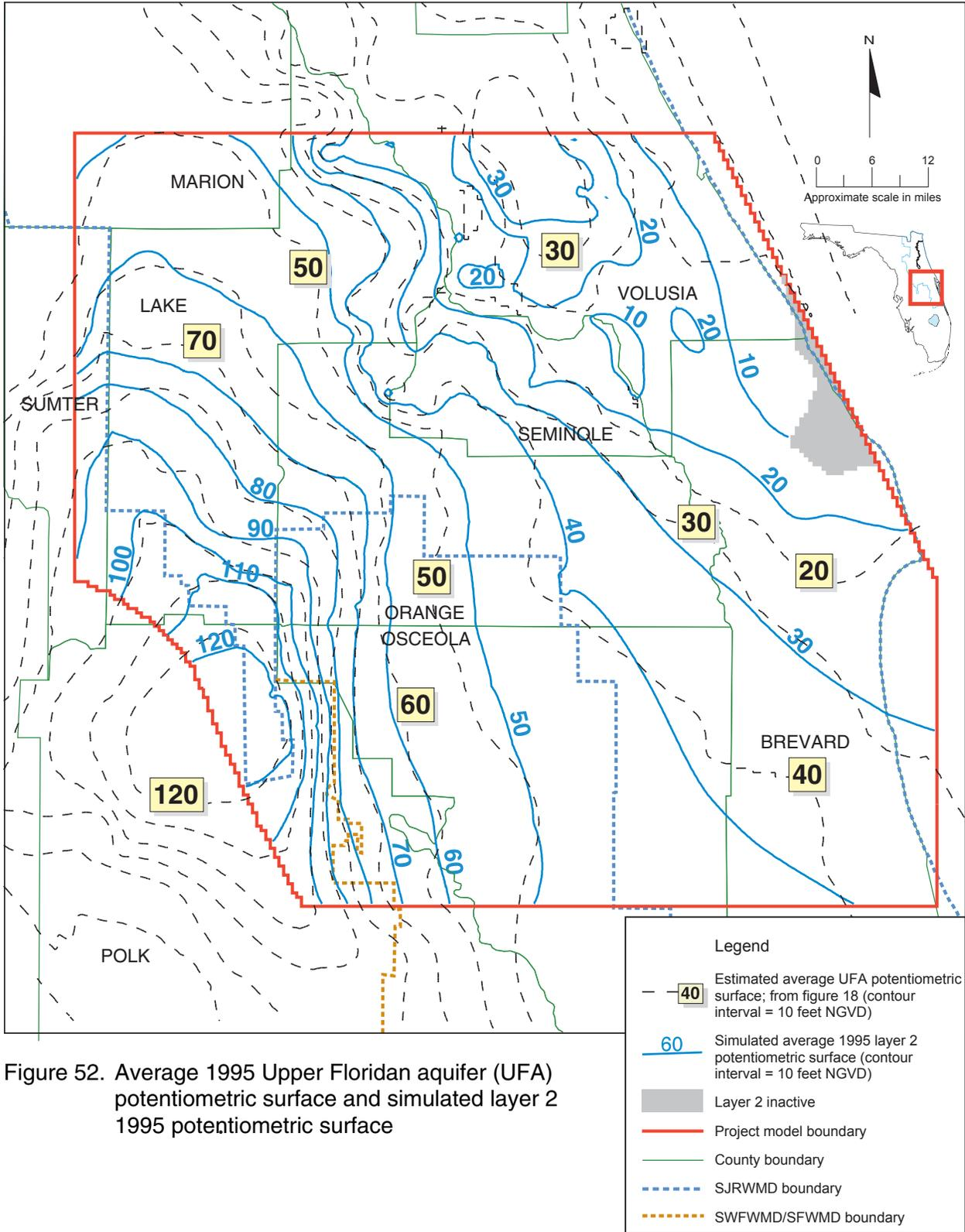
Figure 52. Average 1995 Upper Floridan aquifer (UFA) potentiometric surface and simulated layer 2 1995 potentiometric surface
