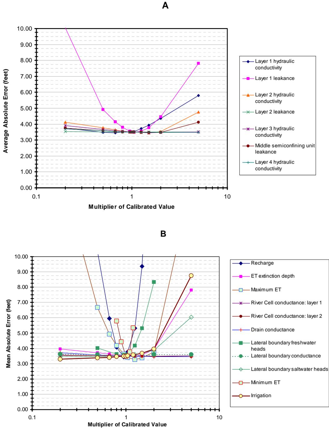
Figure 77. Sensitivity of surficial aquifer system (layer 1) simulated heads to changes in (A) aquifer and confining unit parameters and (B) selected boundary conditions
