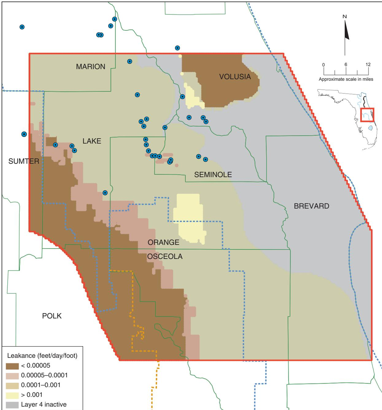
Figure 74. Calibrated leakance of the middle semiconfining unit
