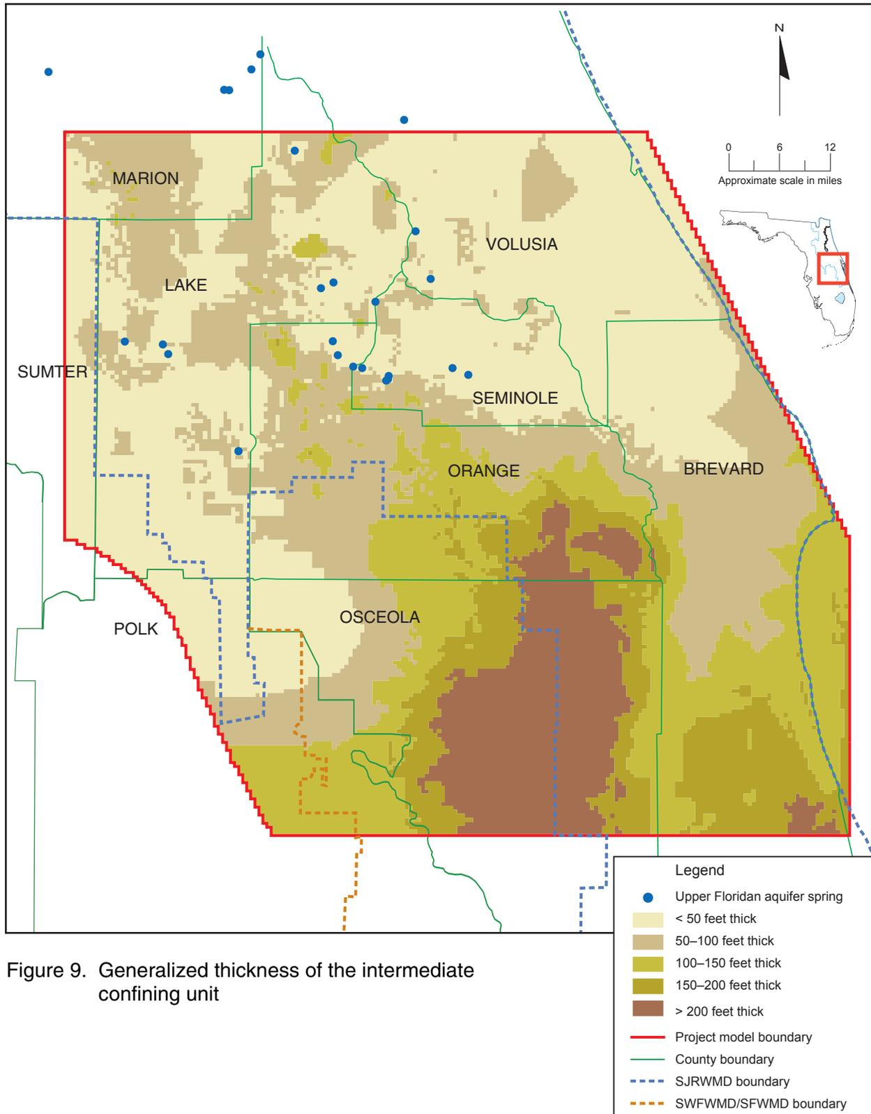
Figure 9. Generalized thickness of the intermediate confining unit
