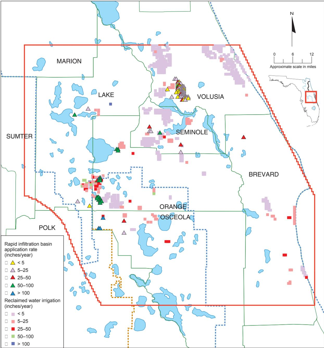
Figure 34. Average 1995 reclaimed water application rates
