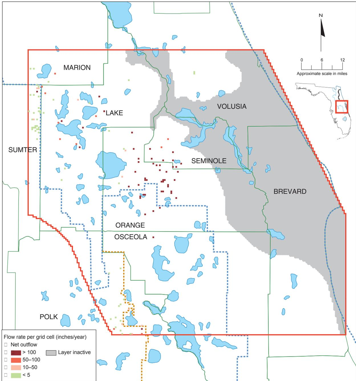
Figure 32. Average 1995 withdrawals applied to model layer 4
