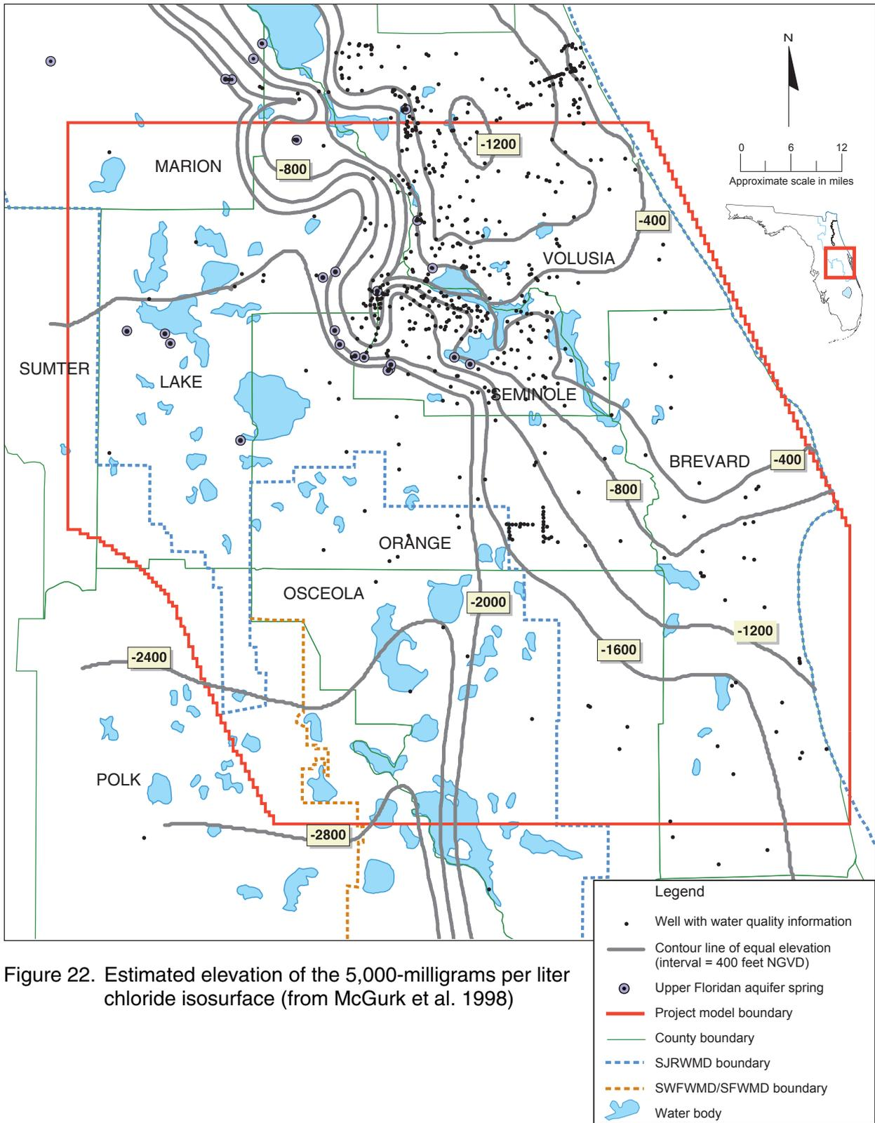
Figure 22. Estimated elevation of the 5,000-milligrams per liter chloride isosurface (from McGurk et al. 1998)
