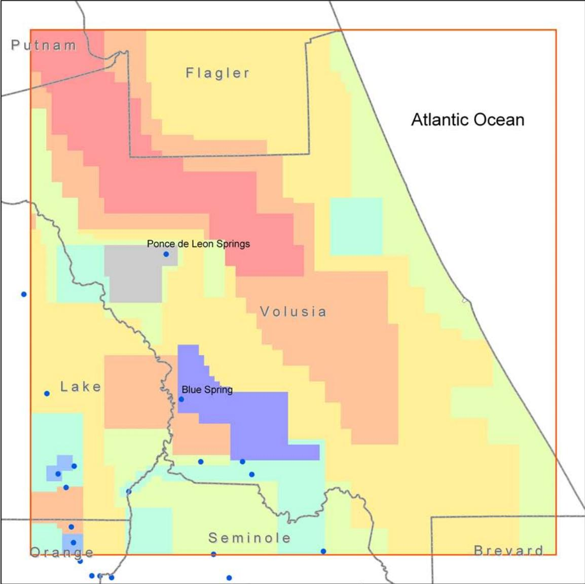
Figure 66. Calibrated horizontal hydraulic conductivity of the Upper Floridan aquifer
