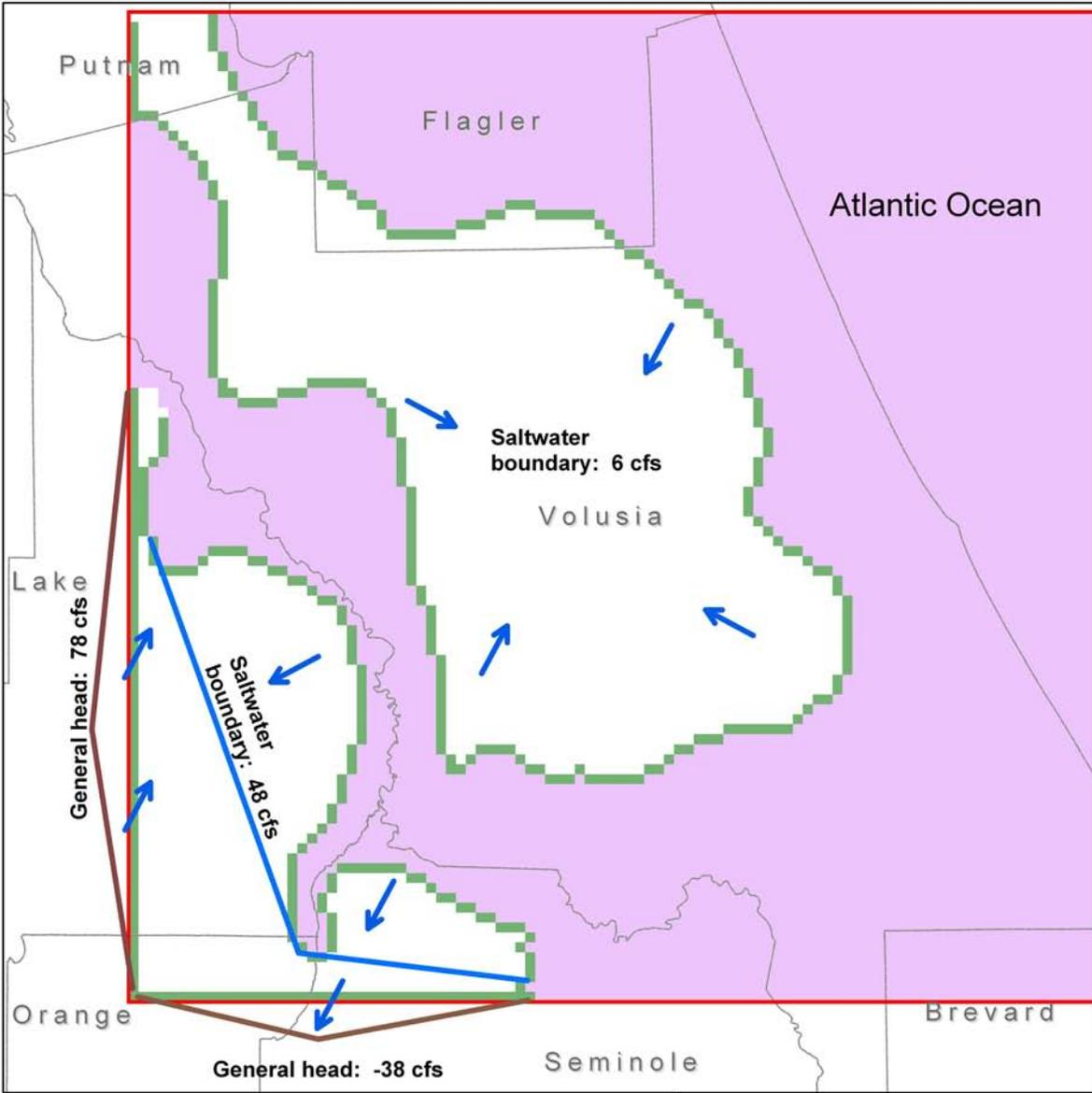
Figure 72. Simulated fluxes to and from general head boundaries assigned to model layer 3, 1995 calibration, in cubic feet per second (cfs)
