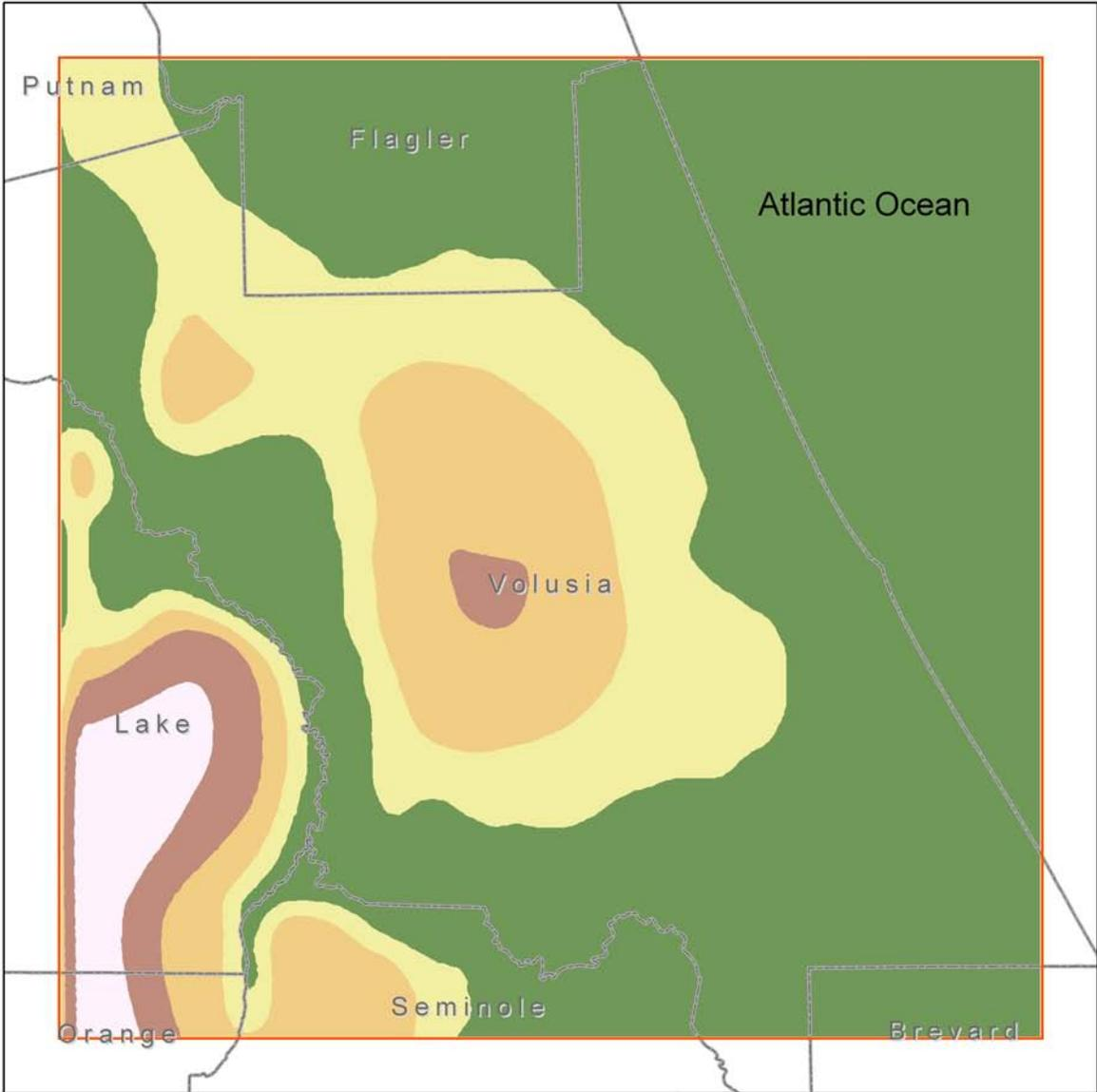
Figure 46. Estimated thickness of the Lower Floridan aquifer with the base modified to the elevation of the 5,000-parts per million chloride isochlor
