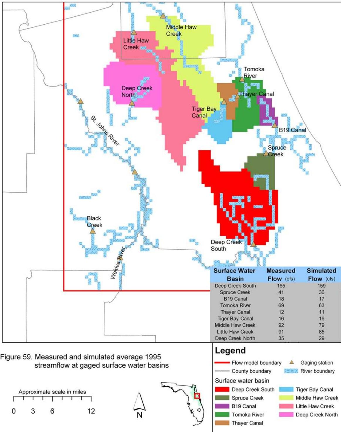
Figure 59. Measured and simulated average 1995 streamflow at gaged surface water basins
