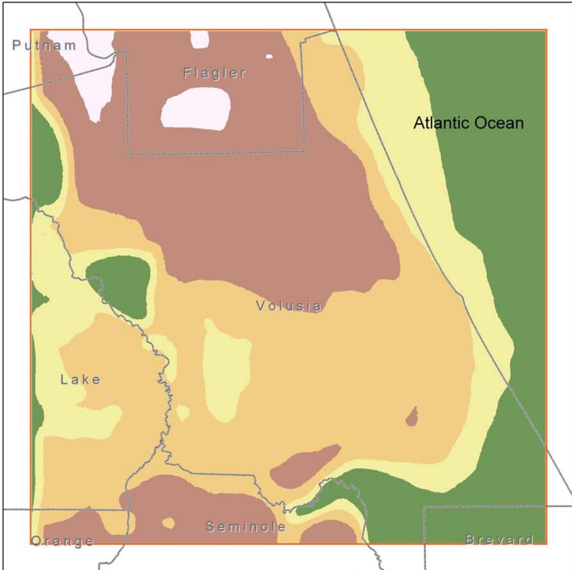
Figure 45. Estimated thickness of the Upper Floridan aquifer with the base modified to the elevation of the 5,000-parts per million chloride isochlor
