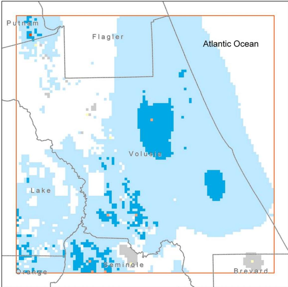
Figure 80. Differences between simulated rates of recharge to or discharge from the Upper Floridan aquifer for the 2020 projection and for the 1995 calibration
