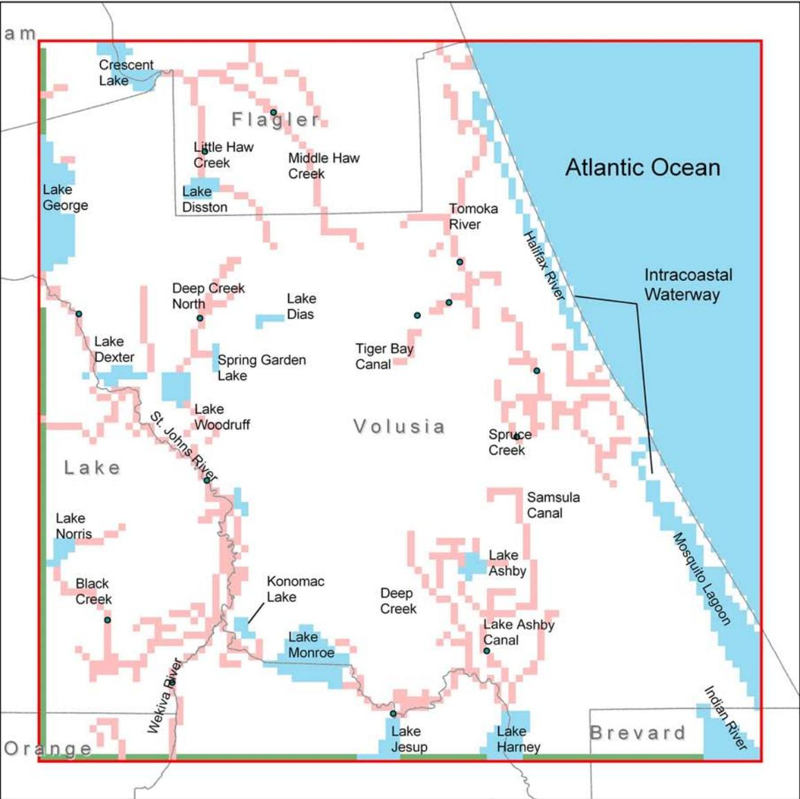
Figure 28. Locations and types of boundary conditions for the surficial aquifer system (model layer 1)
