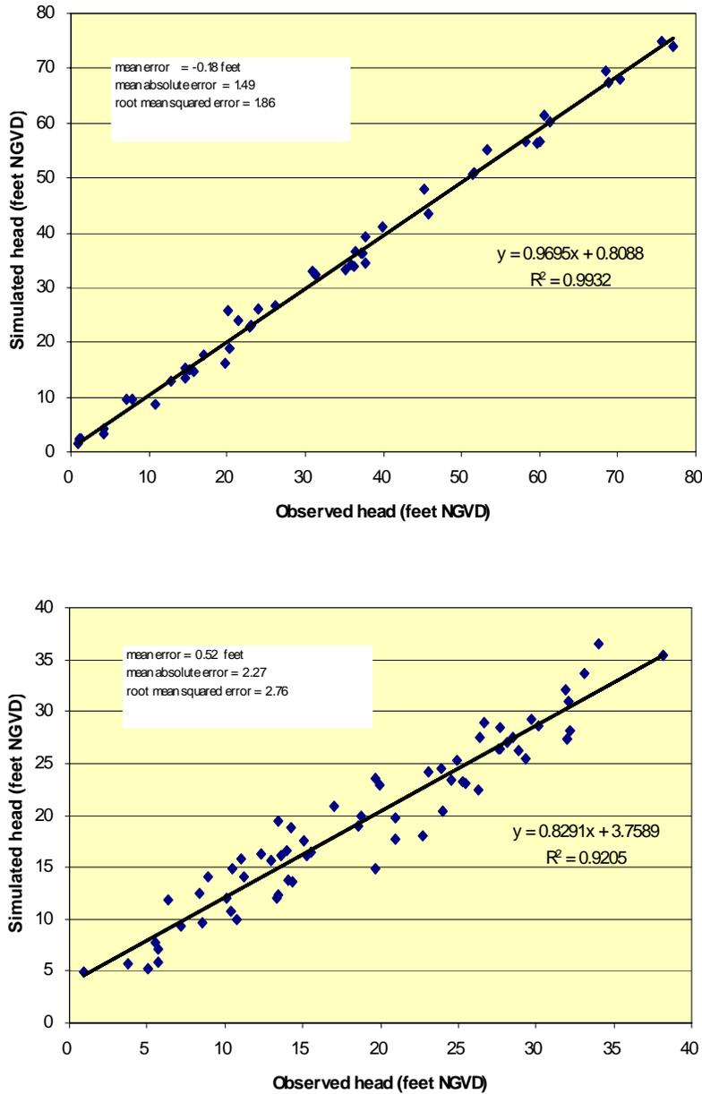
Figure 53. Trend lines of simulated and observed average 1995 heads for (A) water levels within the surficial aquifer system and (B) potentiometric levels within the Upper Floridan aquifer
