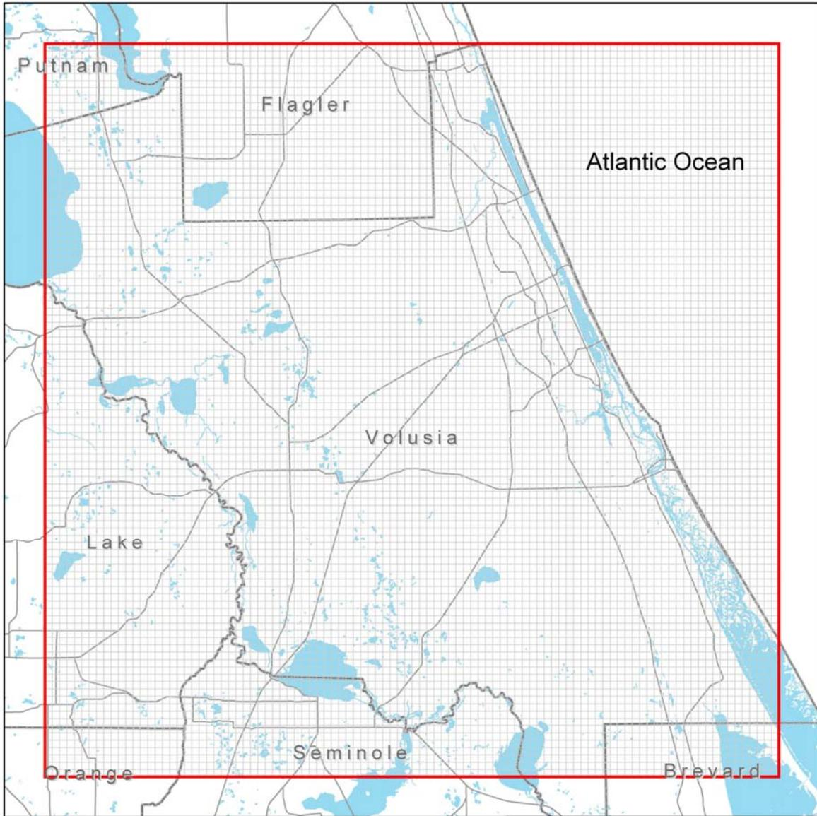
Figure 27. Orientation of the finite-difference grid
