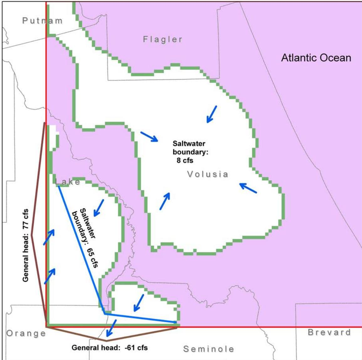
Figure 81. Simulated fluxes to and from general head boundaries assigned to model layer 3, 2020 projection in cubic feet per second (cfs)
