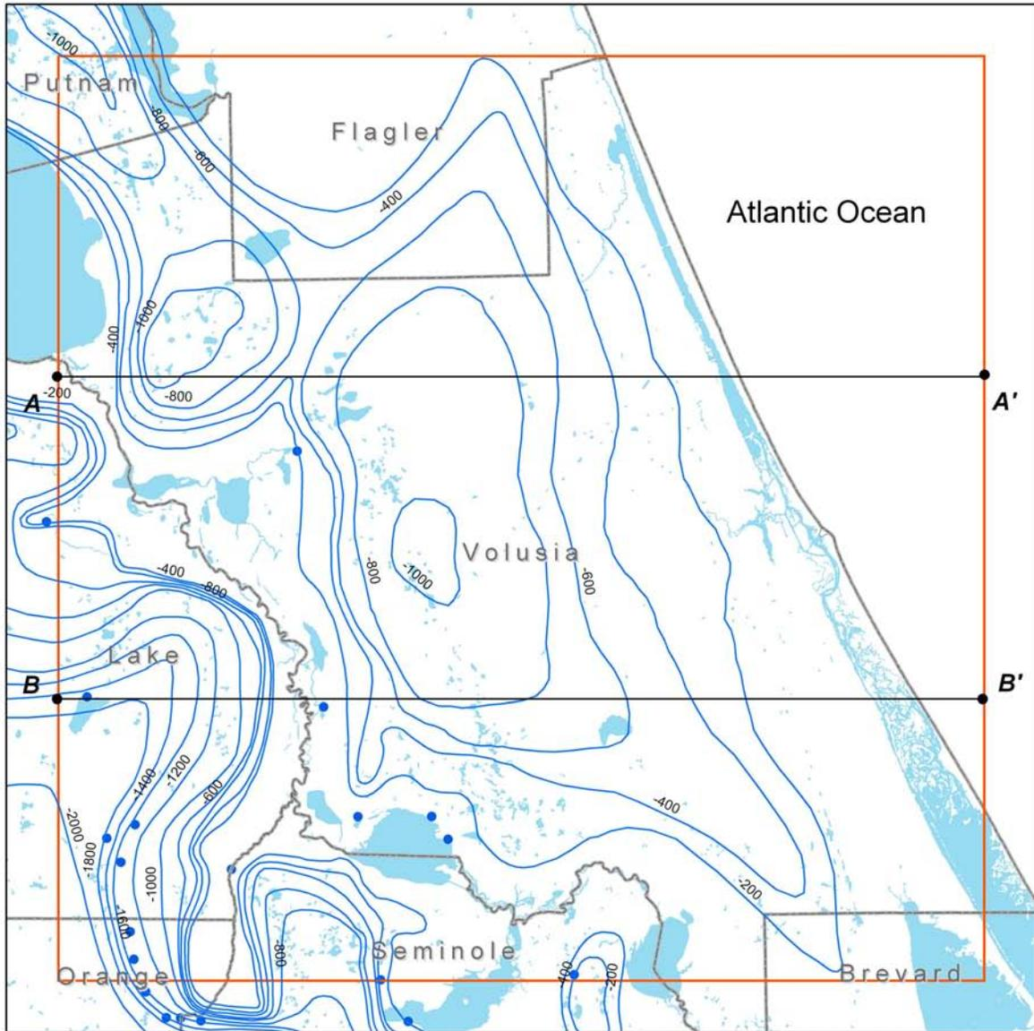
Figure 23. Estimated elevation of the 5,000-parts per million chloride isochlor and locations of cross sections shown in Figures 25 and 26
