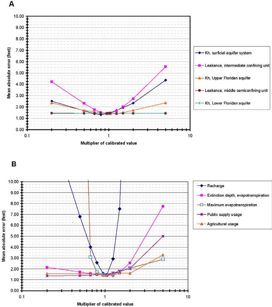
Figure 73. Sensitivity of simulated surficial aquifer system heads to changes in (A) aquifer and confining unit properties and (B) selected boundary conditions
