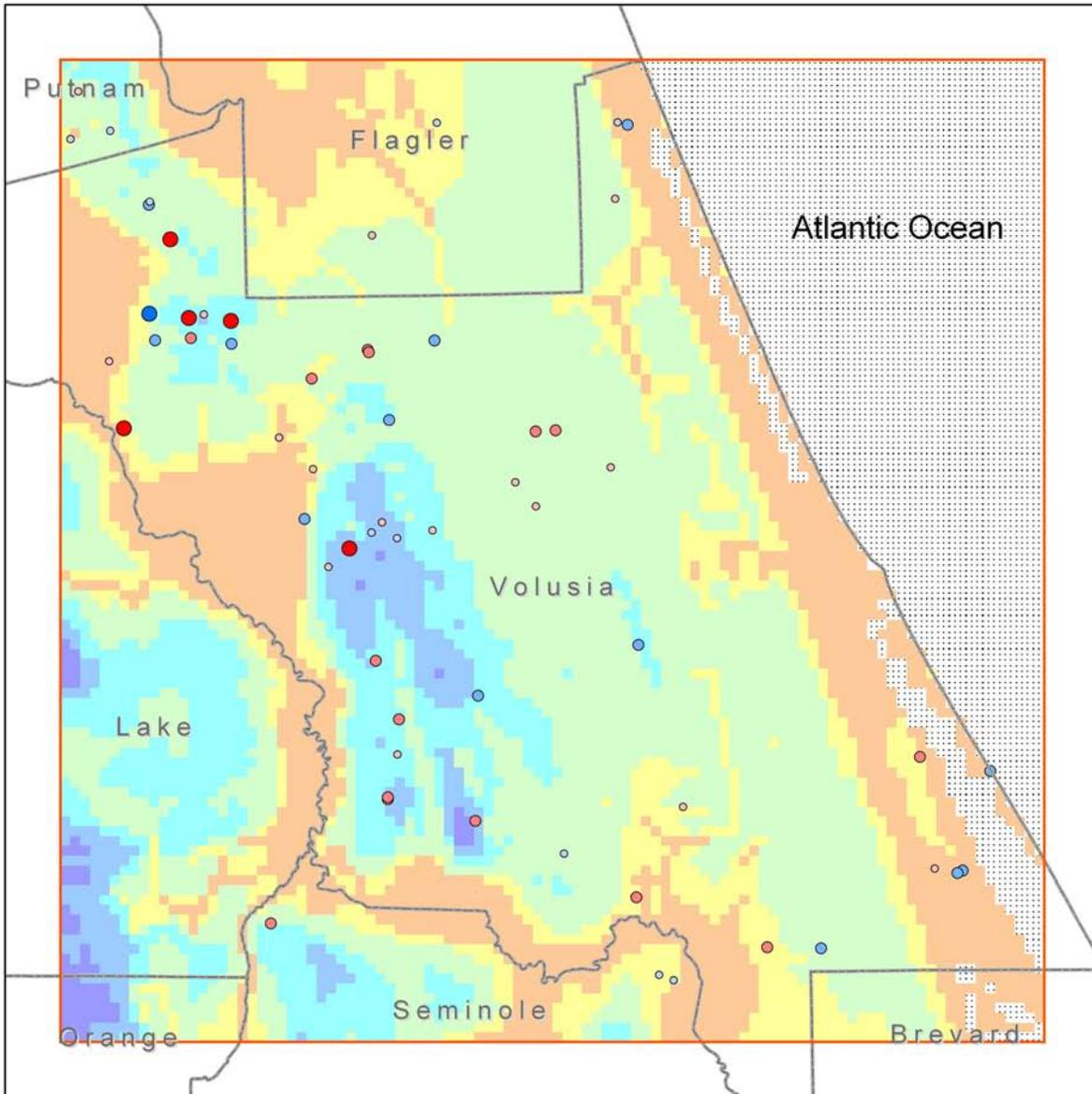
Figure 52. Simulated average 1995 water table and head residuals, surficial aquifer system (model layer 1)
