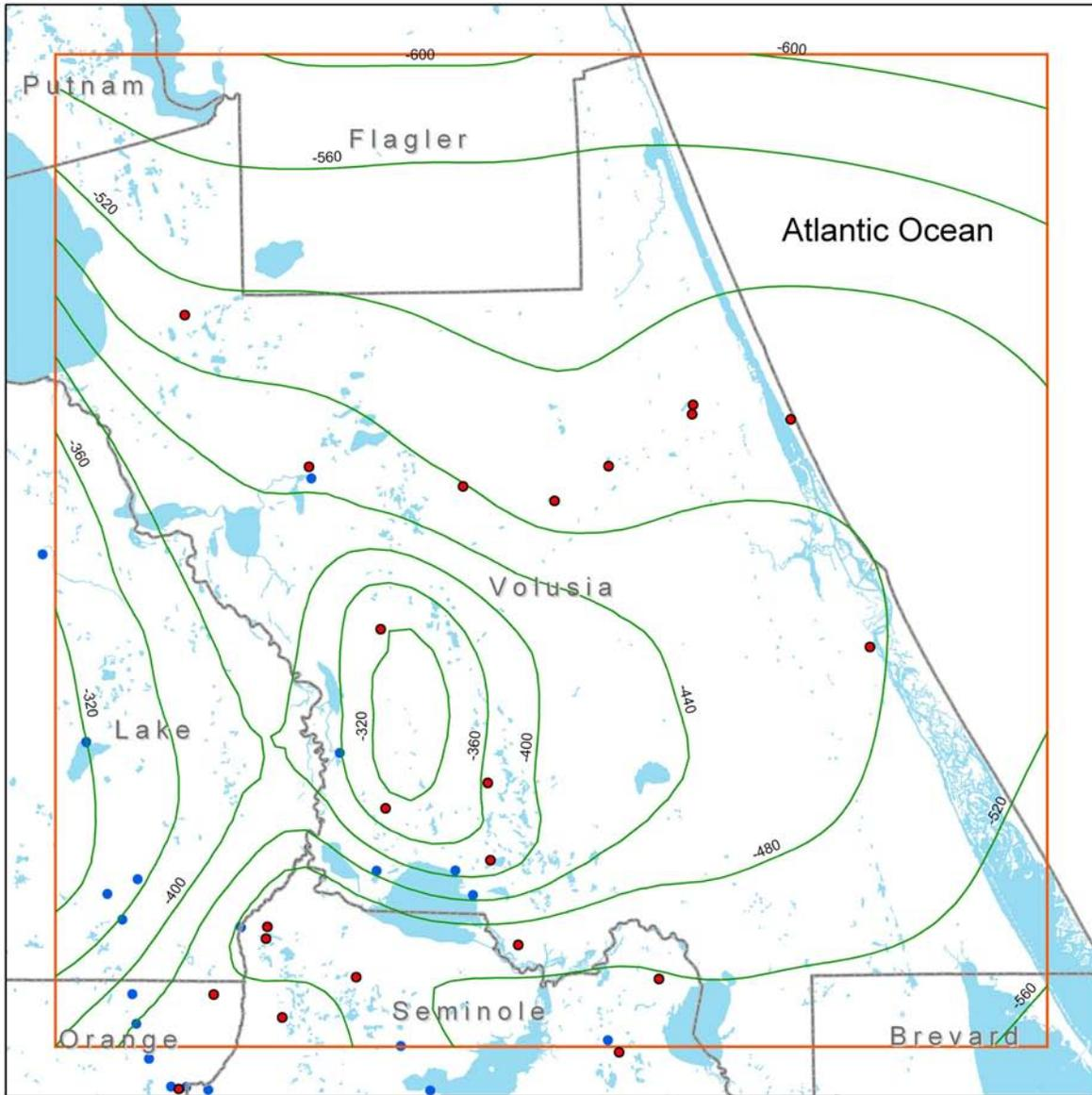
Figure 12. Elevation at the stratigraphic base of the Upper Floridan aquifer
