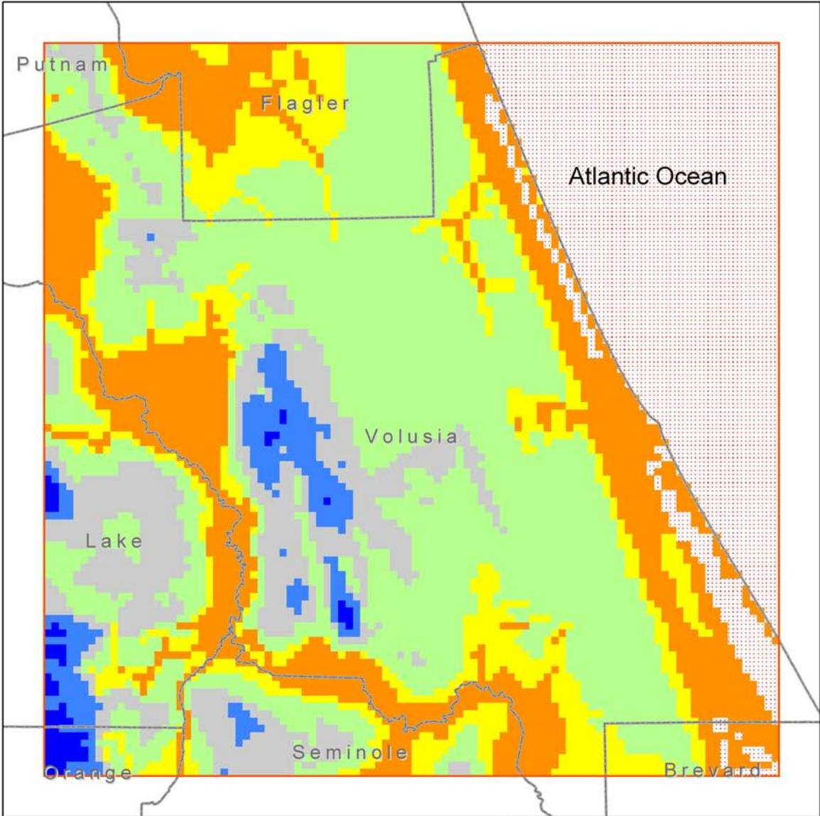
Figure 47. The simulated predevelopment water table in the surficial aquifer system
