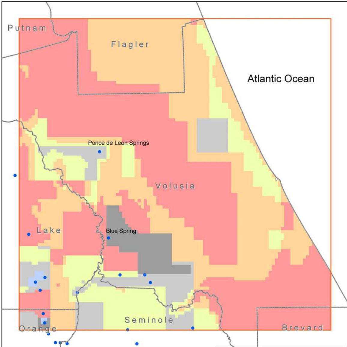
Figure 67. Calibrated transmissivity of the Upper Floridan aquifer
