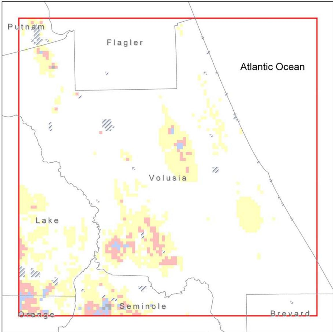
Figure 82. Distribution and range of simulated minimum drawdown of the water table between 1995 and 2020
