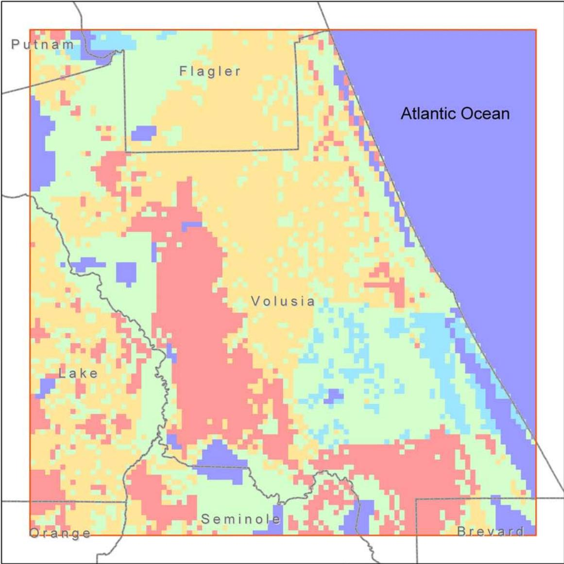
Figure 35. Distribution and rate of overland runoff derived from Soil Conservation Survey curve numbers
