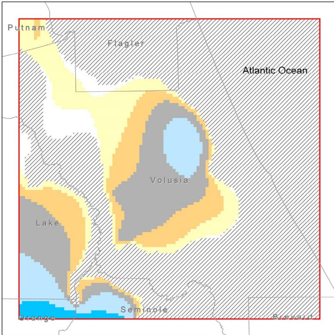
Figure 78. Projected declines in the elevation of the potentiometric surface of the Lower Floridan aquifer between 1995 and 2020
