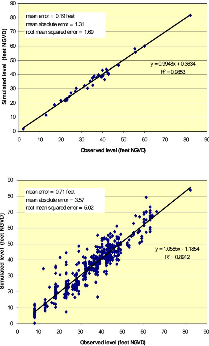
Figure 57. Trend lines of simulated and observed water levels for (A) lakes with stage data for 1995 and (B) lakes with elevations posted on the U.S. Geological Survey maps
