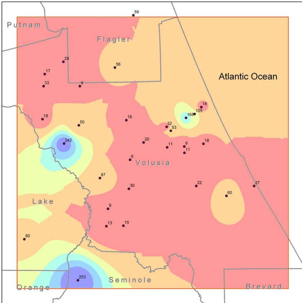
Figure 18. Measurements and interpolated trends of transmissivity of the Upper Floridan aquifer based upon aquifer test results
