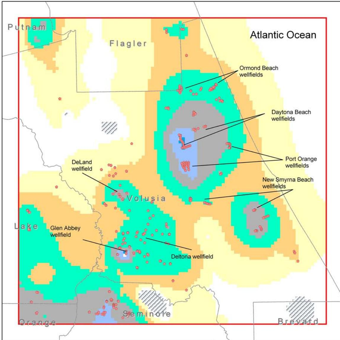
Figure 77. Projected declines in the elevation of the potentiometric surface of the Upper Floridan aquifer between 1995 and 2020
