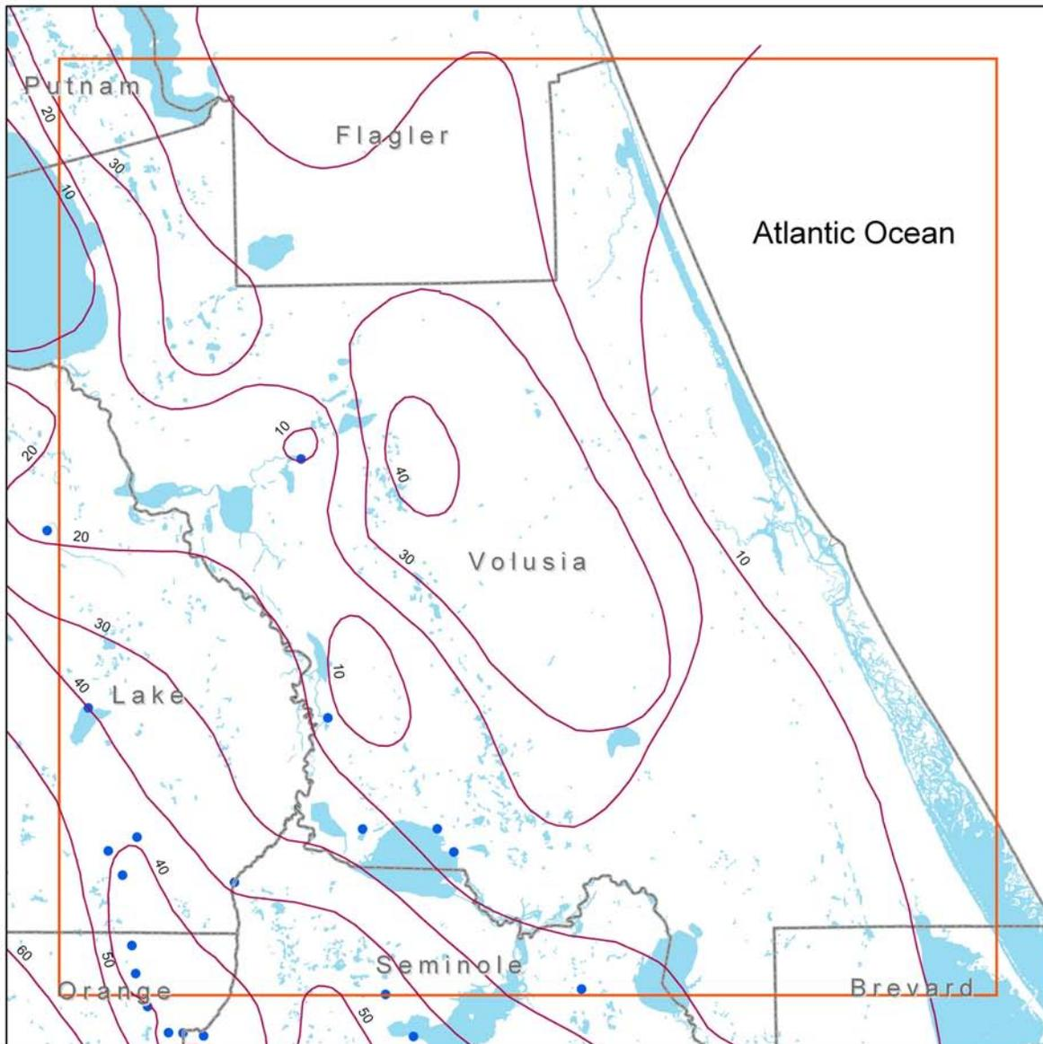
Figure 19. Estimated predevelopment potentiometric surface of the Upper Floridan aquifer (adapted from Johnston et al. 1980)
