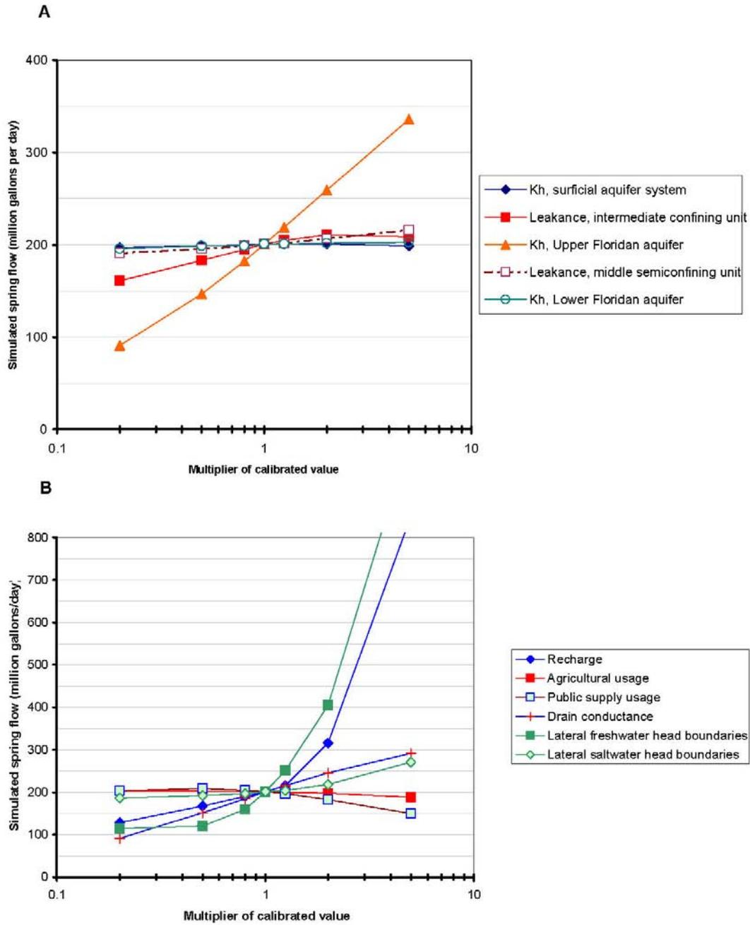
Figure 75. Sensitivity of total simulated spring flow to changes in (A) aquifer and confining unit properties and (B) selected boundary conditions
