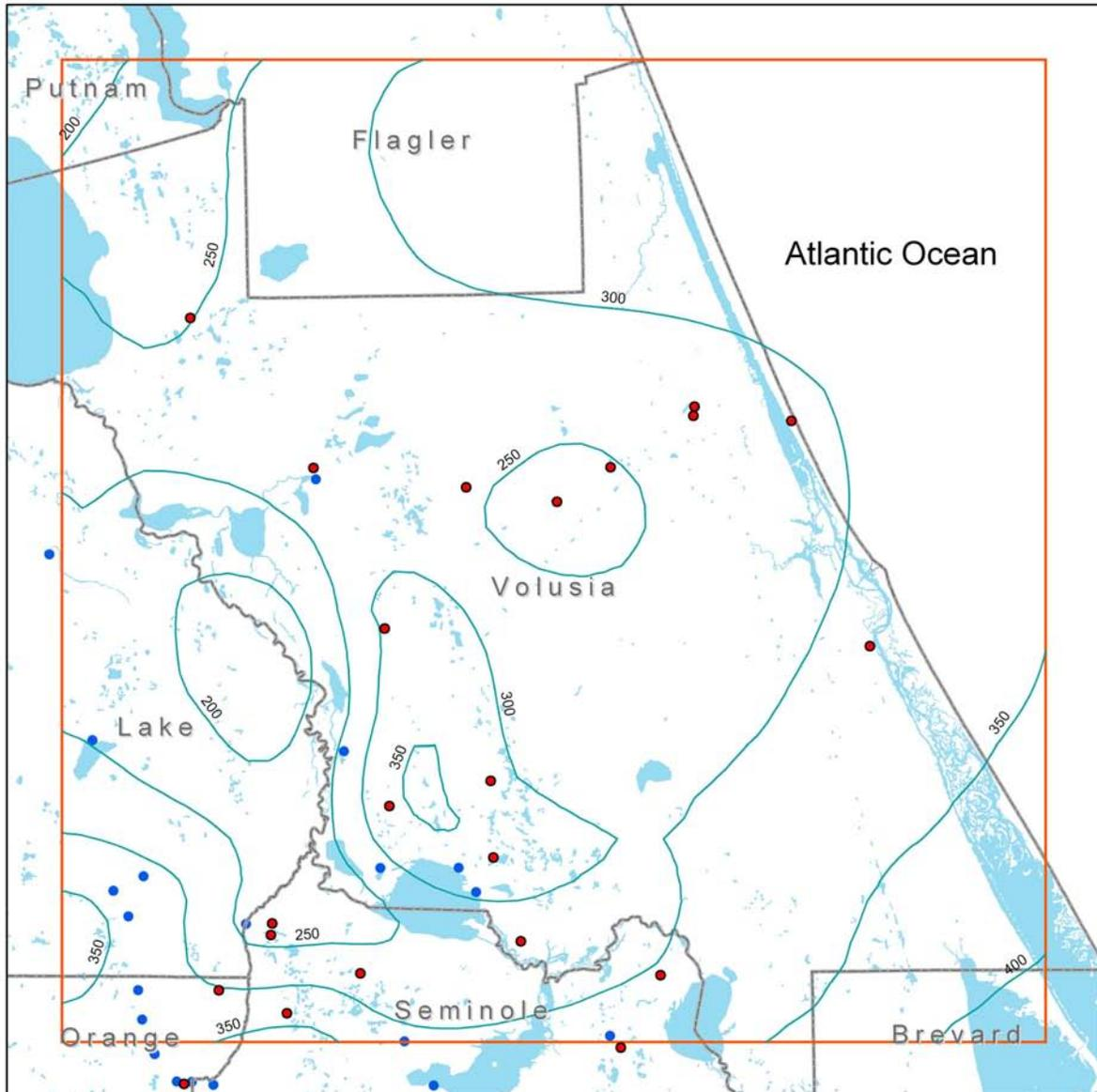
Figure 14. Generalized thickness of the middle semiconfining unit within the Floridan aquifer system
