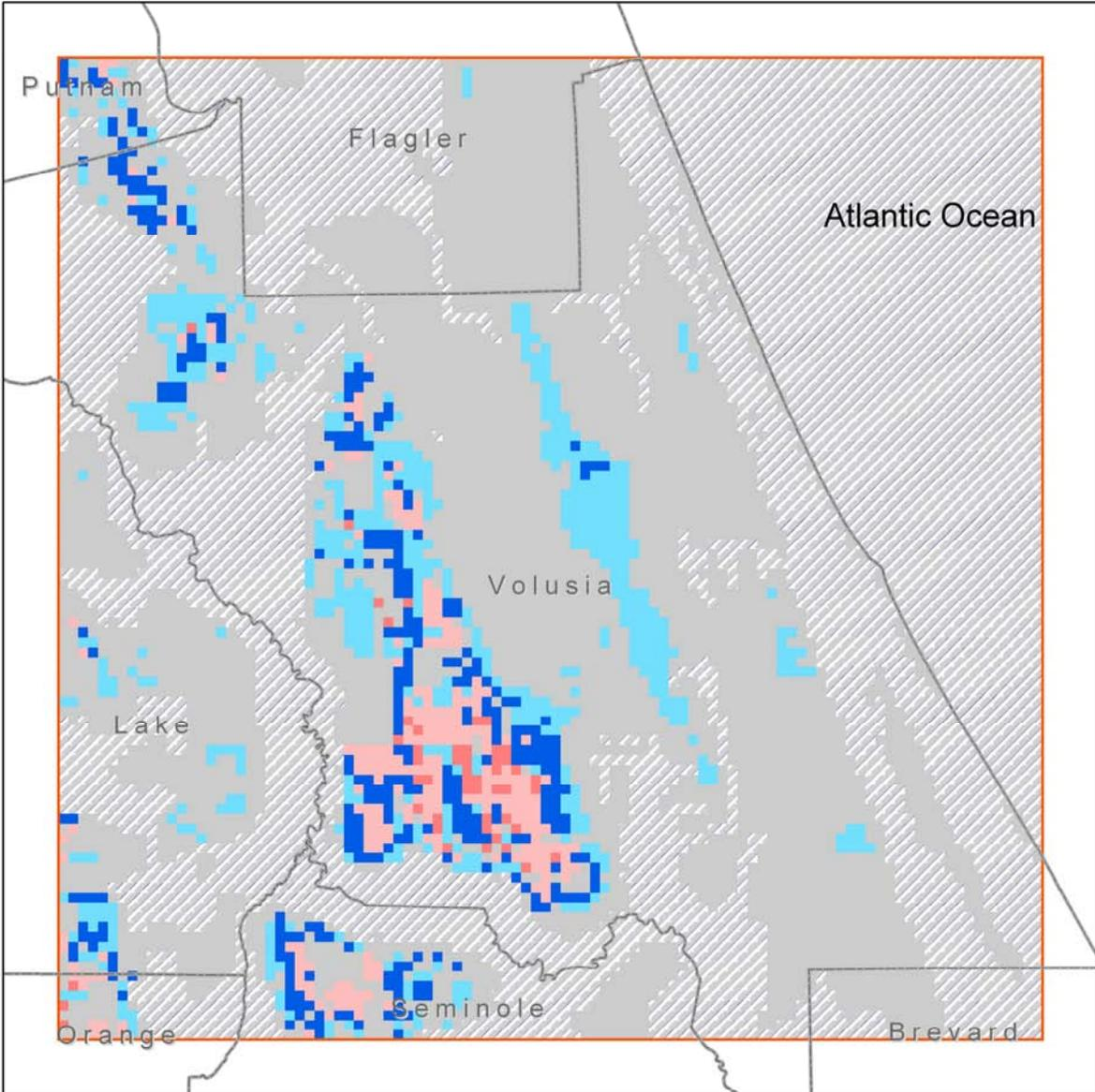
Figure 63. Distribution and rate of simulated recharge to or discharge from the Upper Floridan aquifer based upon the average 1995 calibration
