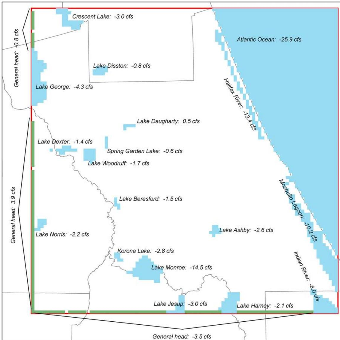
Figure 70. Simulated fluxes to and from constant and general head boundaries assigned to model layer 1, 1995 calibration in cubic feet per second (cfs)
