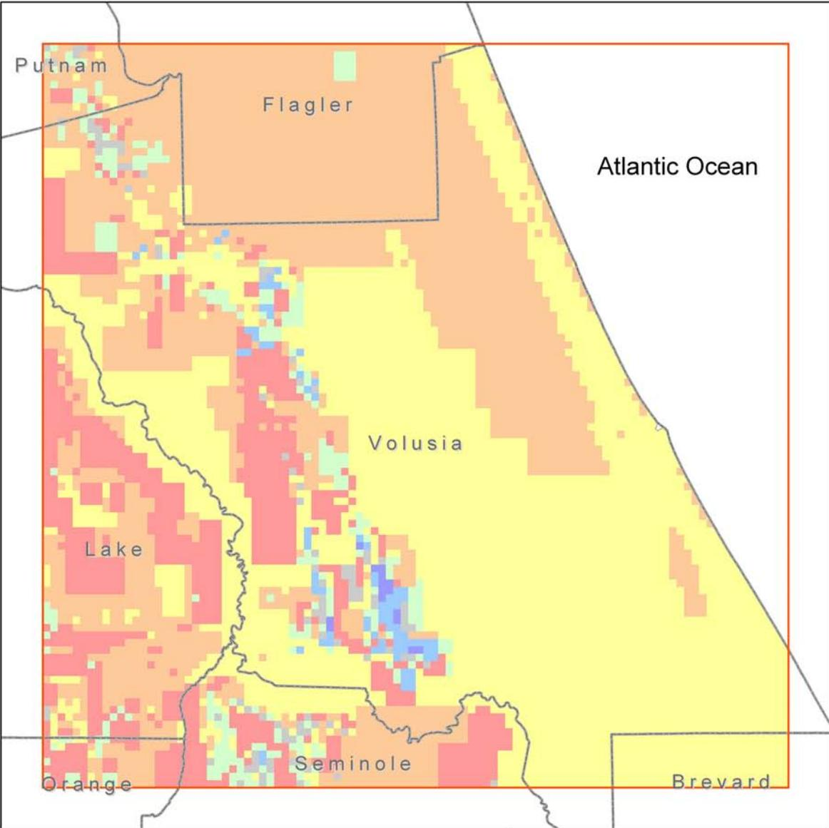
Figure 65. Calibrated leakance of the intermediate confining unit
