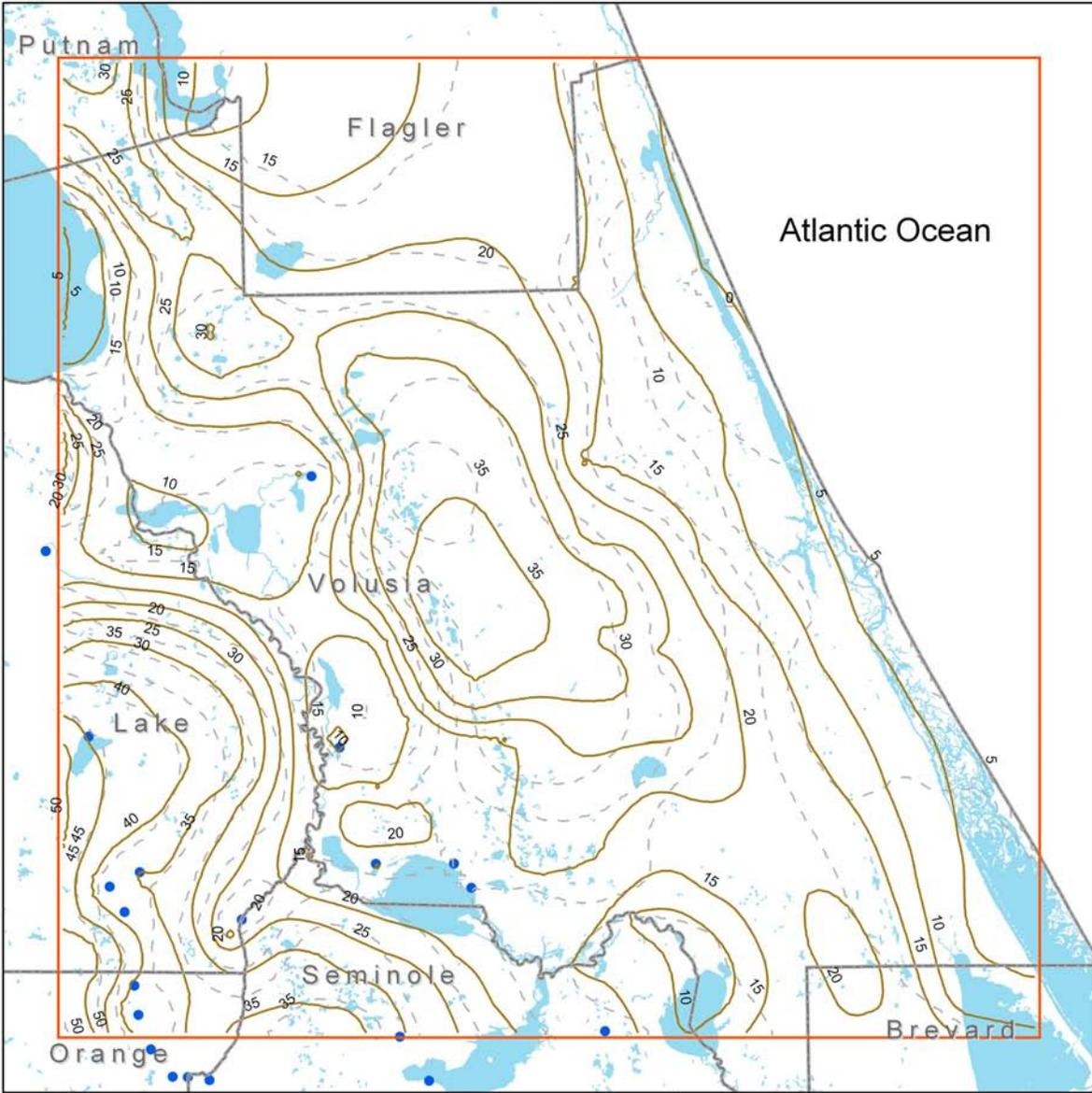
Figure 60. Simulated and estimated average 1995 potentiometric surfaces, Upper Floridan aquifer (model layer 2)
