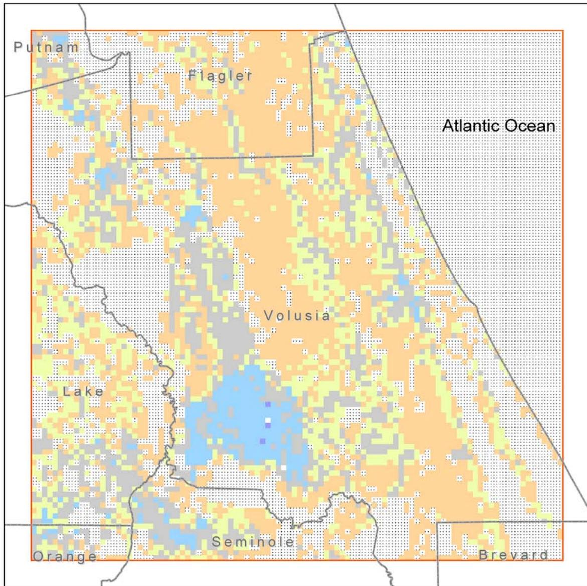
Figure 62. Distribution and rate of net recharge to the surficial aquifer system based upon the average 1995 calibration
