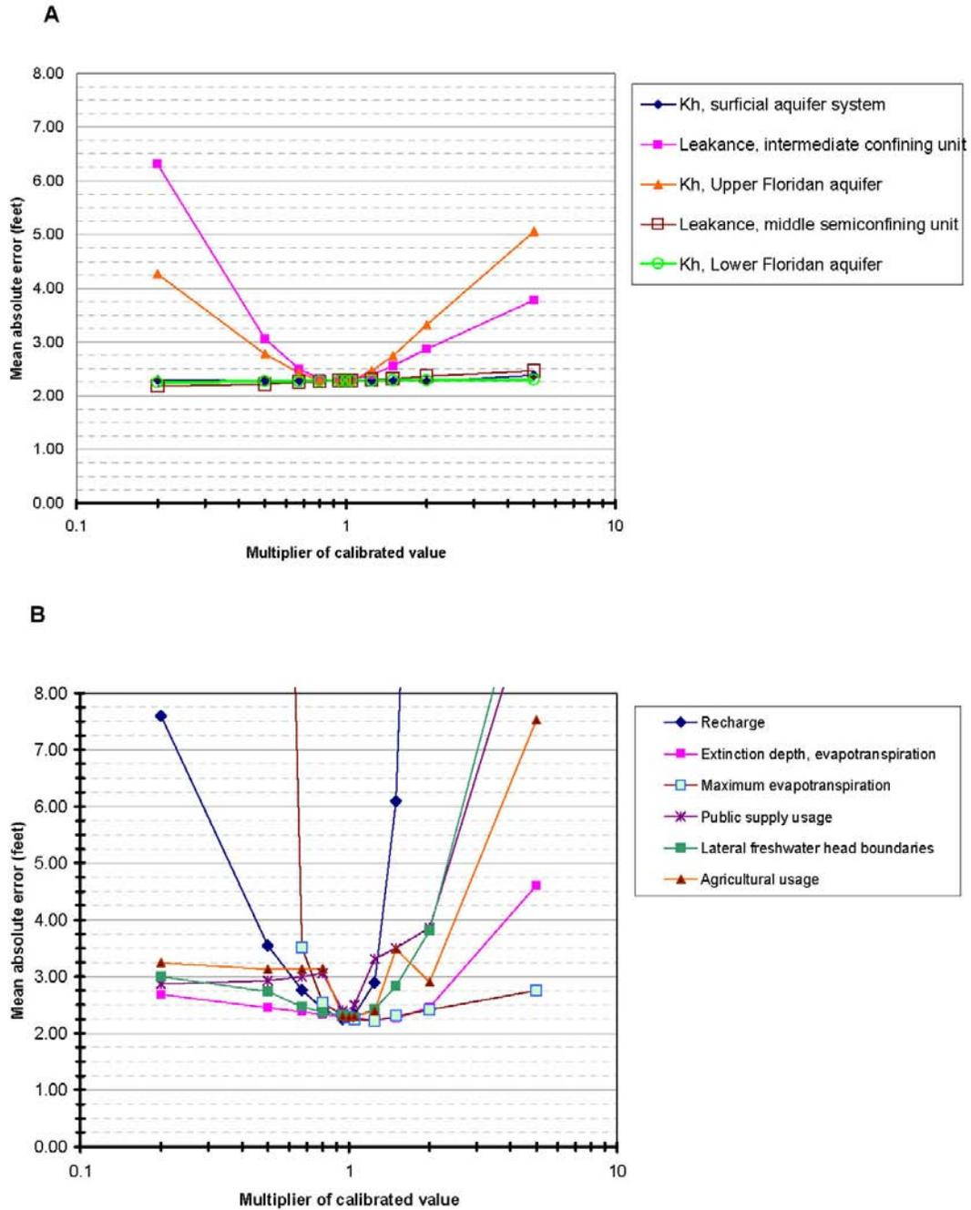
Figure 74. Sensitivity of simulated Upper Floridan aquifer heads to changes in (A) aquifer and confining unit properties and (B) selected boundary conditions
