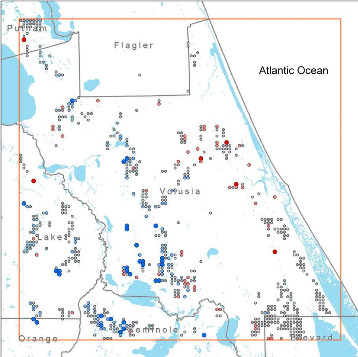
Figure 58. Head residuals at lakes based on elevation data from U.S. Geological Survey topographic maps and corresponding simulated average 1995 water levels, surficial aquifer system (model layer 1)
