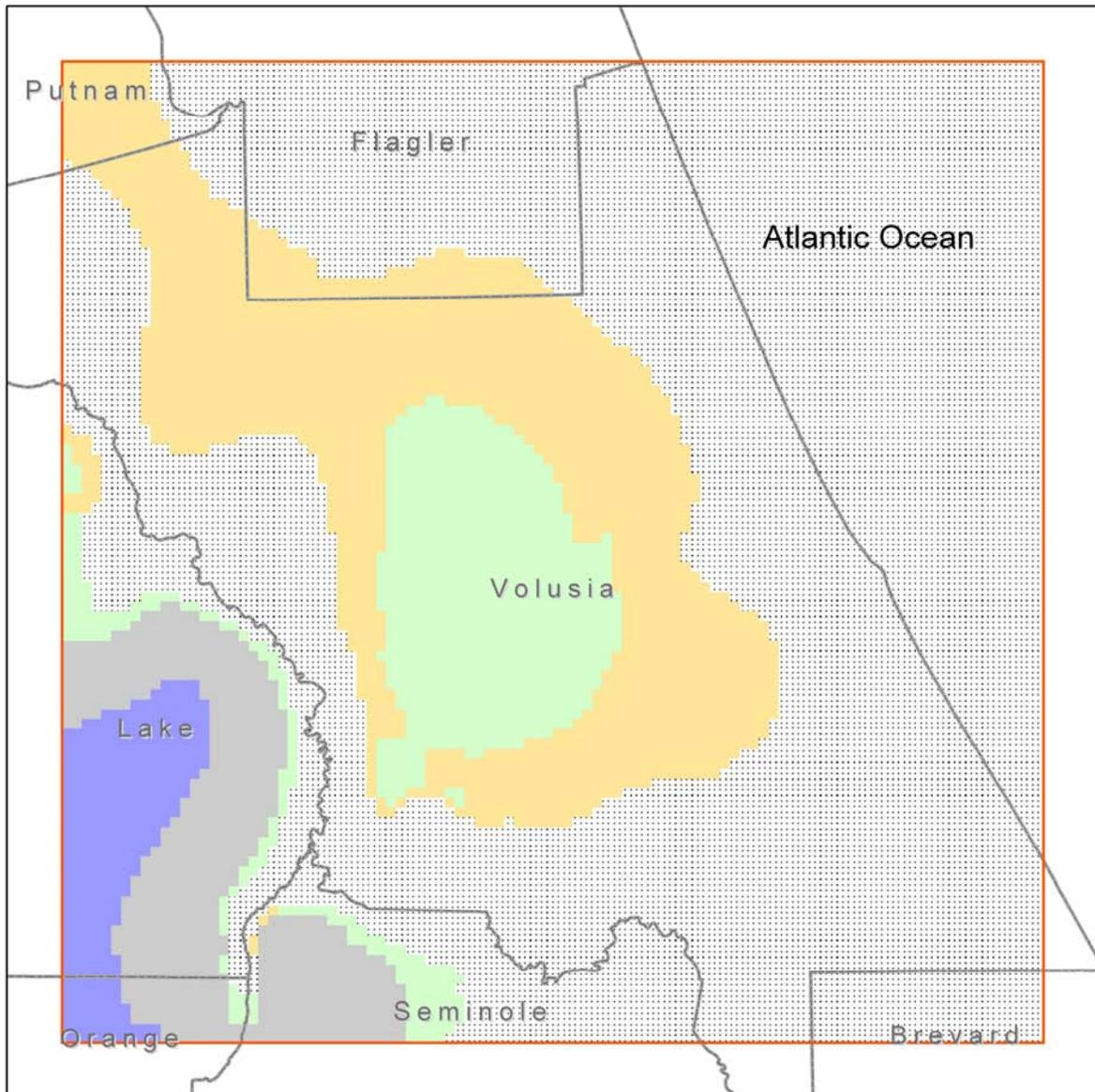
Figure 69. Calibrated transmissivity of the Lower Floridan aquifer
