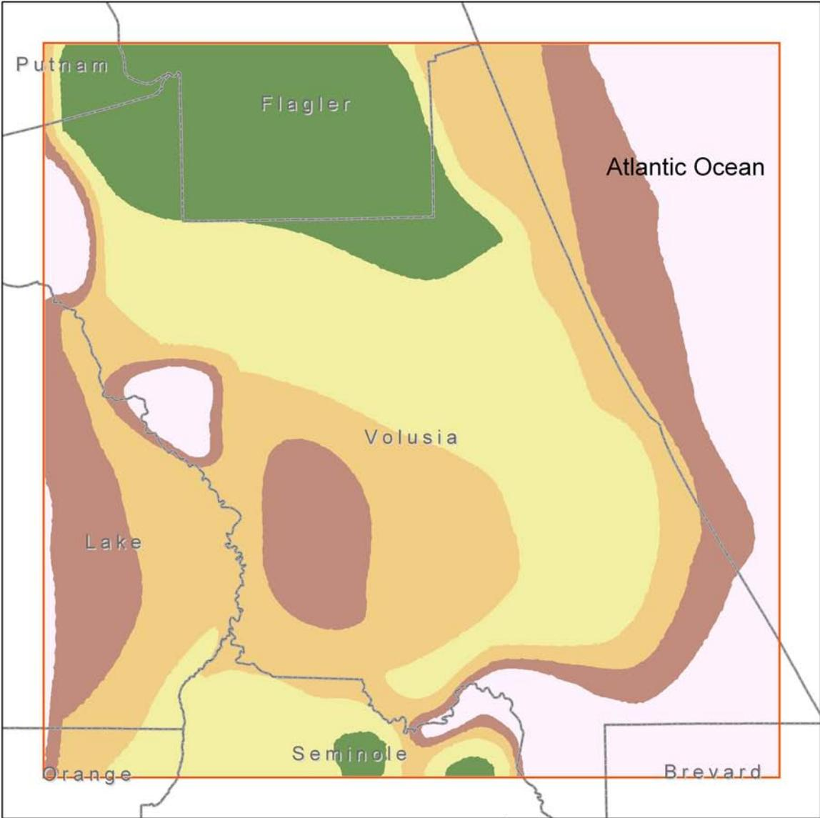
Figure 44. Estimated elevation of the base of the Upper Floridan aquifer modified to the elevation of the 5,000-parts per million chloride isochlor
