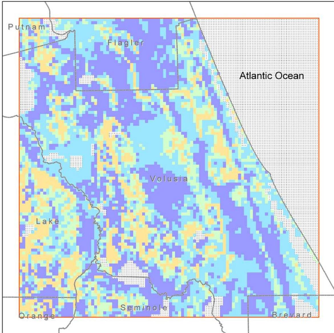
Figure 61. Distribution and rate of total evapotranspiration based upon the average 1995 calibration
