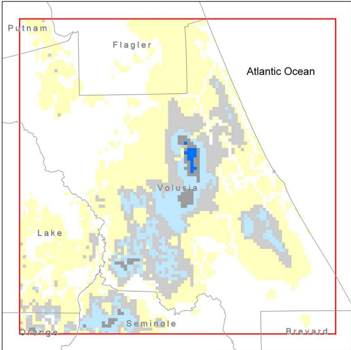
Figure 84. Distribution and range of the difference between simulated maximum and minimum potential drawdown of the water table between 1995 and 2020
