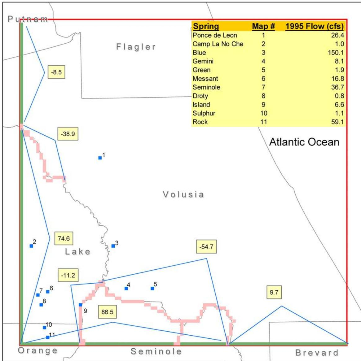
Figure 71. Simulated fluxes to and from specified boundaries assigned to model layer 2, 1995 calibration, in cubic feet per second (cfs)
