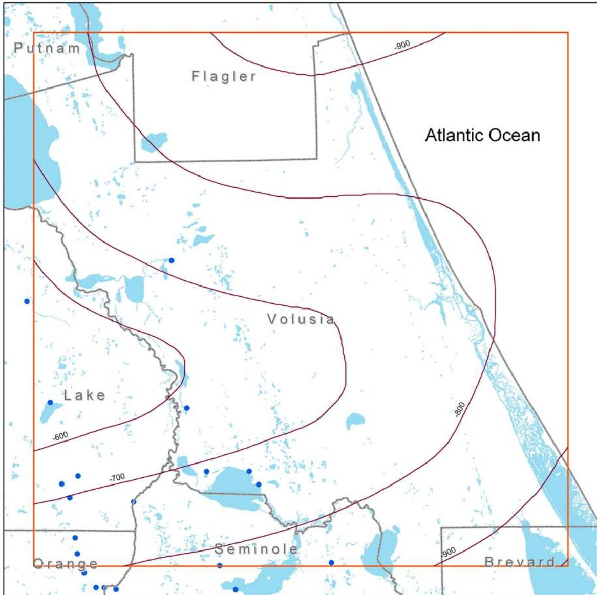
Figure 15. Elevation at the stratigraphic top of the Lower Floridan aquifer
