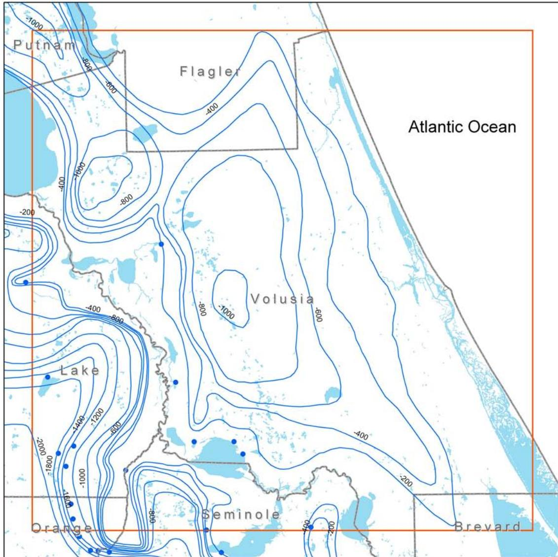
Figure 22. Estimated elevation of the 250-parts per million chloride isochlor
