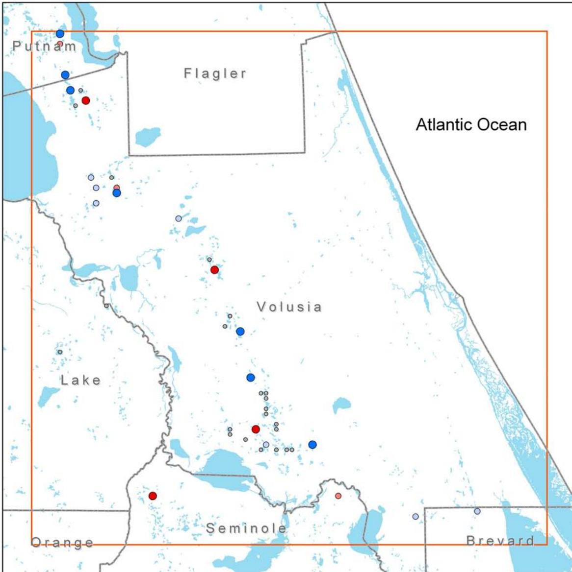
Figure 56. Head residuals based on 1995 measured lake levels compared to corresponding simulated water levels, surficial aquifer system (model layer 1)
