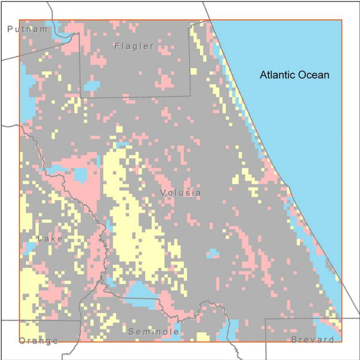
Figure 41. Estimated depth to water derived from the SSURGO database
