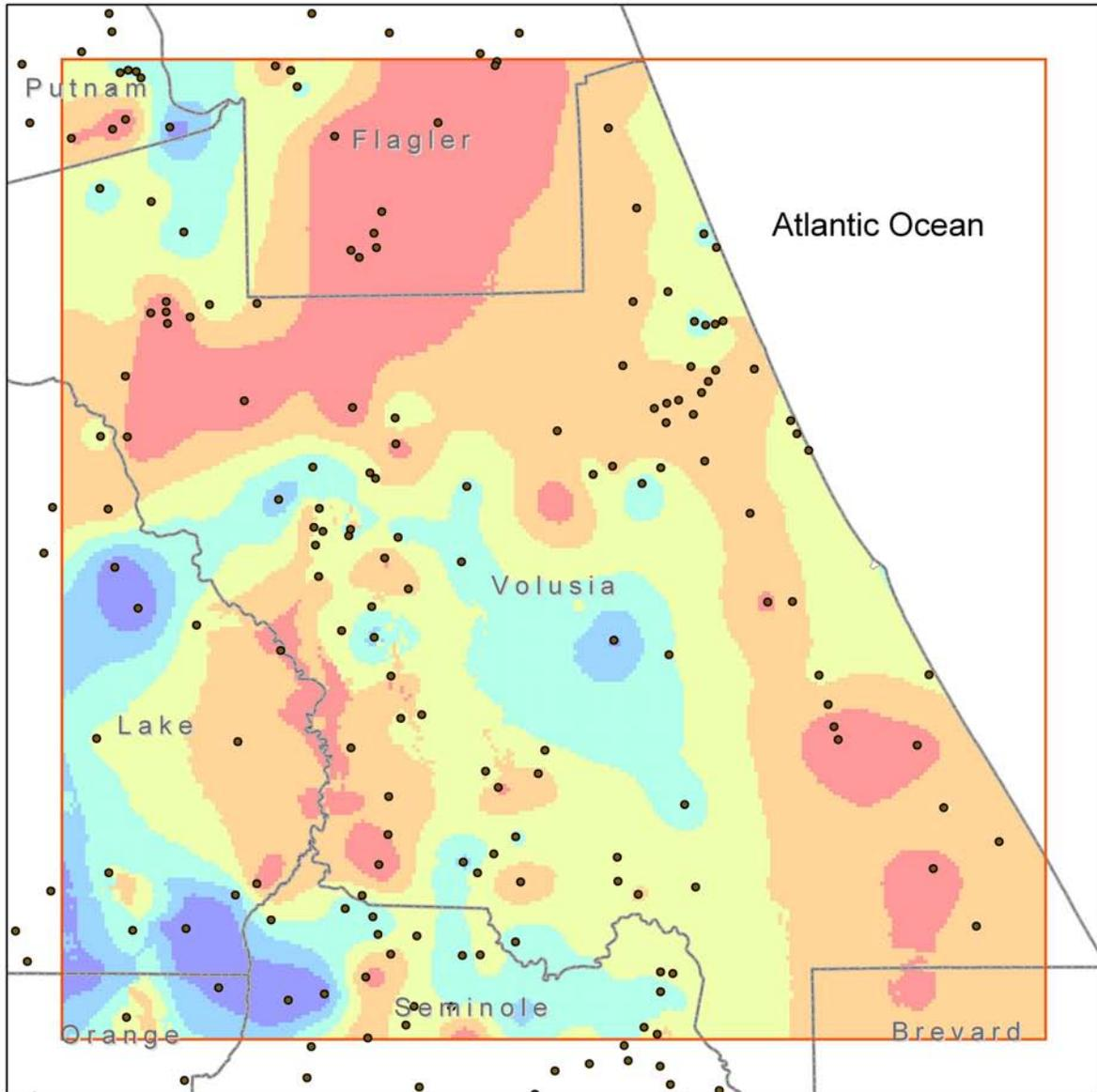
Figure 10. Generalized thickness of the intermediate confining unit
