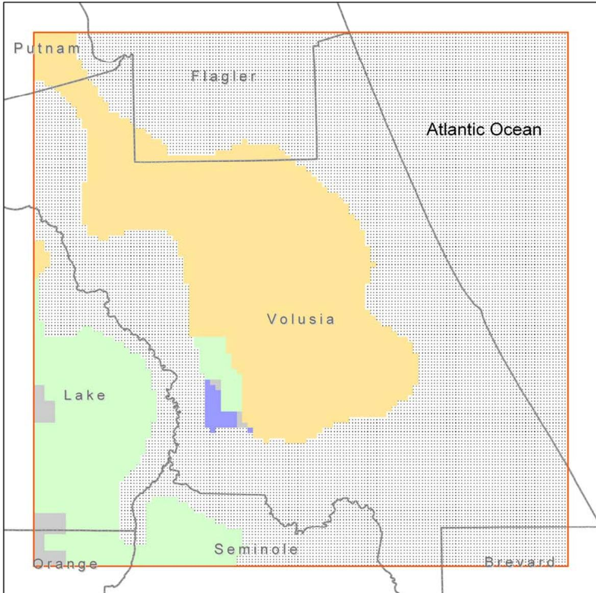
Figure 68. Calibrated leakance of the middle semiconfining unit
