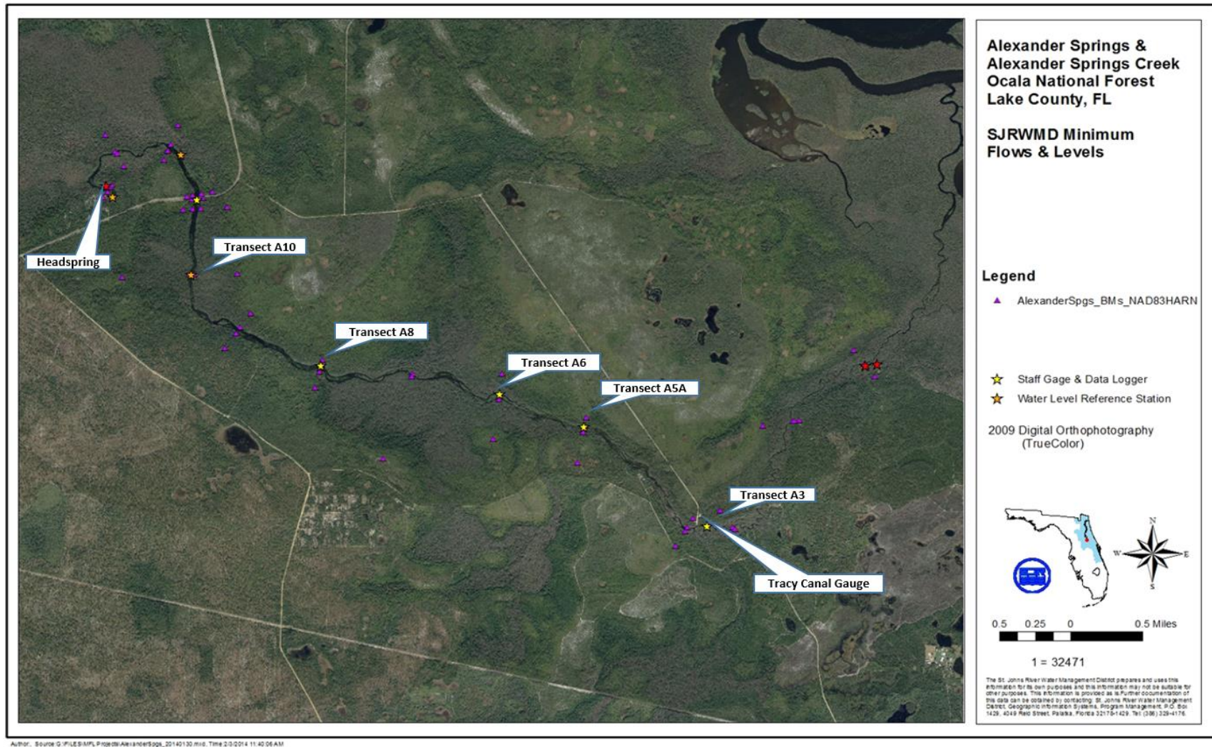
Figure 9. Locations of gauges and HEC-RAS cross-sections
