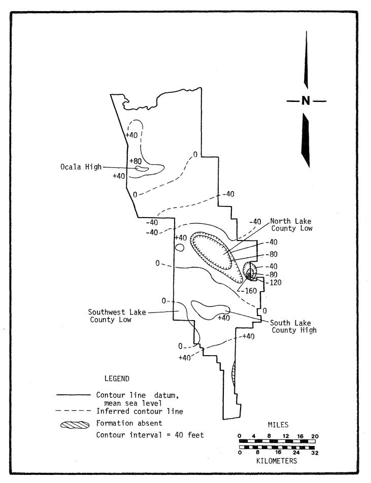
Figure 7. Structure Contour Map of the Top of Ocala Limestone, Oklawaha Basin
