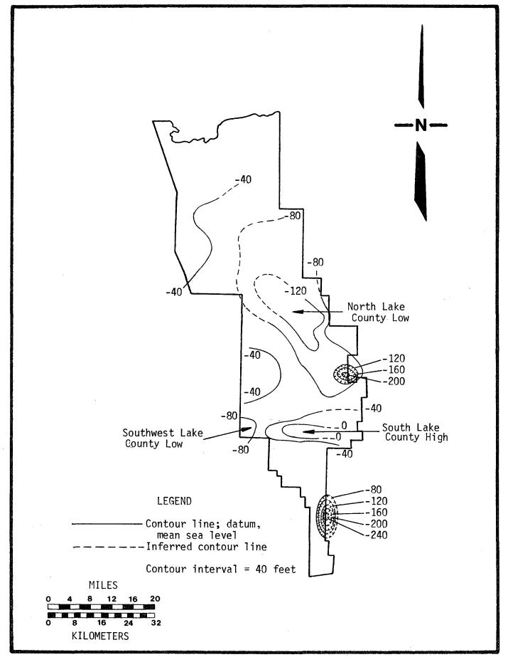
Figure 6. Structure Contour Map of the Top of the Avon Park Limestone, Oklawaha Basin
