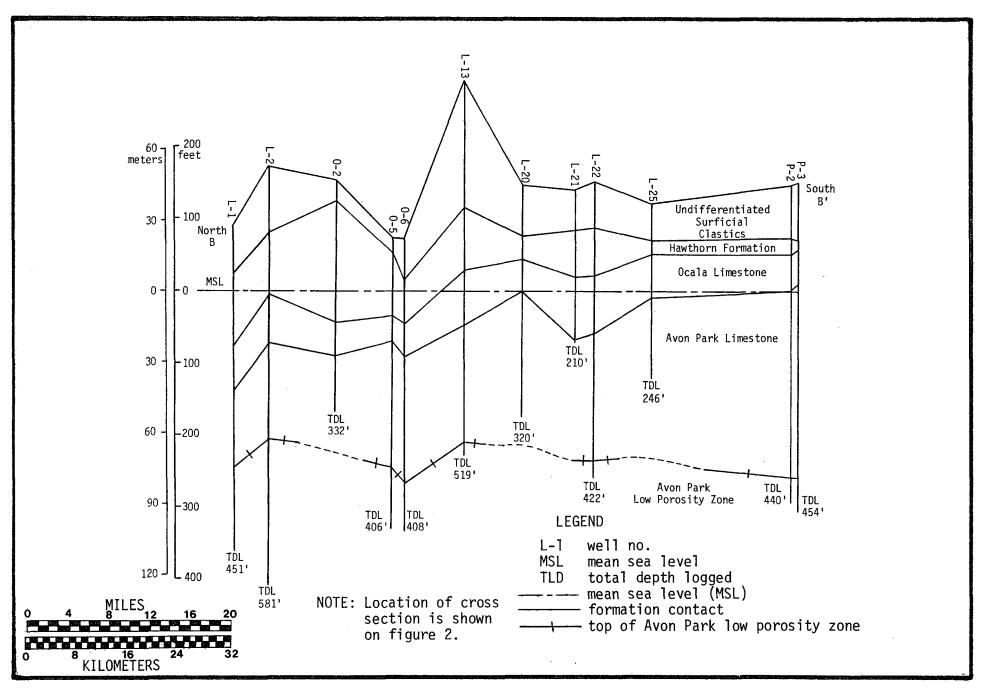
Figure 4. North South Cross Section B-B'
