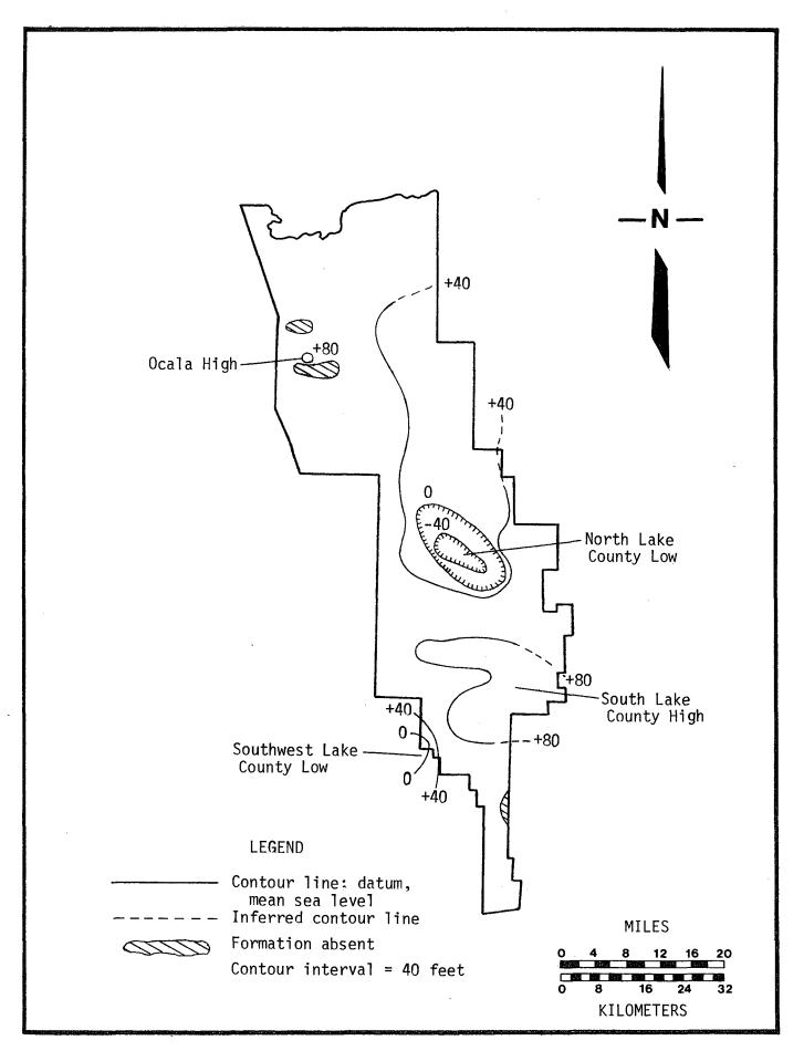
Figure 8. Structure Contour Map of Top of Hawthorn Formation, Oklawaha Basin
