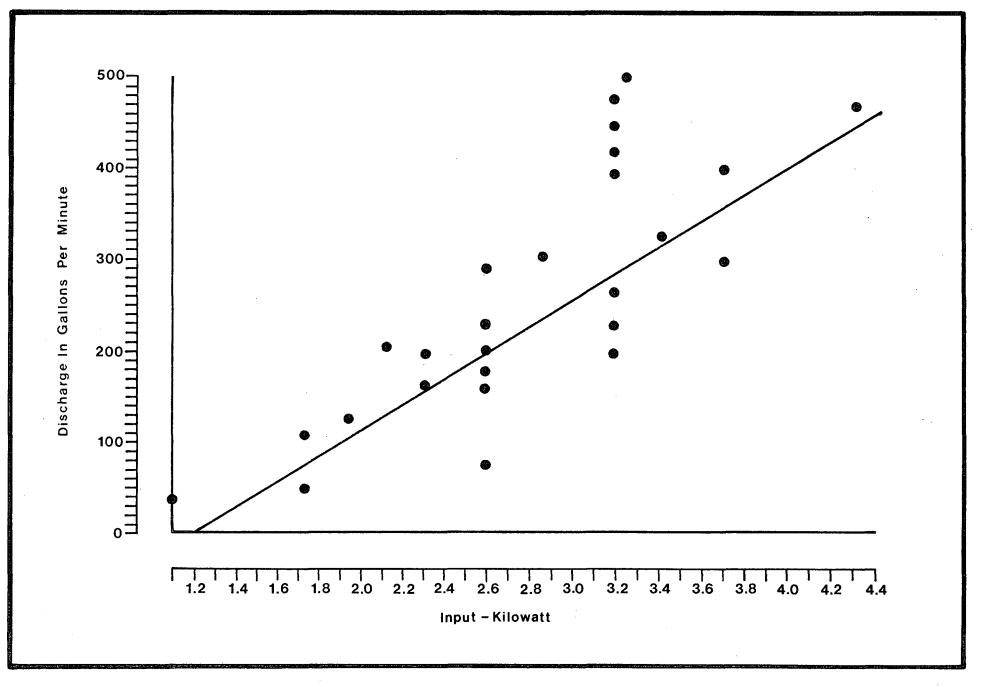
FIGURE 26. -- Generalized Trend of the Relationship Between Kilowatt Input and Discharge for Centrifugal Pumps Inventoried in the Tri-County Area
