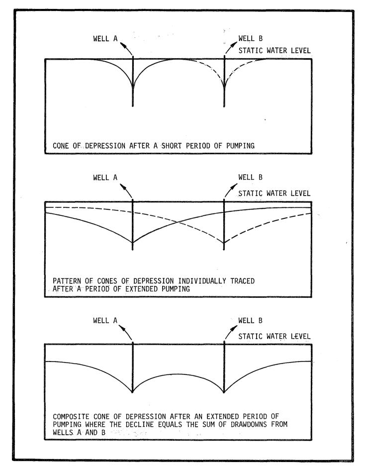
FIGURE 34. -- Development of Composite Cones of Depression by Simultaneous Pumping Wells discharge throughout the growing season. Since the Tri-County area is an established agricultural region, the problems associated with high density and well spacing are inherent.
