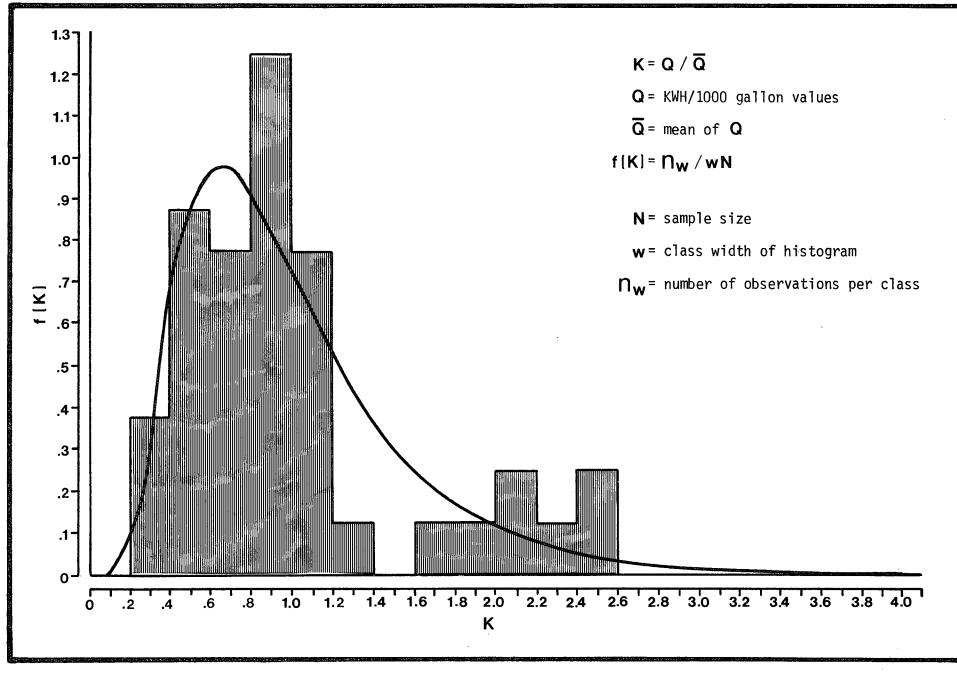
FIGURE 27. -- Log Normal Distribution and Histogram of Pump Data
