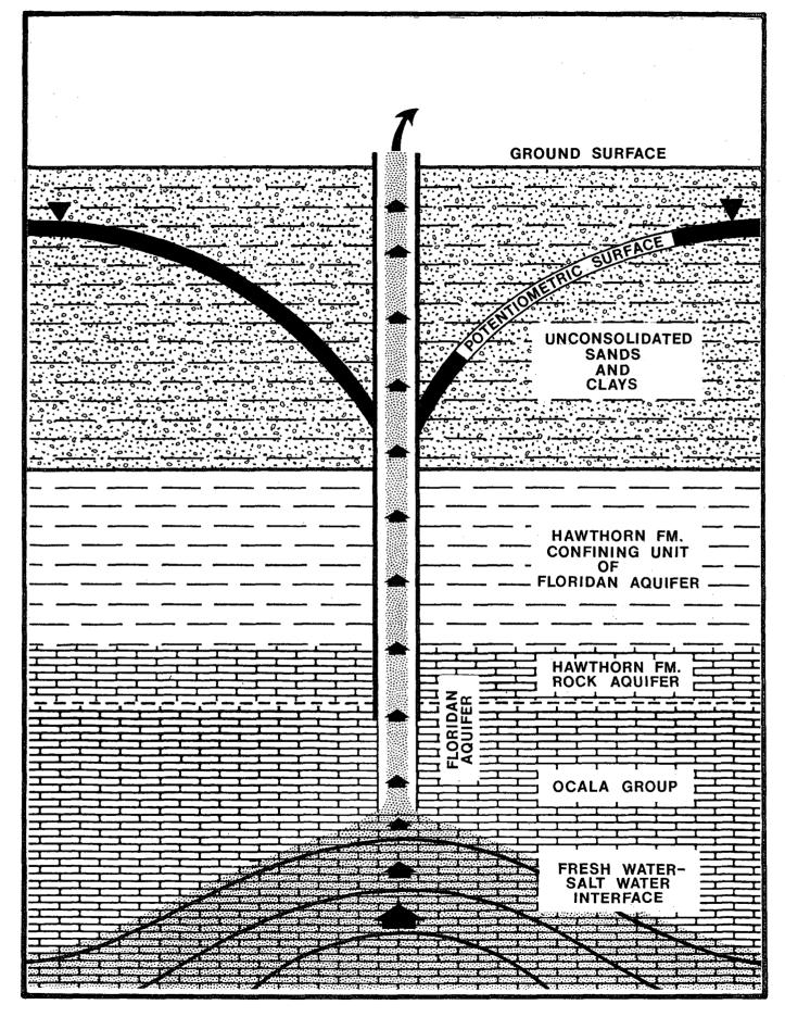
FIGURE 35. -- Schematic Diagram of Salt Water Coning as Related to the Tri-County Area
