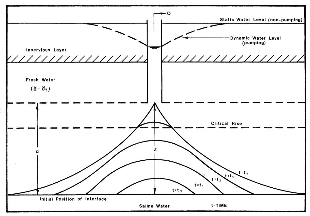
FIGURE 36. -- Upconing of an Abrupt Interface Below a Pumping Well (After Muskat, 1946 and Bear and Dagan, 1964 and 1968)
