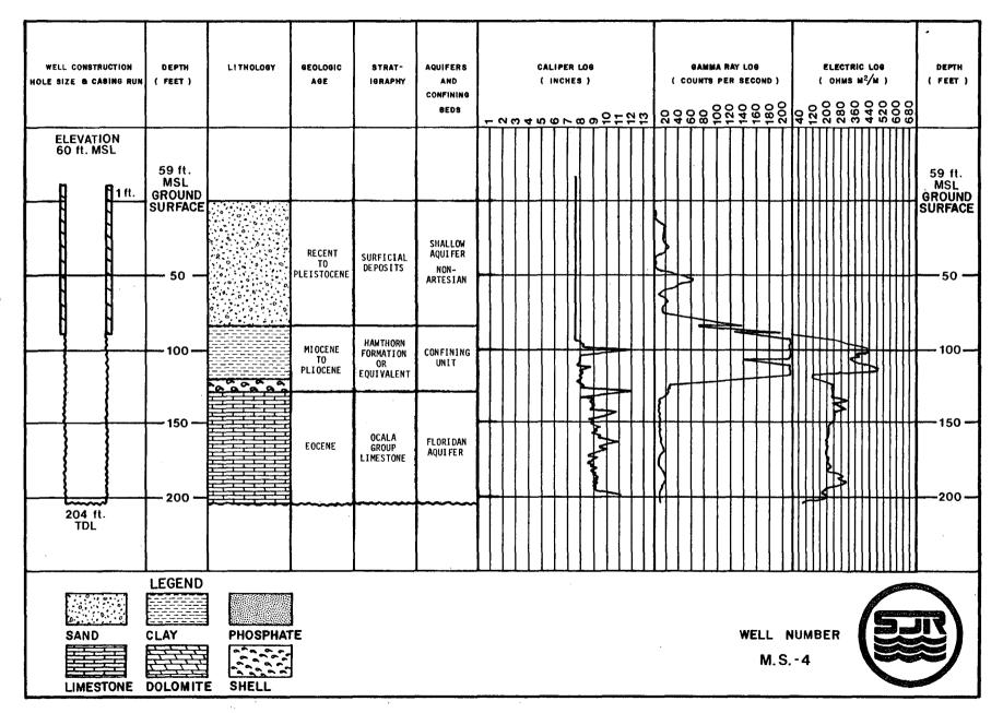
FIGURE A3. -- Hydrogeological and Geophysical Data from Observation Well MS-4
