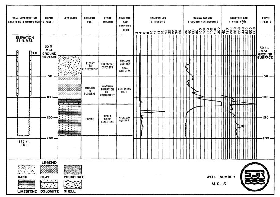
FIGURE A4. -- Hydrogeological and Geophysical Data from Observation Well MS-5
