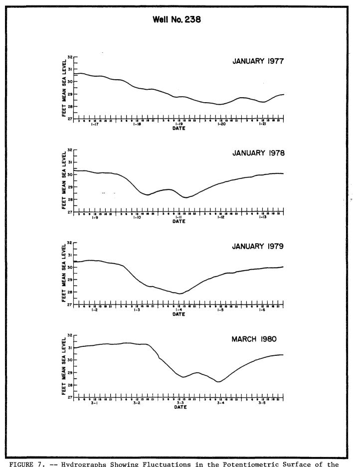
FIGURE 7. -- Hydrographs Showing Fluctuations in the Potentiometric Surface of the Floridan Aquifer at Observation Well 238 Concurrent with the Most Severe Freezes of Winters 1977-80
