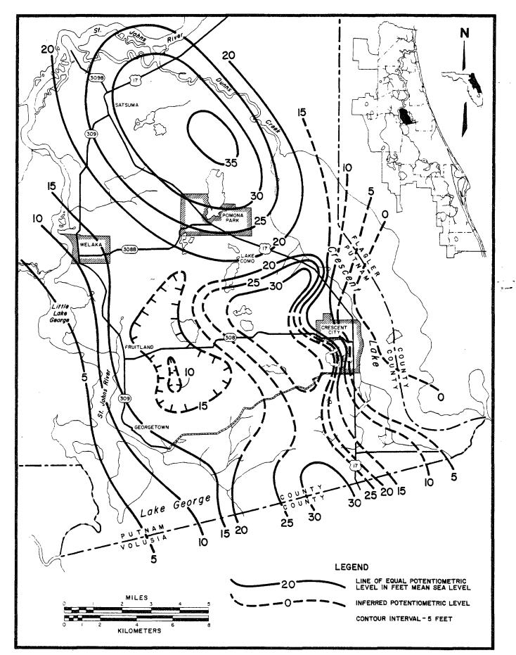
FIGURE 10. -- Map of Crescent City Ridge Depicting Elevation of the Potentiometric Surface of the Floridan Aquifer Prior to Pump Shutdown During the Freeze of March, 1980
