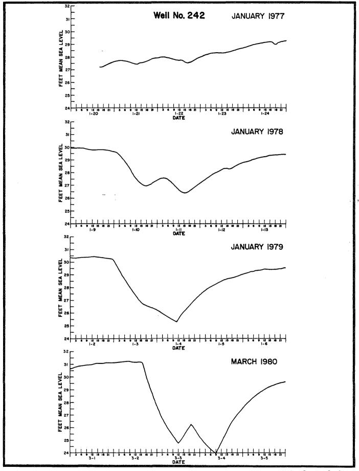
FIGURE 8. -- Hydrographs Showing Fluctuations in the Potentiometric Surface of the Floridan Aquifer at Observation Well 242 Concurrent with the Most Severe Freezes of Winters 1977-80
