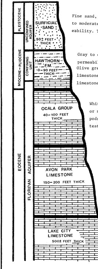
Fine sand, shell, and clayey sand. Yields small to moderate amounts of water depending on permeability. Transmissivity 10,000 to 7,500 gal/day/ft
