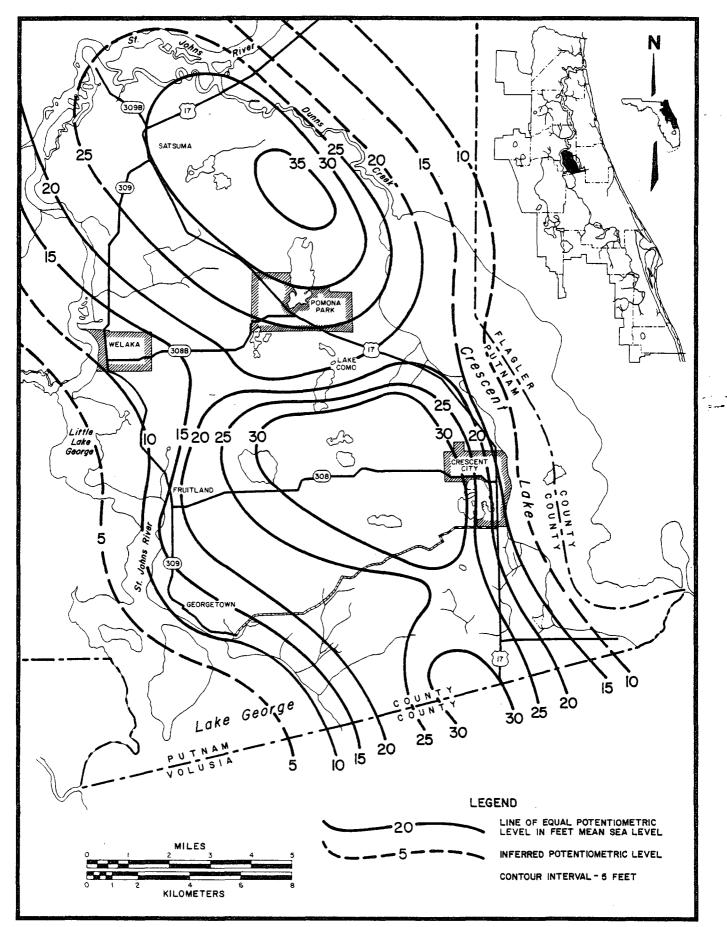
FIGURE 9. -- Map of Crescent City Ridge Showing Elevation of the Potentiometric Surface of the Floridan Aquifer for September, 1978
