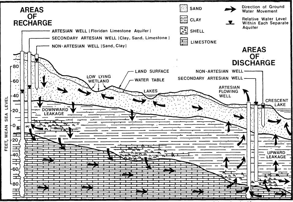
FIGURE 5. -- Diagram Showing Relationship Between Non-Artesian, Secondary Artesian, and Artesian Aquifers on the Crescent City Ridge
