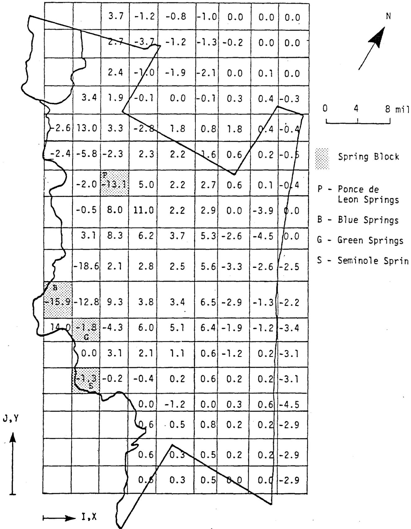
Figure 4.7 Final Recharge Distribution (Inches/Year), for the Three-Layer Model.
