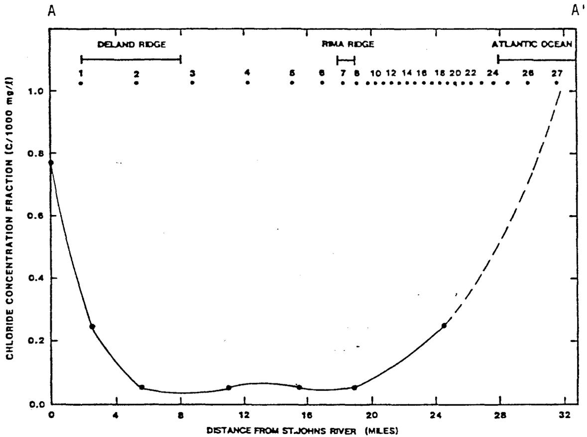
Figure 4.9 Chloride Concentration Fraction in the Upper Floridan Aquifer, 1980, Along Section A-A' (from SJRWMD).
