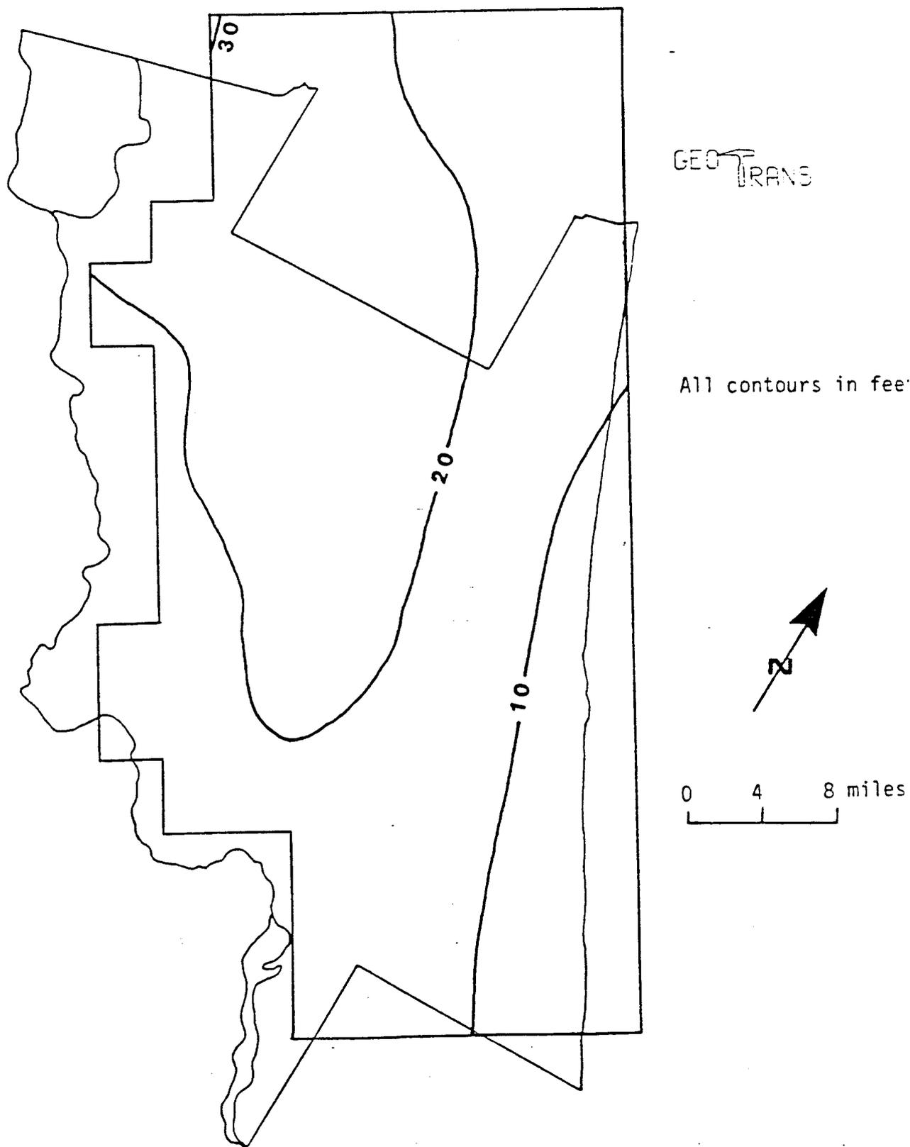
Figure 4.6 Potentiometric Head Distribution in the Lower Floridian Aquifer using a Three-Layer Model.
