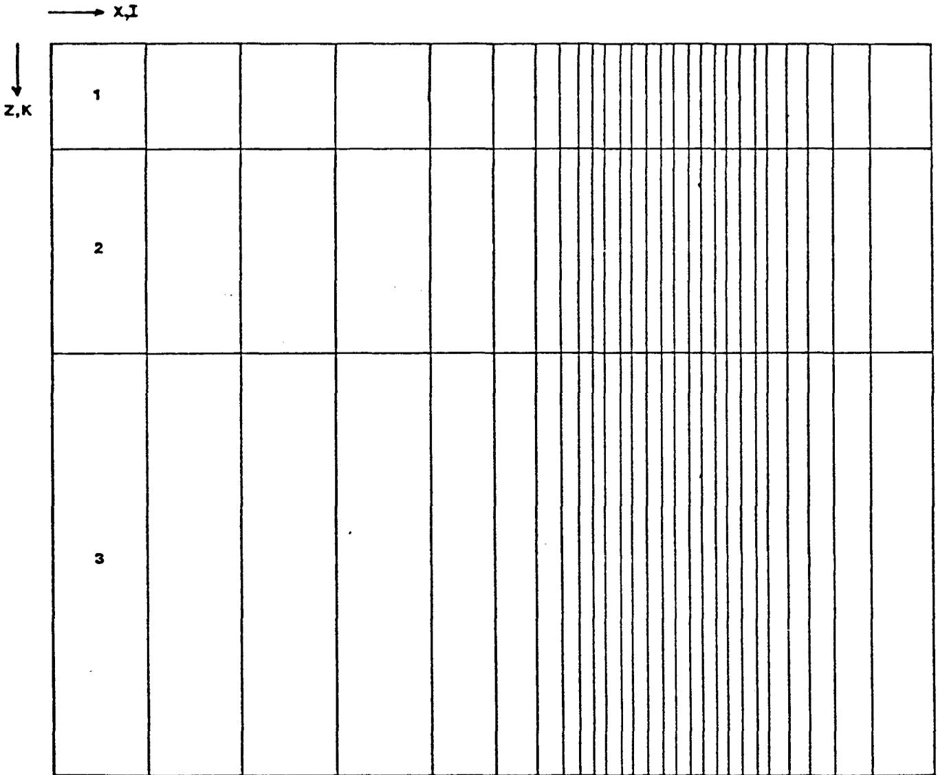
Figure 4.3 Two-Dimensional, Finite-Difference Grid Used for the Three-Layer Flow and Transport Model (vertical exaggeration  $\sim 230:1$ ).
