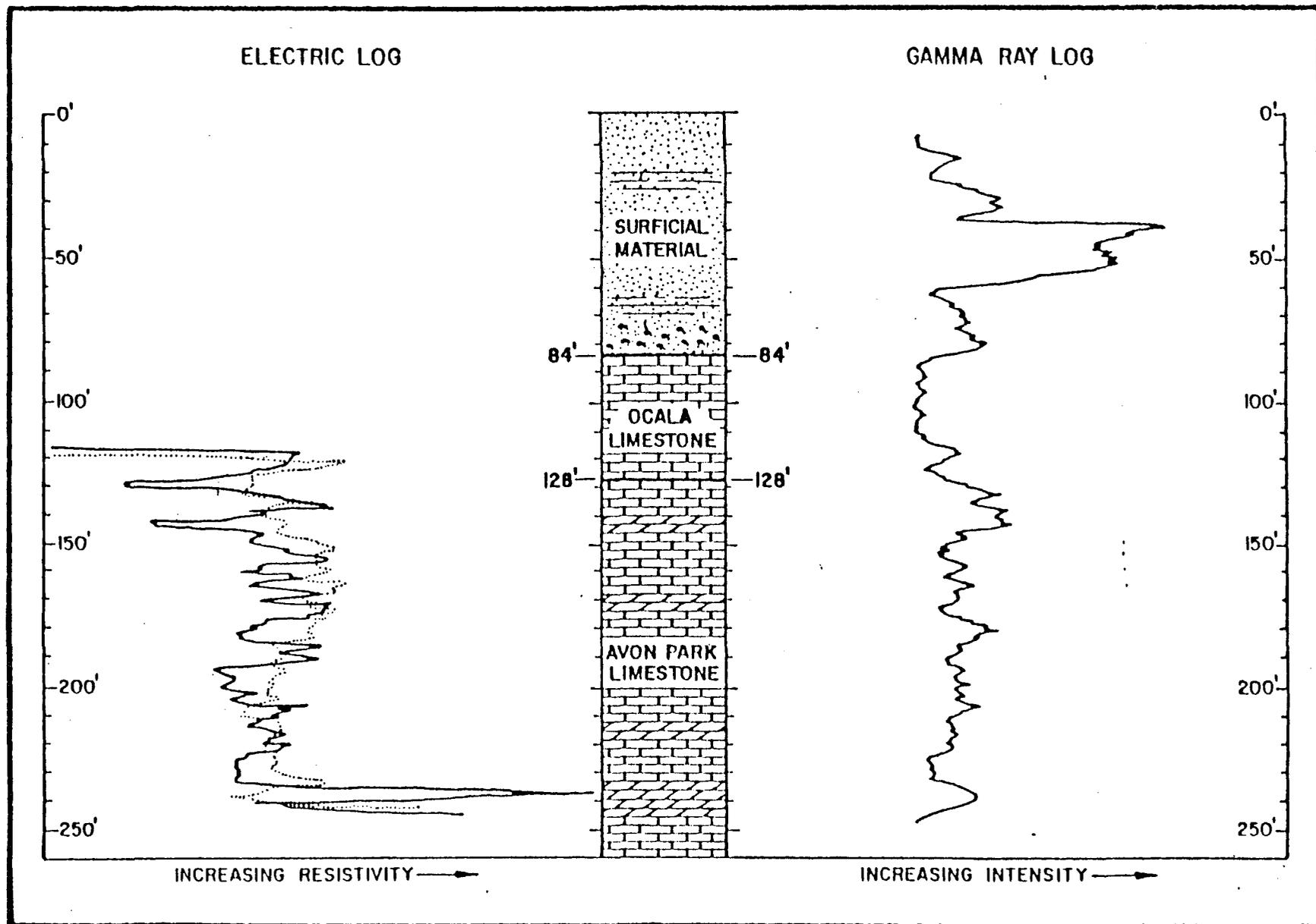
Figure 3.2 Gamma-ray and Electric (Resistivity) Logs of Well V-15 (from Johnson, 1981).
