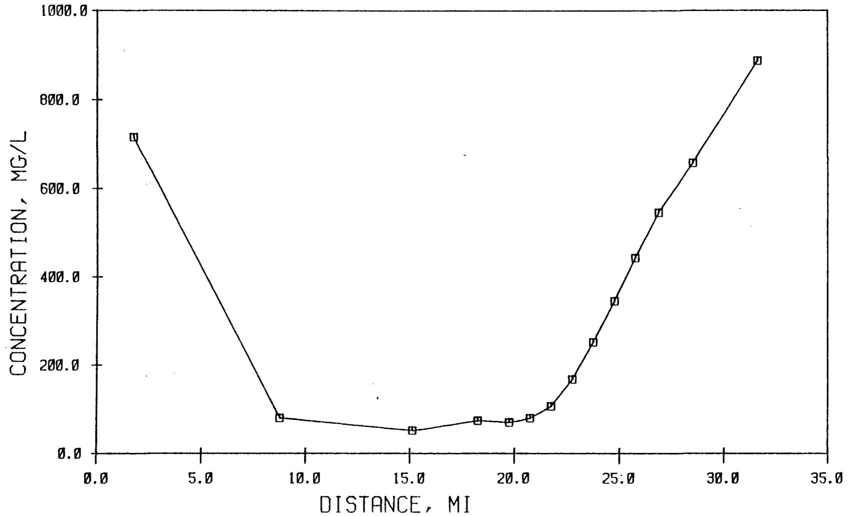
Figure 4.11 Steady-State Chloride Distribution, From Run SS1, Along Cross Section A-A' in Upper Floridan Aquifer.
