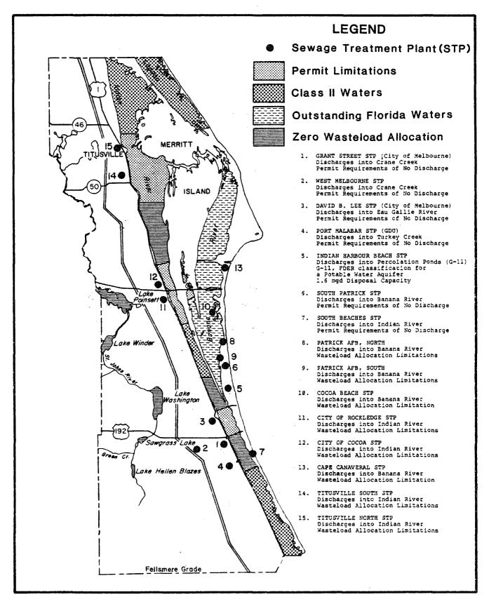
Figure 8. Location of WWTP's in Brevard County and pre-1985 information on disposal methods of the WWTP's.
