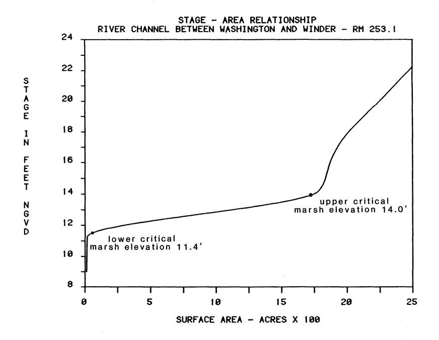
Figure 20. Stage area curve for RM 253.1, 1.3 miles downstream of the Lake Washington weir.
