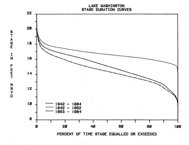
Figure 9. Stage duration curves for the St. Johns River at Lake Washington.
