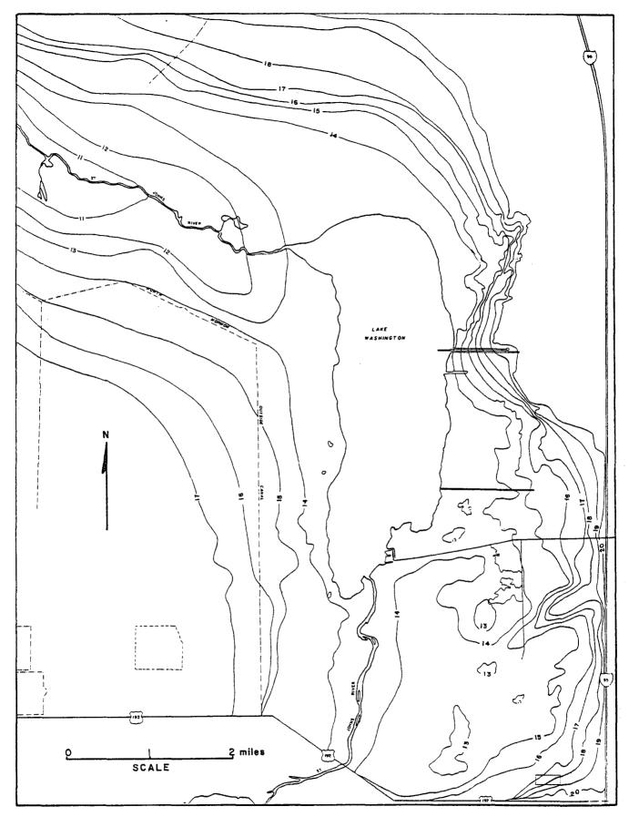
Figure 13. Map of the Greater Lake Washington Basin showing one-foot elevation contours for the time period 1985.
