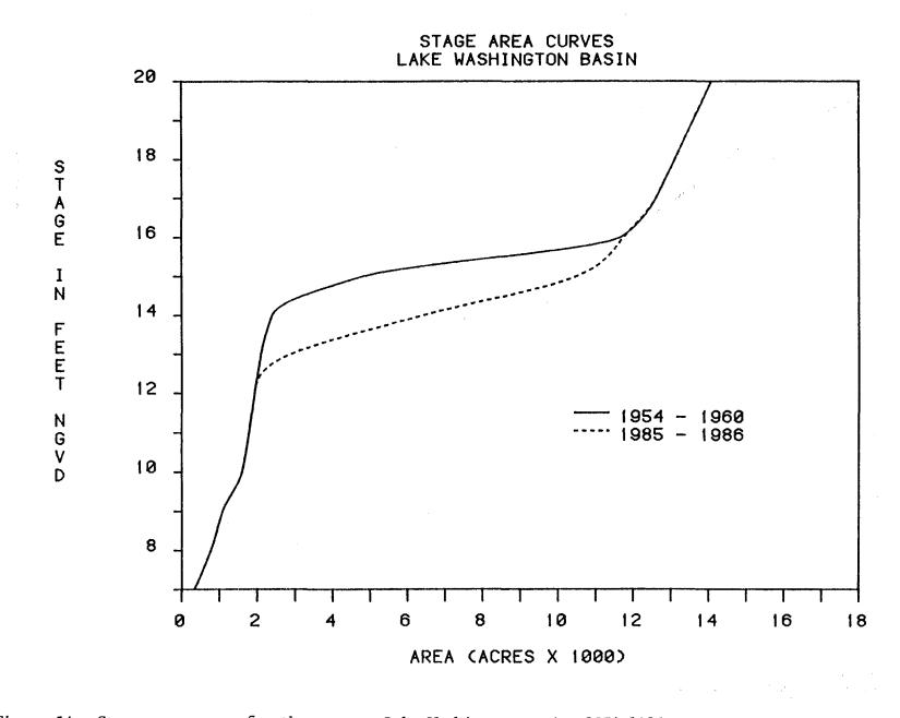
Figure 14. Stage area curve for the Greater Lake Washington Basin, 1954-1986.
