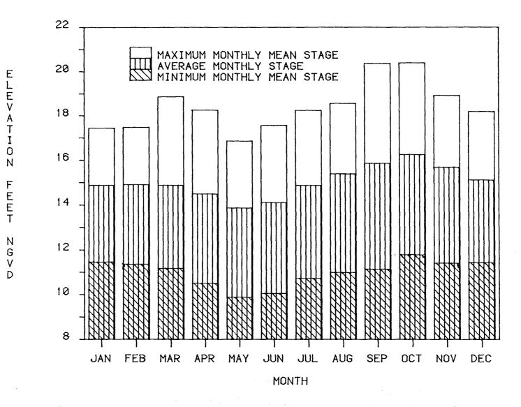
Figure 5. Monthly variation in mean, maximum and minimum lake elevation. Lake Washington, 1942-1984.
