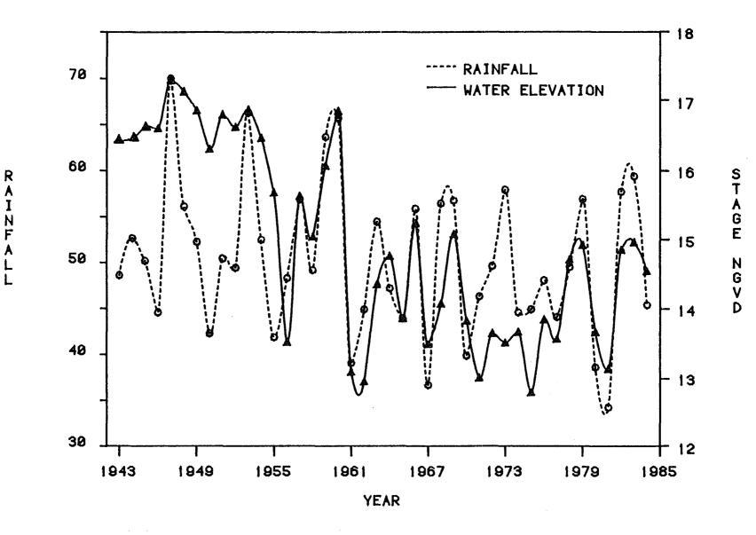
Figure 8. Variation in total annual rainfall and surface water elevation at Lake Washington from 1943-1984.
