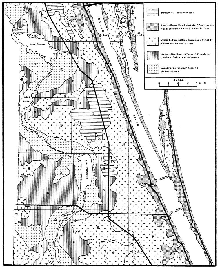
Figure 3. Soils of the Upper St. Johns River Basin (USDA, Soil Conservation Service, 1974).
