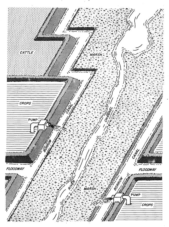
Figure 2. Typical floodplain levee system
