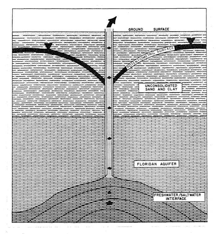
Figure 9. The movement of relict brackish water at the freshwater/saltwater interface caused by pumping
