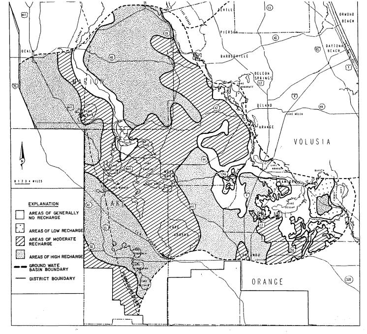
Figure 7. Approximate areas of natural recharge and discharge for the Floridan aquifer in the Middle St. Johns ground water basin, modified from Stewart (1980)
