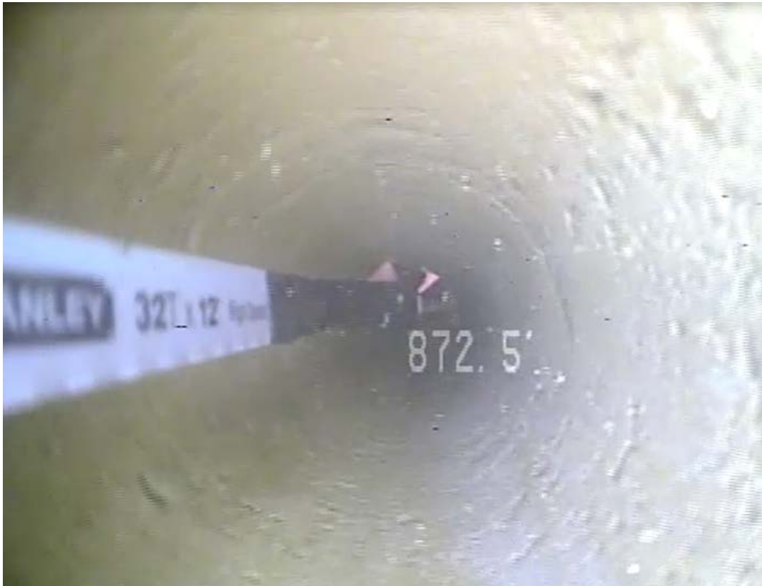
Figure 9. Borehole video view of in-gage section at 872 feet bls with no fractures and minor dissolution features.
