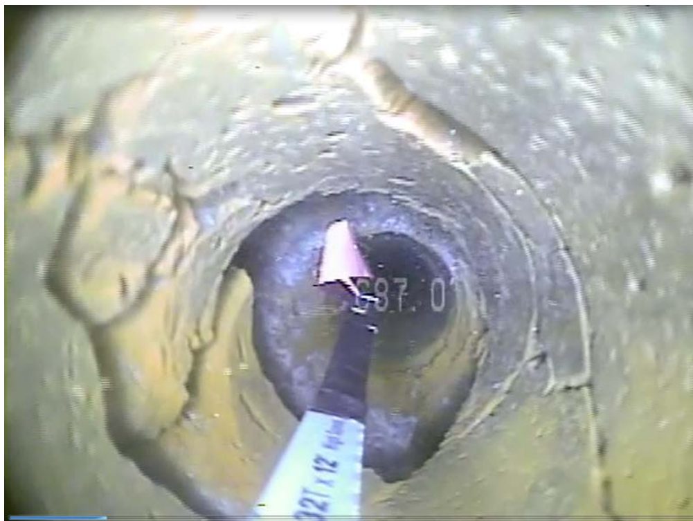
Figure 7. Borehole video example showing fractures and a bedding plane breakout feature at 687 feet bls.
