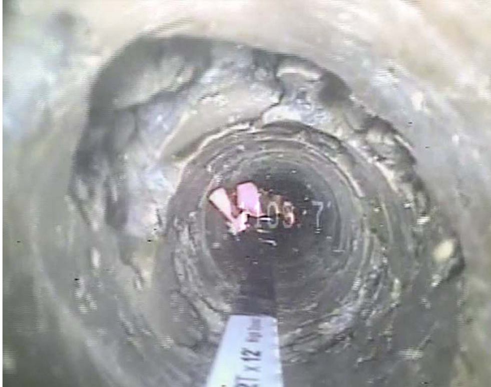
Figure 11. Breakout zone at 1,103 feet bls with pieces of very hard dolostone that have broken off the borehole wall during the drilling process.
