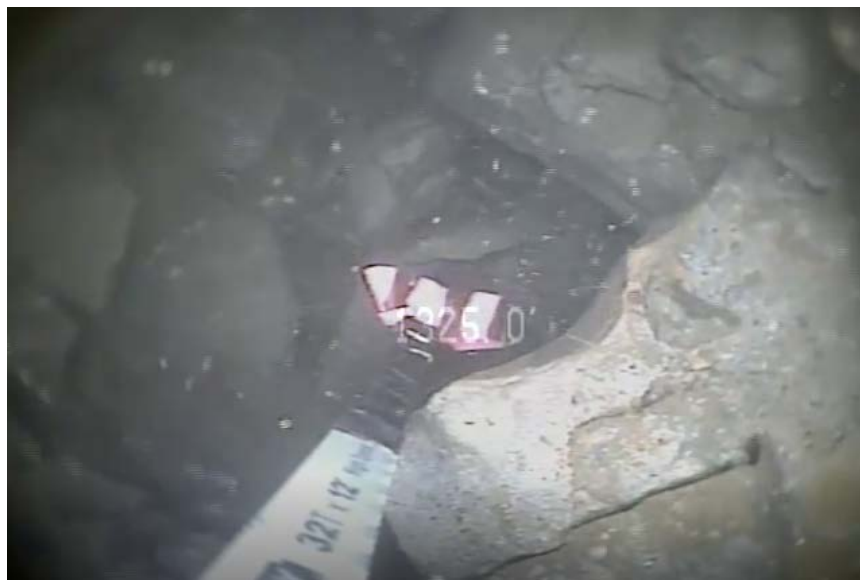
Figure 12. Borehole video showing rocks obstructing the borehole at 1,325 feet. White particles are moving rapidly down through the rocks indicating strong downward flow.
