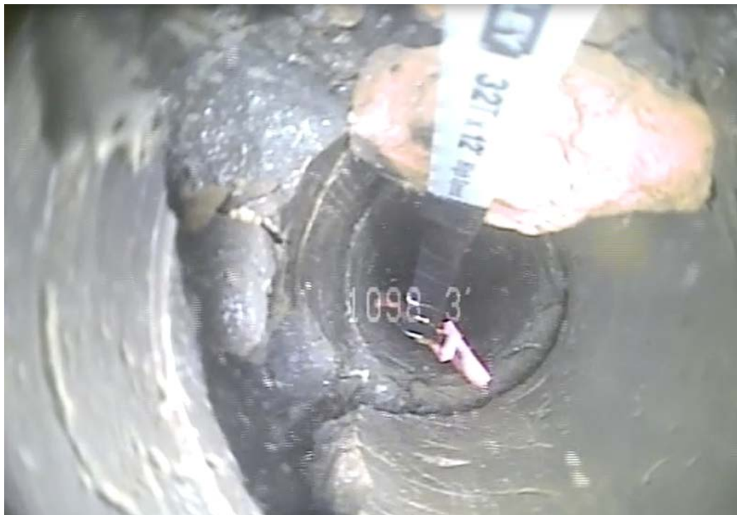
Figure 10. Fracture zone at 1,098 feet bls with rock balancing on camera.
