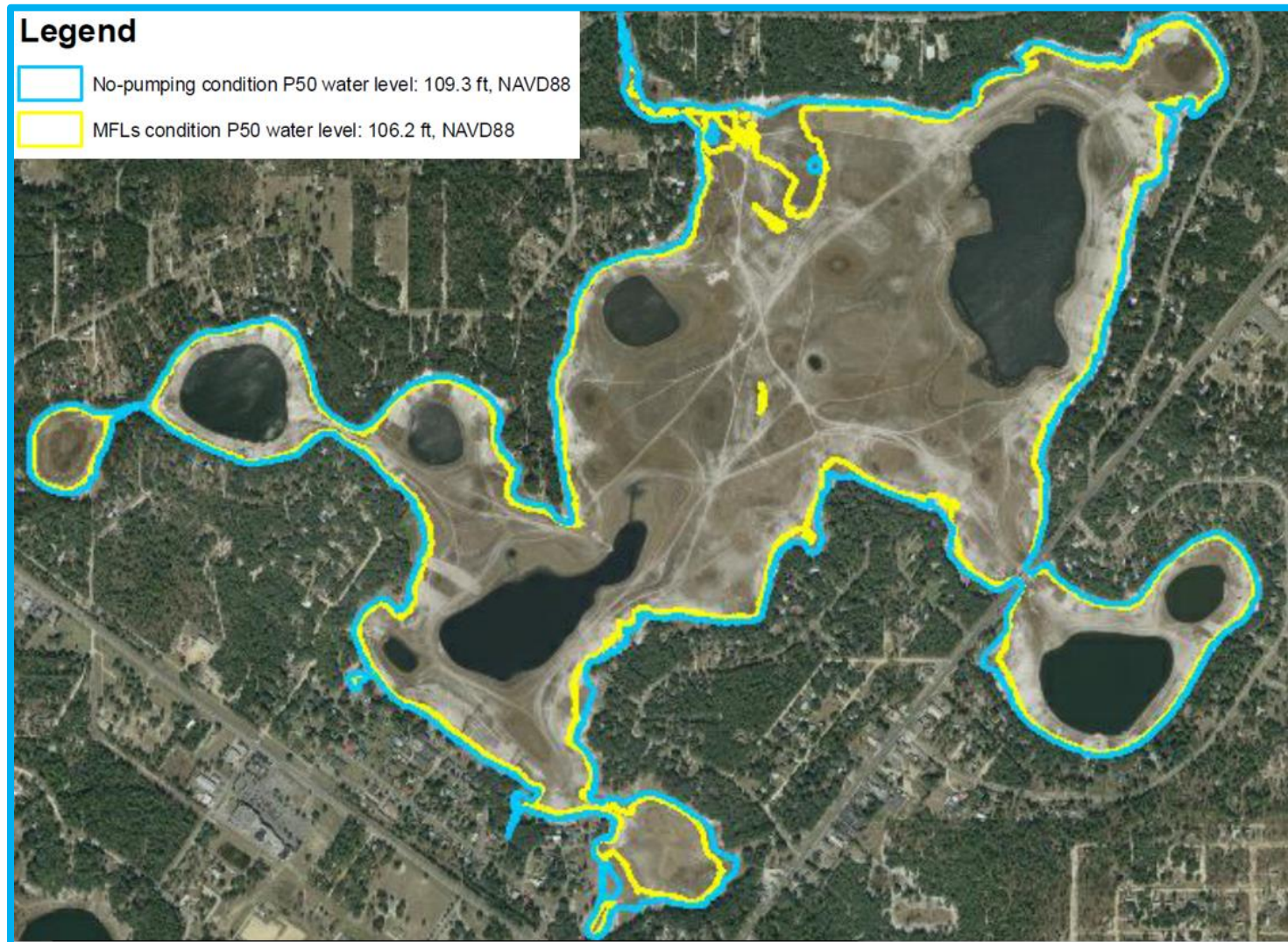
Figure 24. Difference between the no-pumping and MFLs condition for Lake Brooklyn at the P50 lake level.
