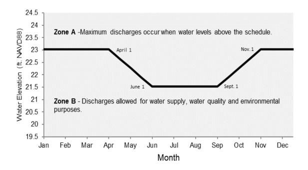
Figure 1. Flood control regulation schedule for Blue Cypress Marsh Conservation Area showing Zones A and B. When water levels are in Zone A, discharges are regulated by the MWCM. When water levels are in Zone B, discharges are regulated by the EWMP. Dates show when regulation schedule changes between the dry and wet seasons.
