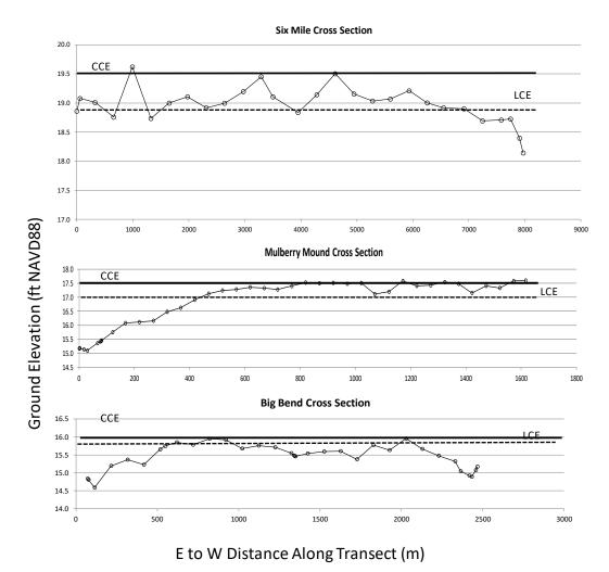
Figure 10. Cross sectional survey data in 2013 for three SJMCA transects showing central critical elevations (CCE; solid line) and lower critical elevations (LCE; dashed line).
