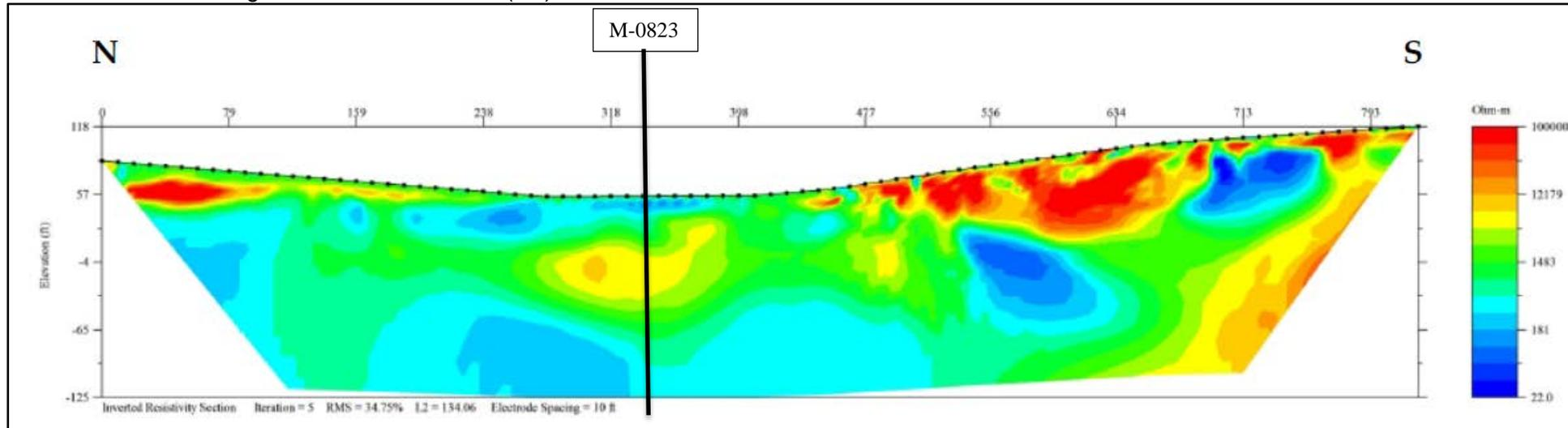
Figure 10. Site 1 Line 2 Electrical Resistivity profile (modified from Jones Edmunds/ Geohazards) report included in Appendix A)
