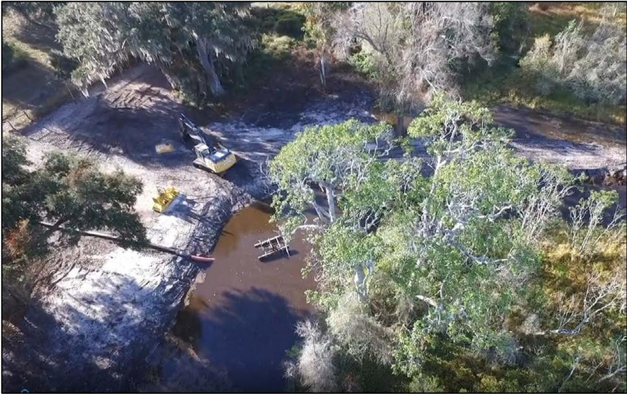
Figure 7. UAV view of surface water pump and intake location in rim canal sump excavated by District staff.
