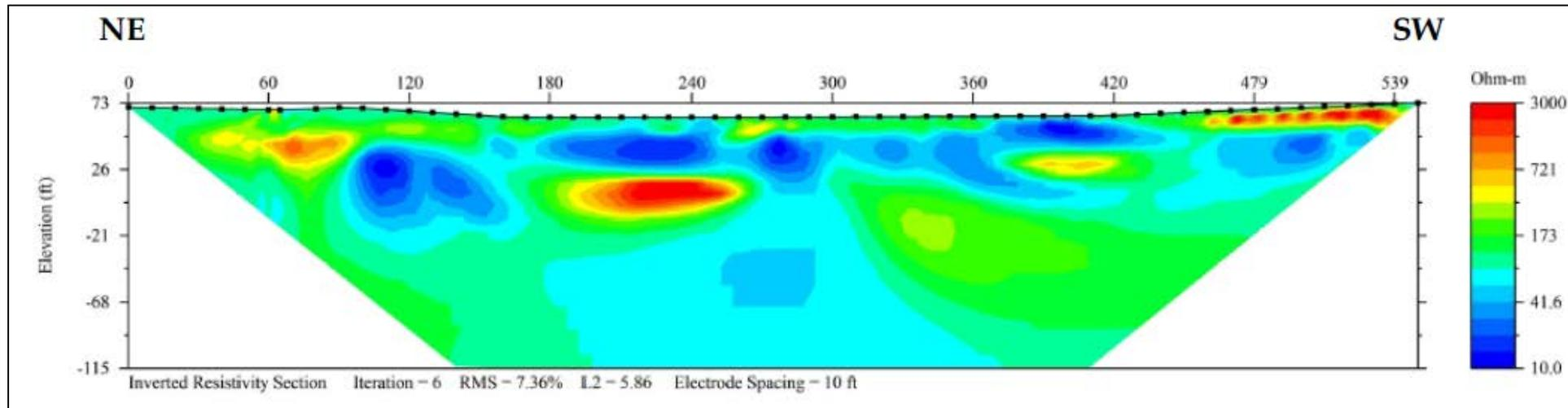
Figure 11. Site 2 Electrical Resistivity Profile 3 (adapted from Jones Edmunds/Geohazards report Appendix A)
