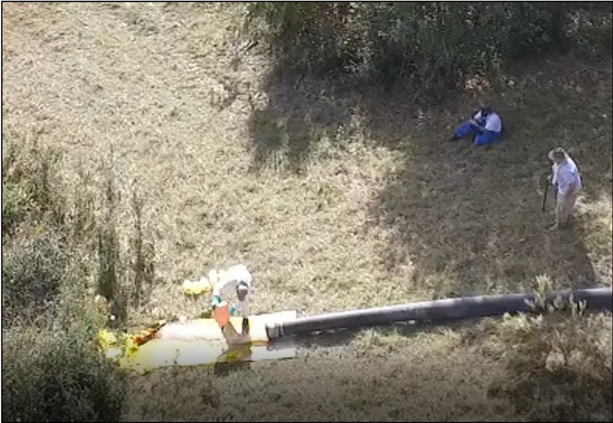
Figure 8. UAV view of surface water discharge pipe with dye being introduced into the flowing water by Karst Environmental Services staff.
